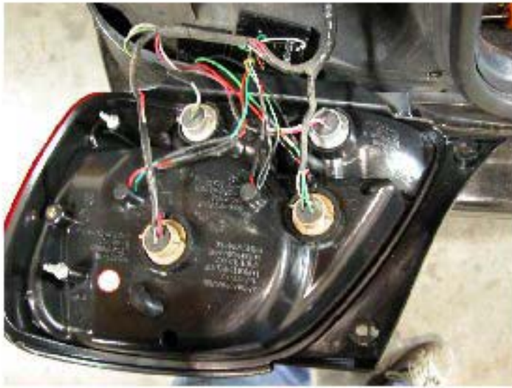
11. Replace the sockets back into the L.E.D. Tail light please see the "L.E.D. TAIL LIGHTS installation instructions" if your Tail lights don't have L.E.D. You can skip the installation instructions.
