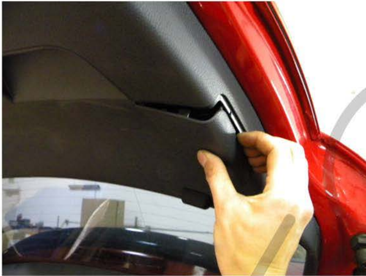
1. Remove the cover from inside of the trunk
