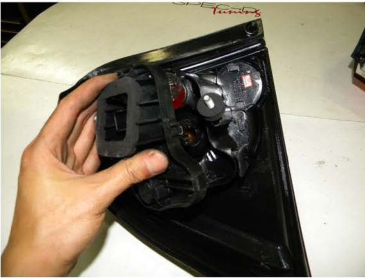
11. Install taillight socket to the new taillight
