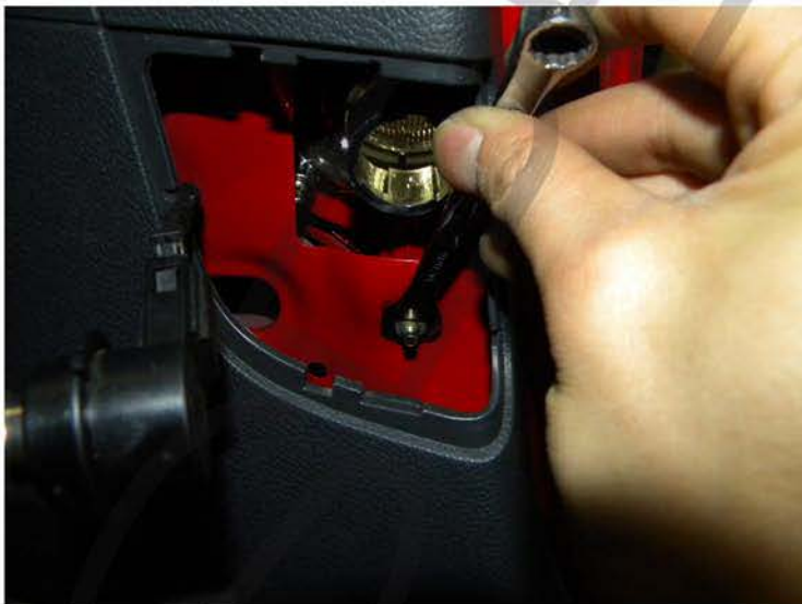
3. Remove two 10mm bolts then remove the trunk taillight
