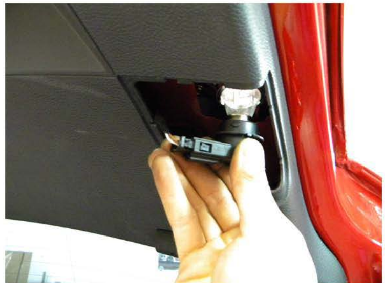
4. Install new trunk taillight two 10mm bolts and install back up light socket
