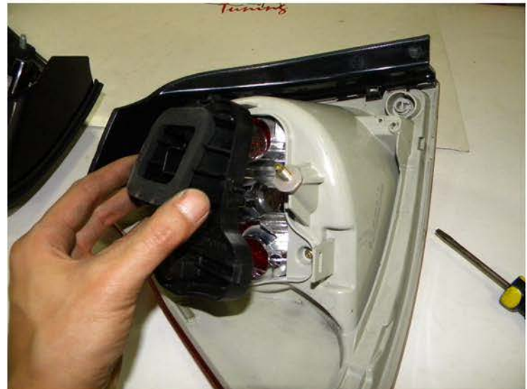
10. Remove the taillight socket from the OEM taillight
