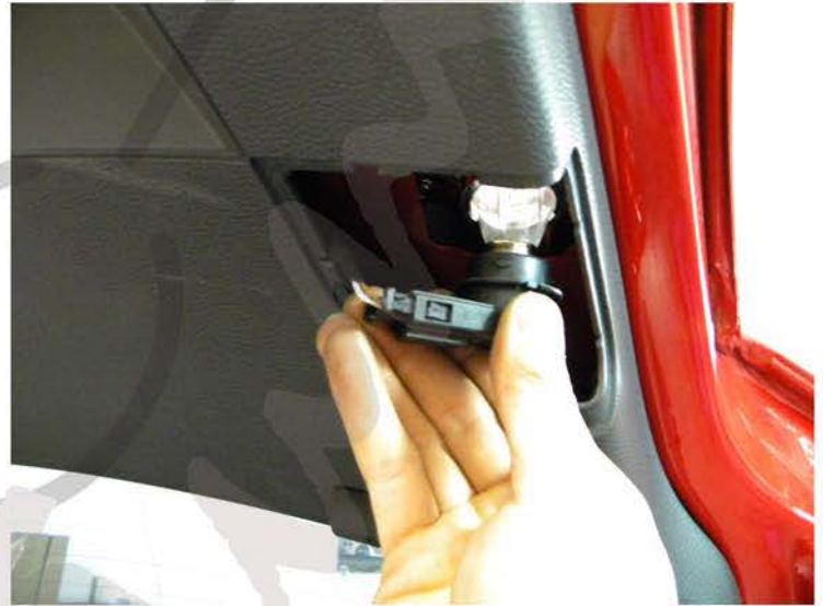
2. Remove back up light light bulb socket
