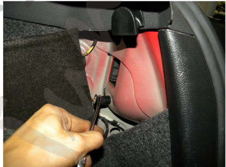
8. Remove two 13mm taillight bolts
