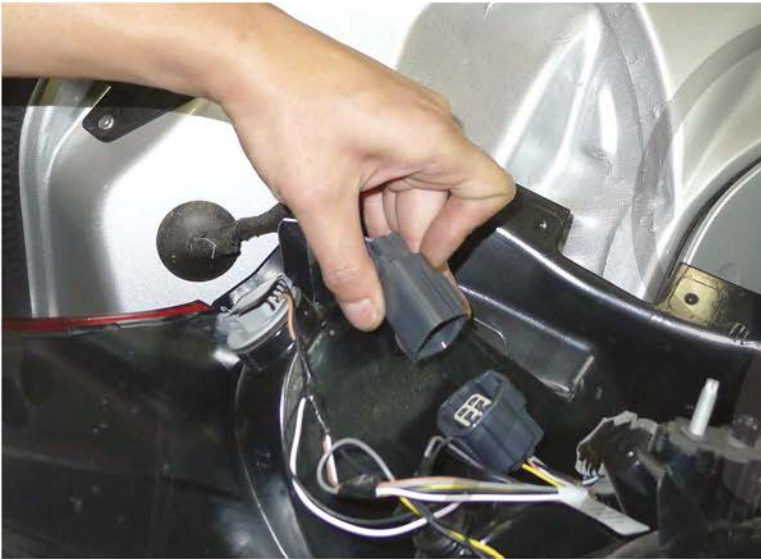
7. Disconnect the taillight harness
