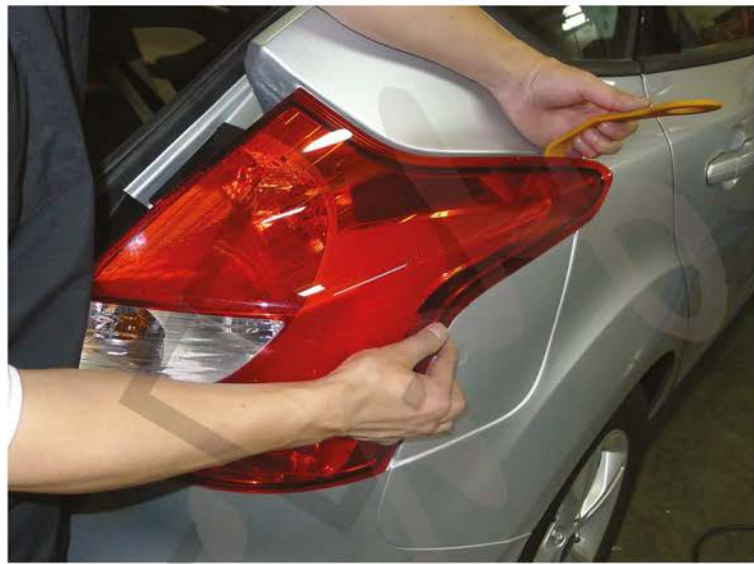
6. Remove the factory taillight
