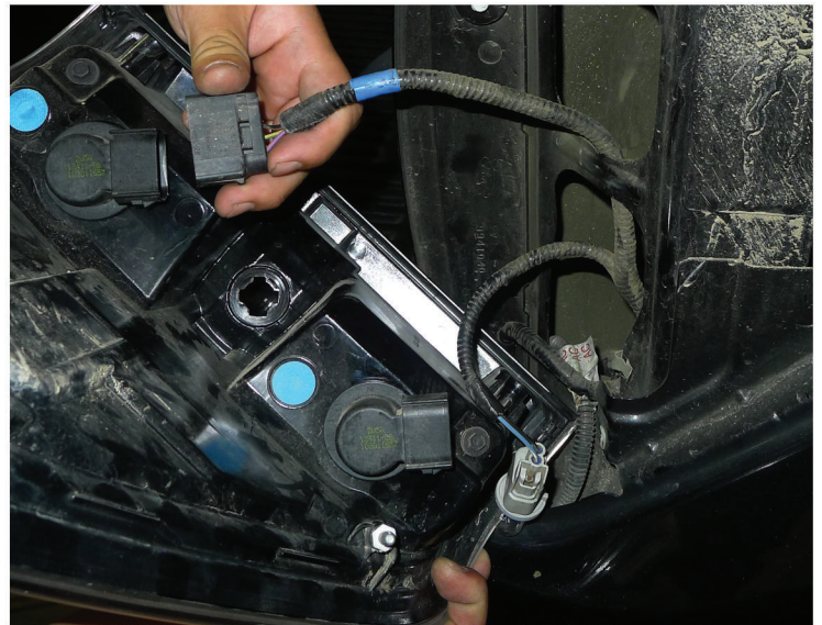
4. Disconnect the wire harness
