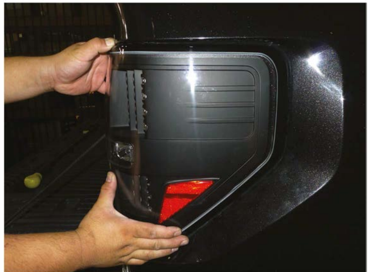
10. Place the LED tail light in the stock location
