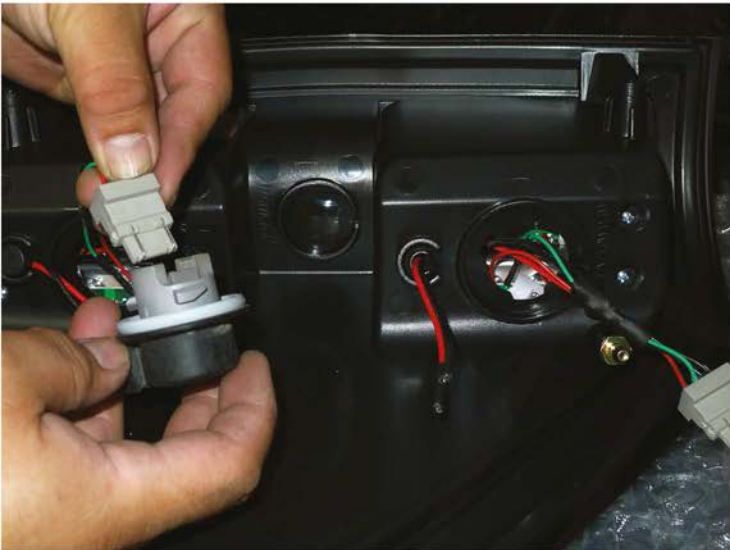
7. Connect the brake and signal light socket to the LED tail light
