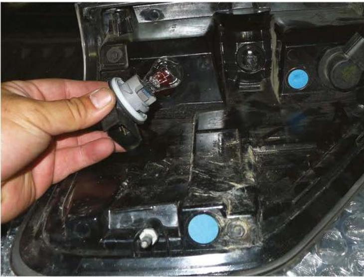
5. Remove the brake and signal light socket
