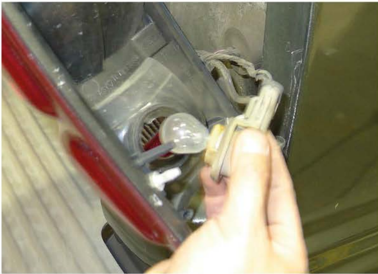
5. Remove the taillight sockets
