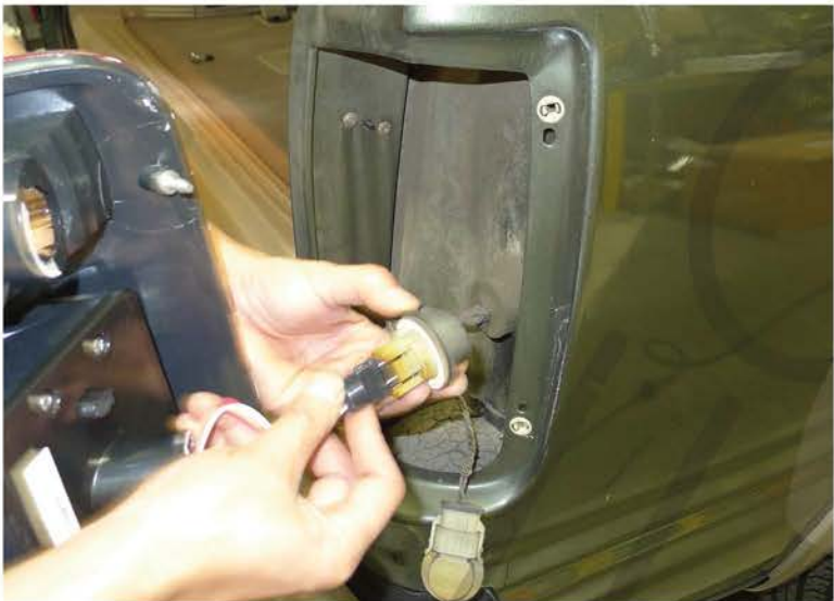
7. Connect the LED taillight harness to the taillight socket
