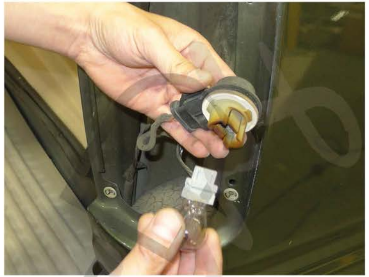
6. Remove the taillight bulb
