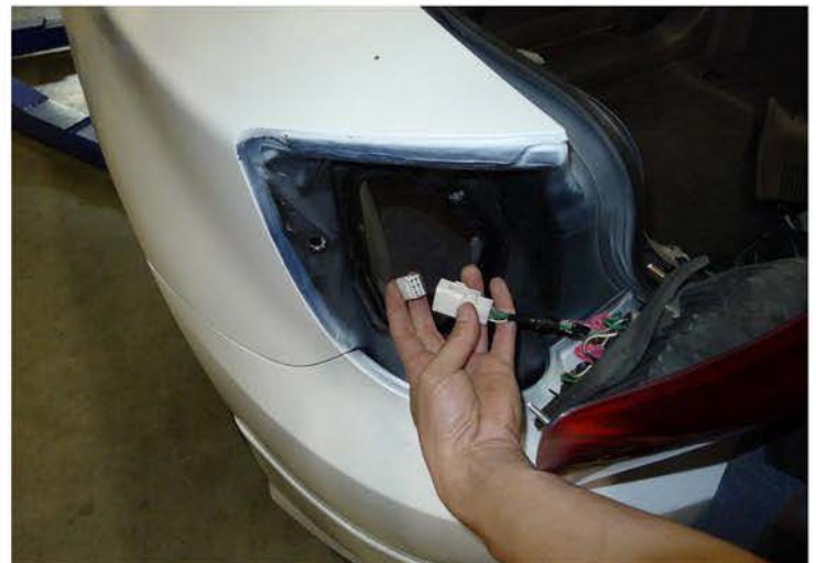
10. Disconnect the tail light harness
