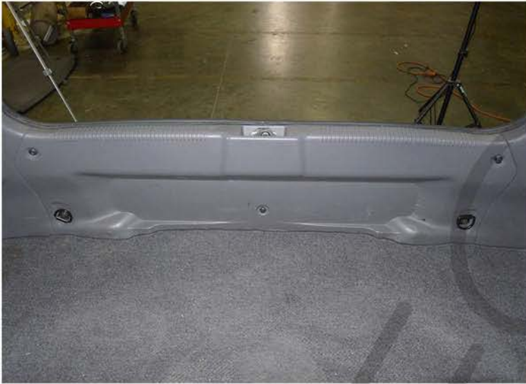
1. (3) Plastic clips and the (2) 10mm bolts location
