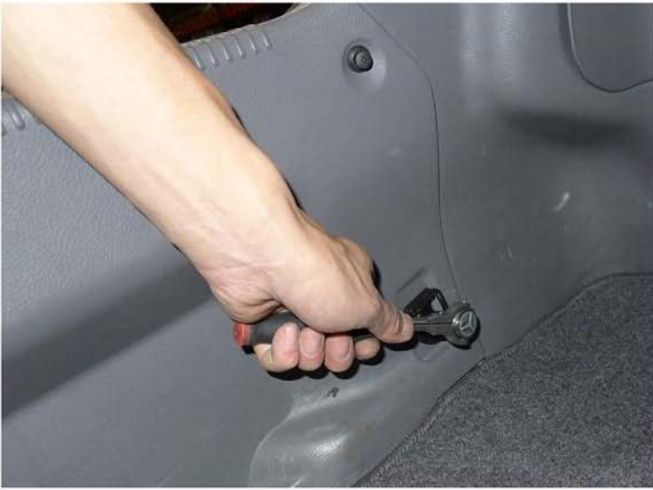
17. Tighten the (2) 10mm bolts and replace the (3) plastic clips
