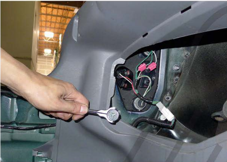
13. Tighten the (3) 10mm nuts
