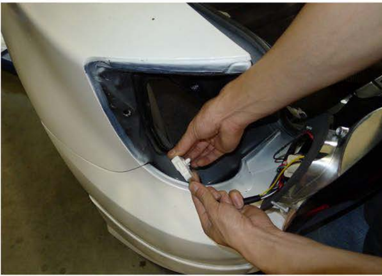
11. Connect the tail light harness to the LED tail light Please see the "L.E.D. tail lights installation instructions" If your tail lights don't have L.E.D. you can skip the installation instructions.
