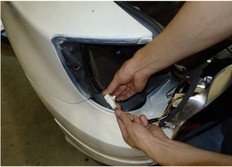
11. Connect the tail light harness to the LED tail light Please see the "L.E.D. tail lights installation instructions" If your tail lights don't have L.E.D. you can skip the installation instructions.
