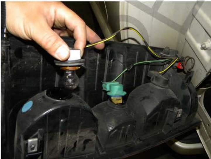
3. Remove the tail light sockets from the tail light
