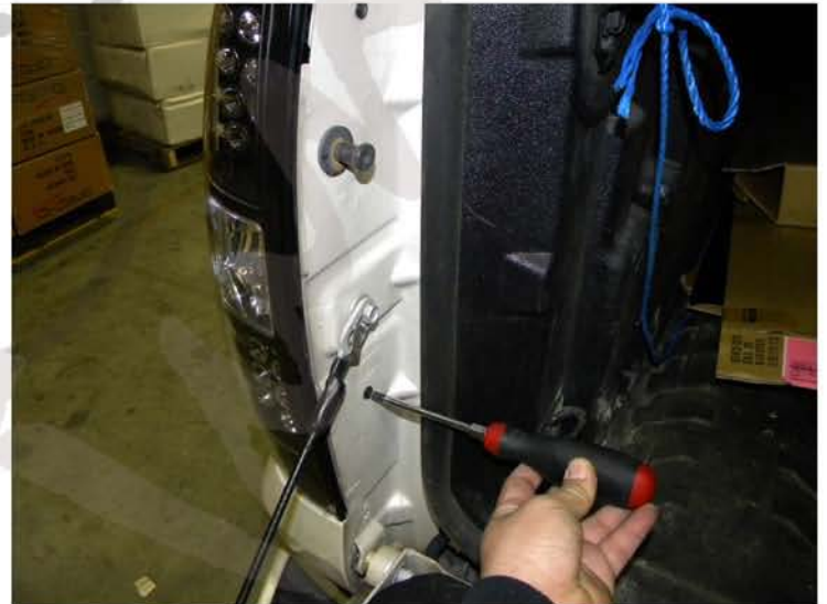
8. Tighten the (2) phillips head screws
