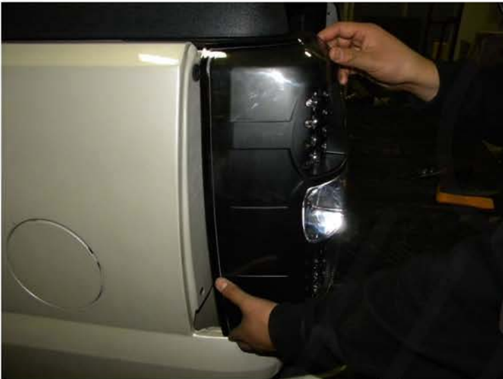
7. Place the LED tail light into stock location
