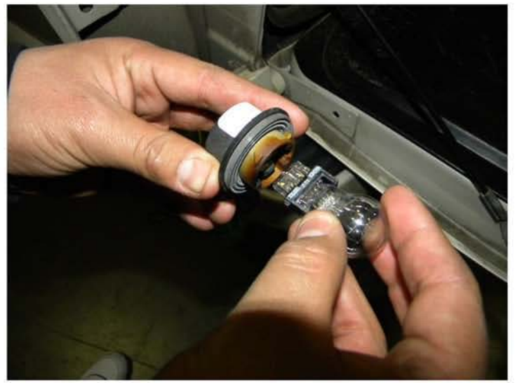
4. Remove the brake lightbulbs
