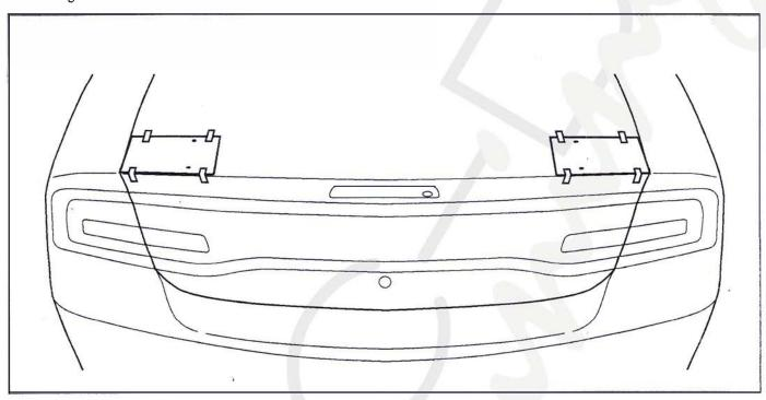
5. **IMPORTANT:** Before marking and drilling the mounting holes, verify the measurements as they are marked on the template with a ruler. Also make a visual check by positioning the spoiler on the trunk lid and double-check the hole positions with the sheet metal openings inside the trunk lid.
