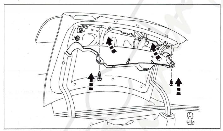
9. Reinstall trim covers at left and right corners. Use (2) 8mm bolts to reinstall grab handle. Close trunk.
