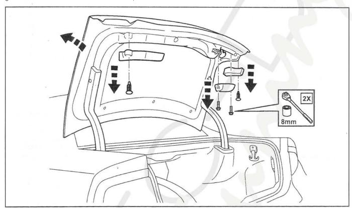
3. Remove fasteners and clips from upper half of trunk liner and carefully pull liner down to access trunk sheet metal. Notice openings in left and right corners where spoiler drill holes will pass through. Retain all parts for reinstallation.
