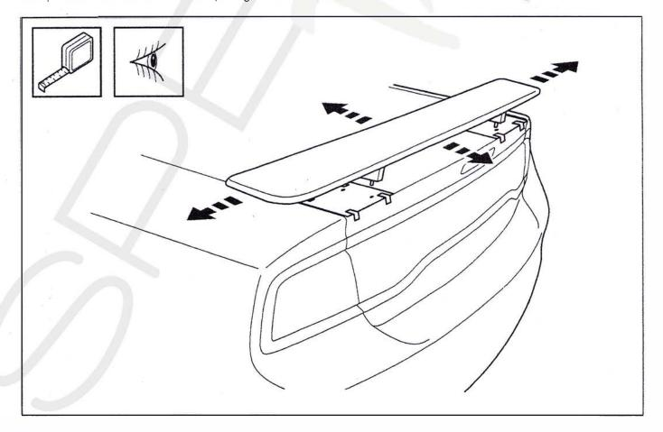
6. Mark each hole position with a punch. Remove the templates. Drill a 5/16" hole at each marked position. Use a deburring tool to clean each hole. Treat all holes with sealant before mounting spoiler.
