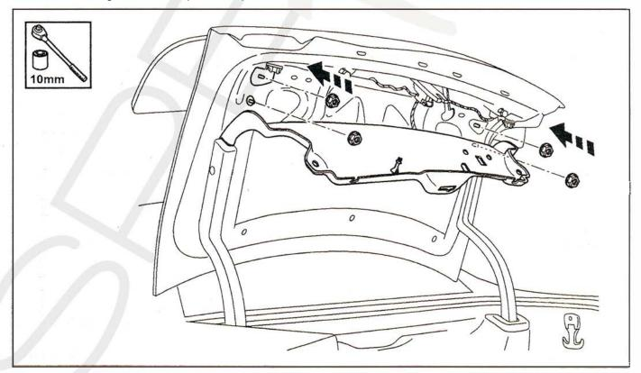
8. Carefully reinstall liner and replace fasteners and clips.
