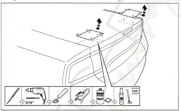
7. Place spoiler into mounting holes and hold in position. Open trunk lid and attach (4) 10mm mounting nuts to spoiler from the inside. Tighten to 6 Nm (4.5 ft. lbs.)
