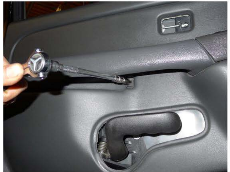
10. Remove the 7mm screw
