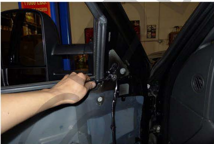
21. Tighten the (3) 10mm nuts
