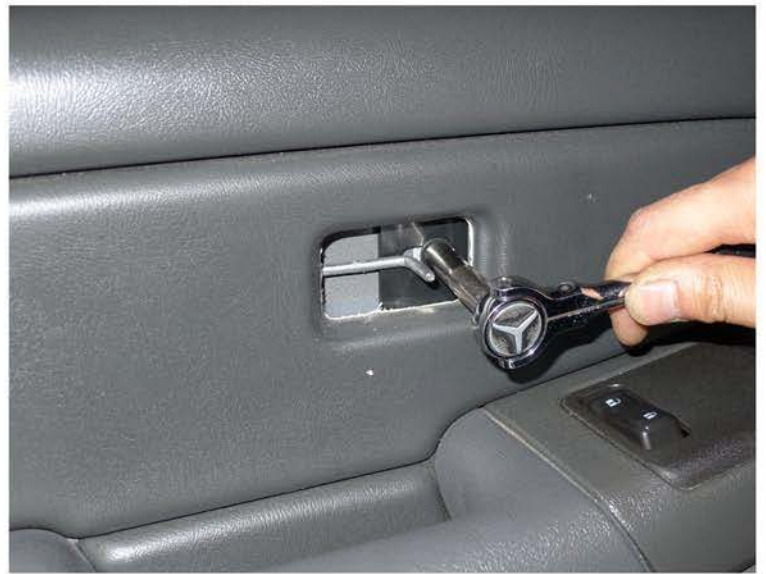
4. Remove the 7mm screw
