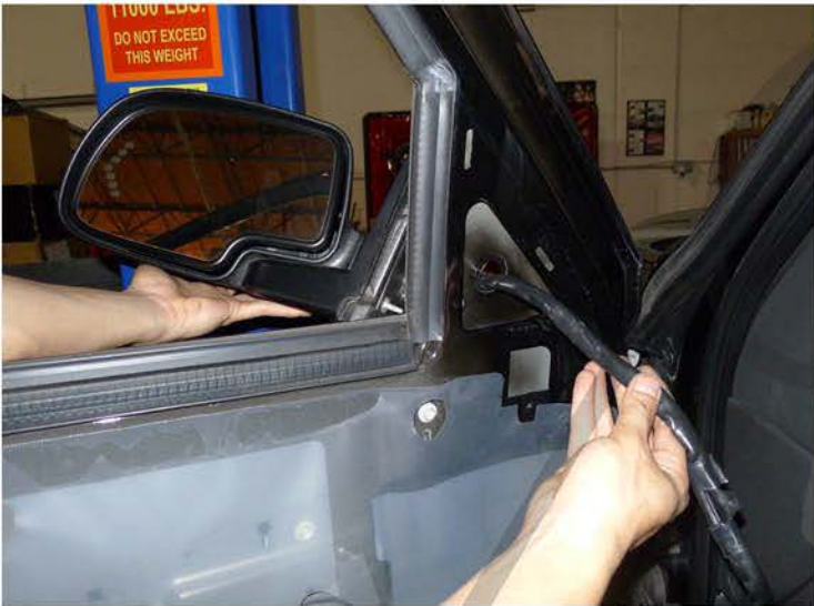
19. Remove the stock mirror
