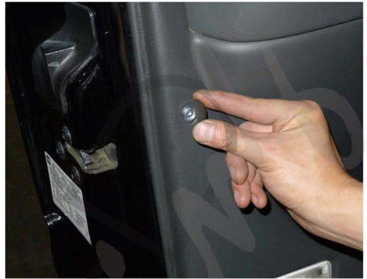
6. Remove the plastic cover
