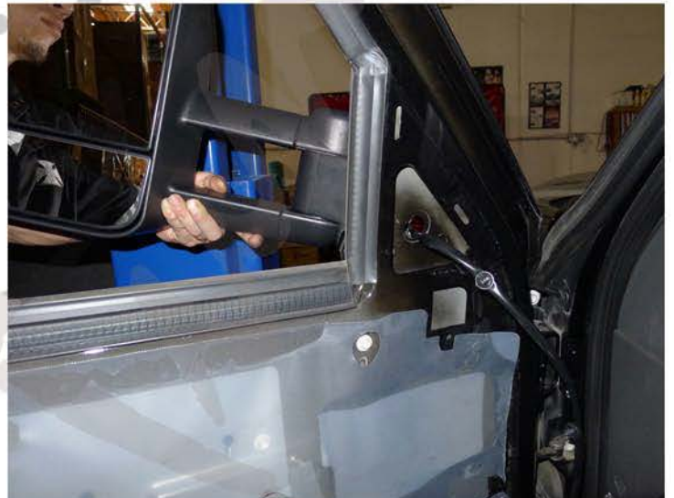
20. Place the new mirror in the stock location
