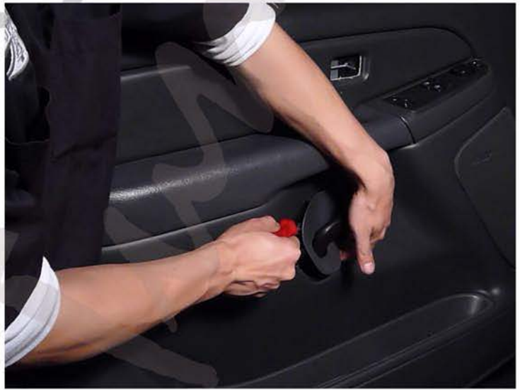
8. Remove the inside handle bezel
