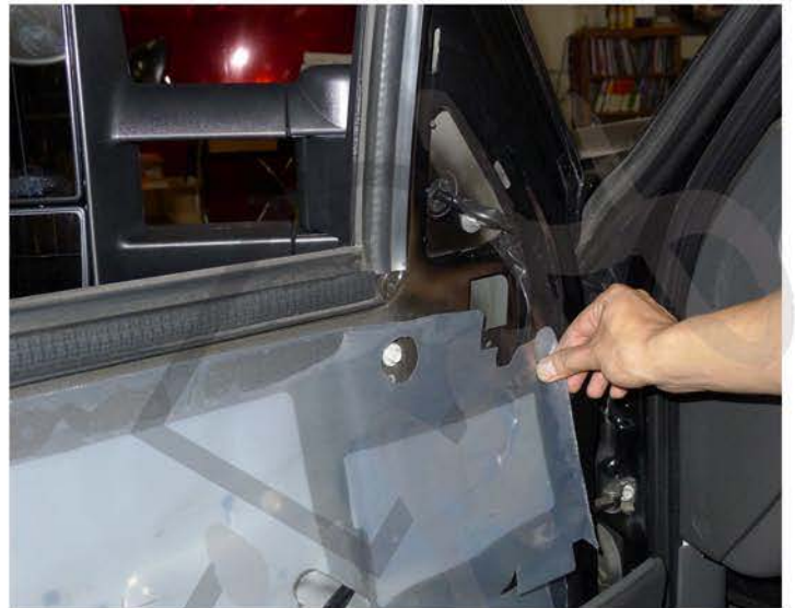
24. Replace the plastic sheet
