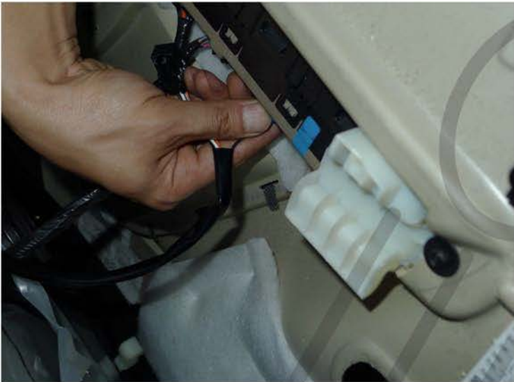
25. Connect the mirror harness to the switch panel
