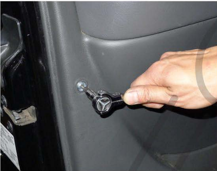
7. Remove the T20 bolt
