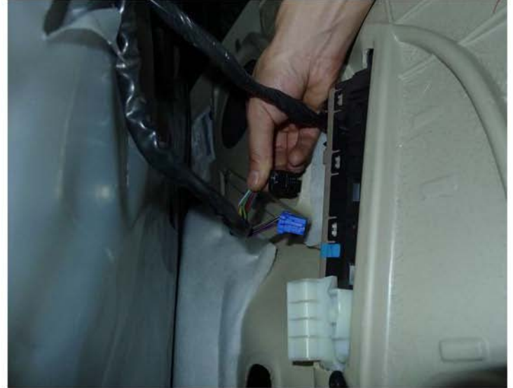
14. Disconnect the mirror harness
