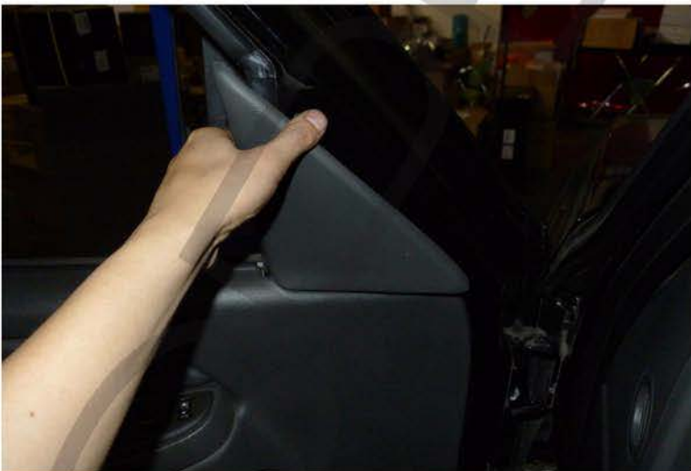
34. Replace the door trim Please repeat the steps in order from 1 to 34 for the opposite side
