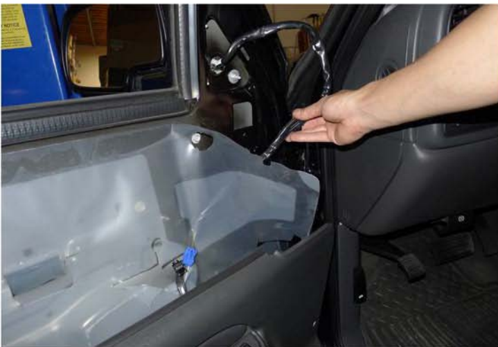
15. Remove the mirror harness from under the plastic sheet
