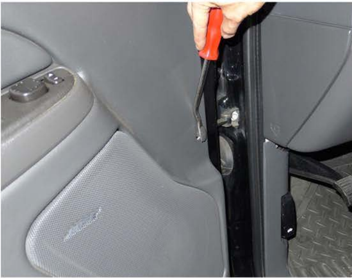
5. Remove the plastic clip
