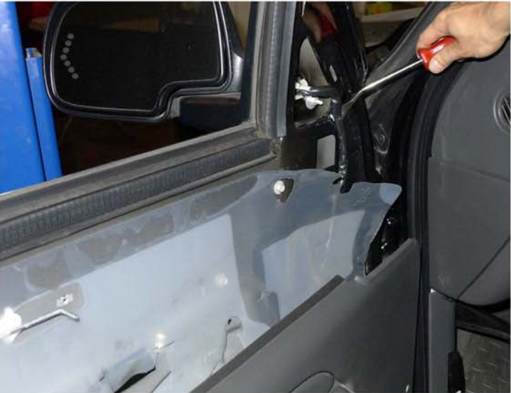
13. Unclip the mirror harness
