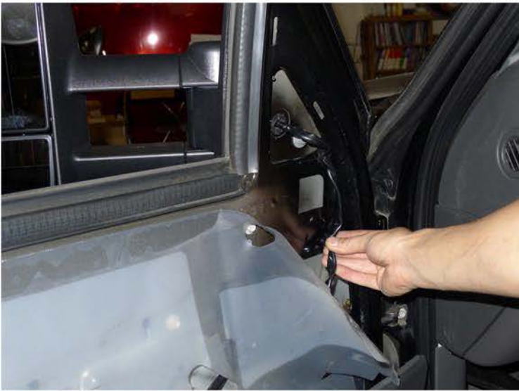
23. Attach the harness clips to the door
