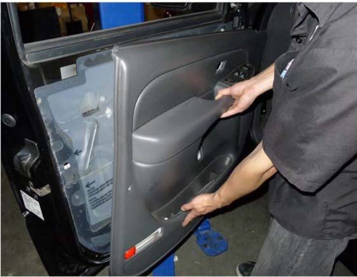
11. Lift the door panel up and away from the door
