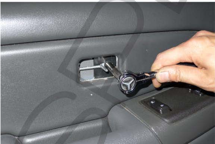
27. Tighten the 7mm screw
