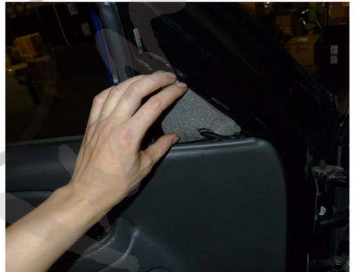
33. Replace the foam insulation
