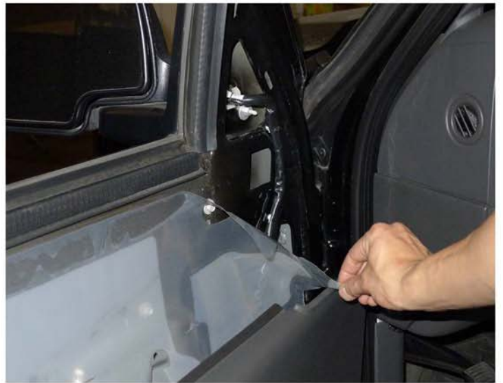
12. Peel away the plastic sheet
