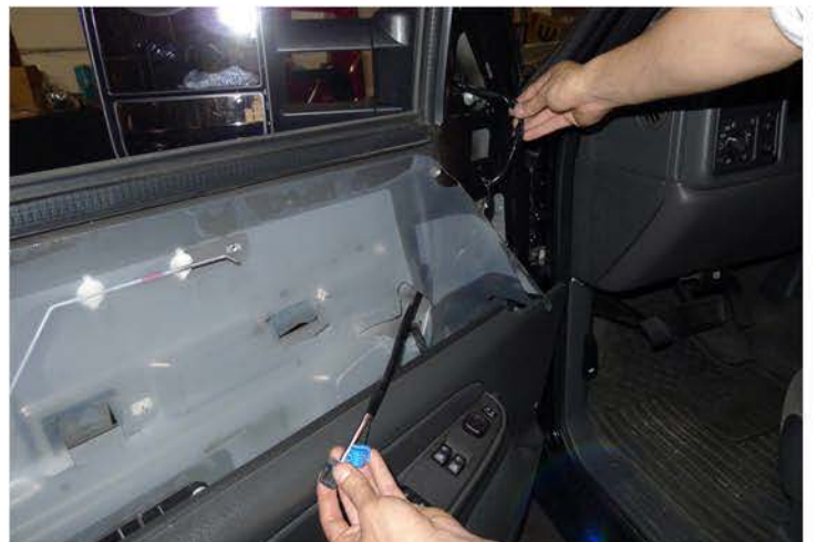
22. Run the mirror harness under the plastic sheet
