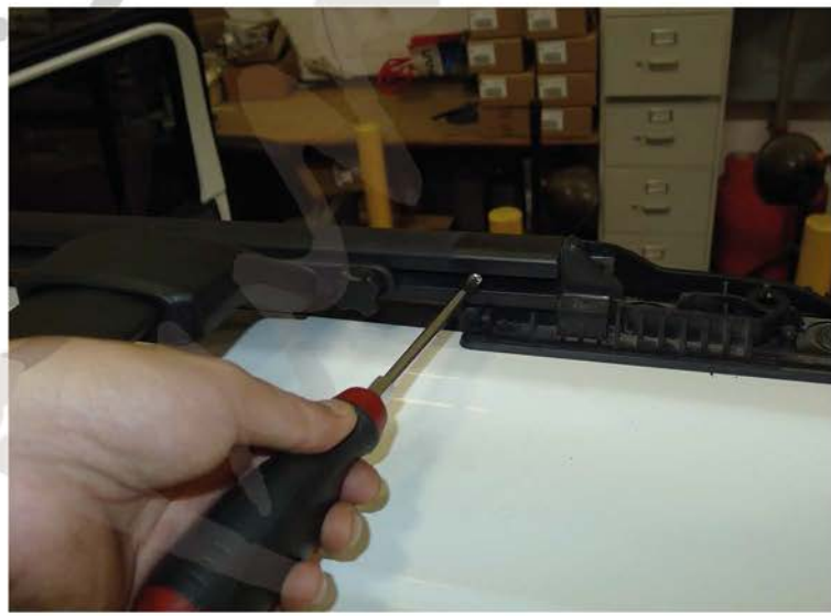
15. Install the phillips head screw into the hole towards the rear end of the roof rack.
