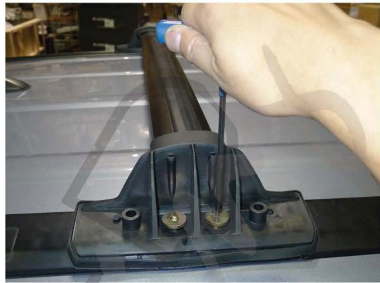
12. Line up the mounting holes then secure roof rack with the allen headed hardware
