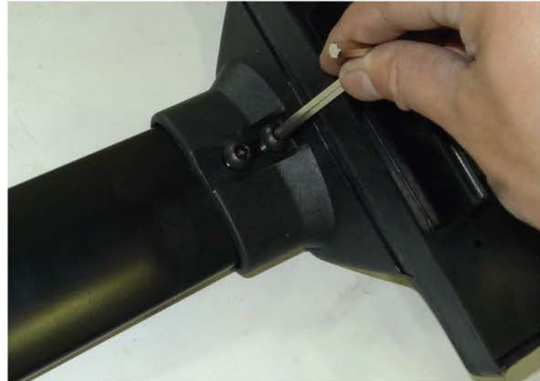
10. Secure mount to rail with the (2) allen headed bolts
