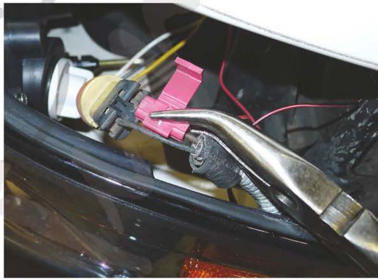
14. Connect the DRL wires to the 12v power wire
