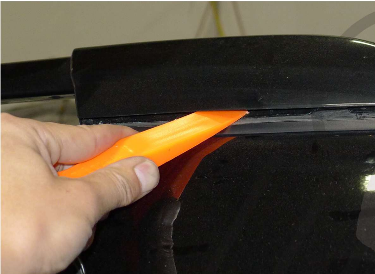
13. Remove the roof rack support cover
