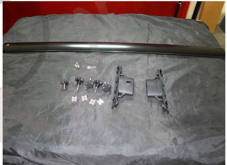
2. Assemble crossrail components
