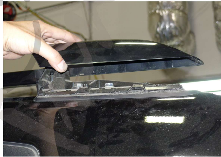
14. Remove the roof rack support cover
