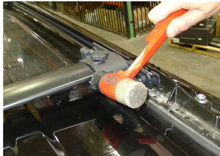
16. Tap crossrail into position with the mallet
