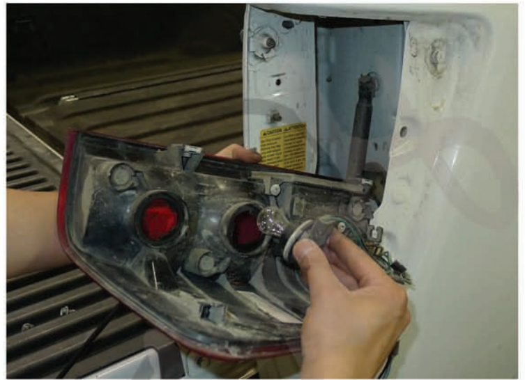
6. Remove the brake light sockets
