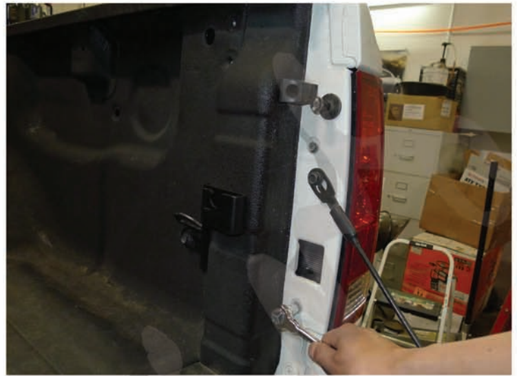
18. Tighten the (2) 10mm bolts
