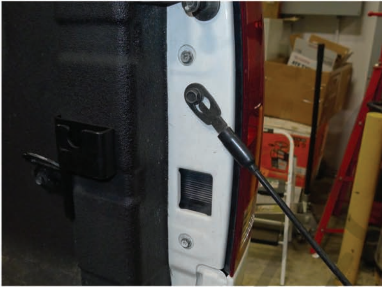
1. (2) 10mm bolts location
