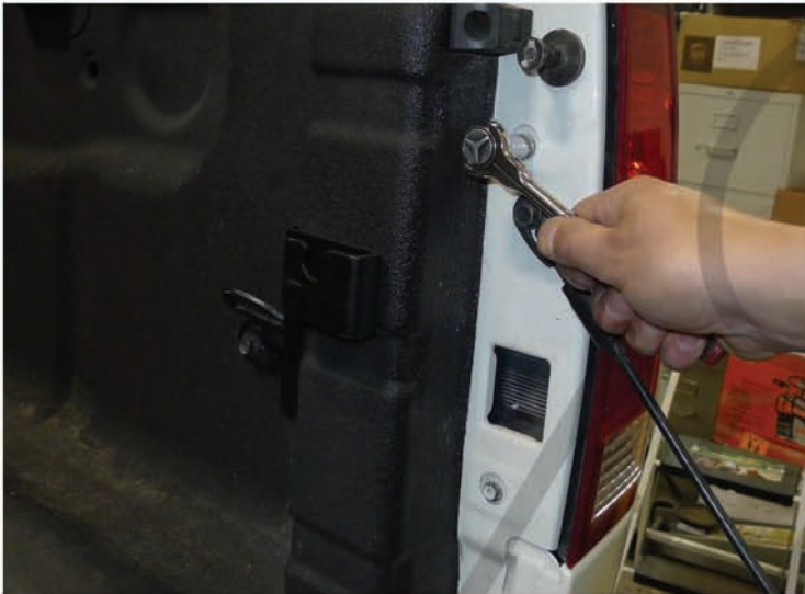
19. Tighten the (2) 10mm bolts Please repeat the picture order from 1 to 19 for the opposite side
