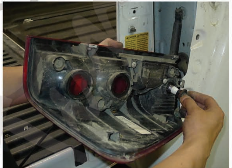
8. Remove the brake light sockets
