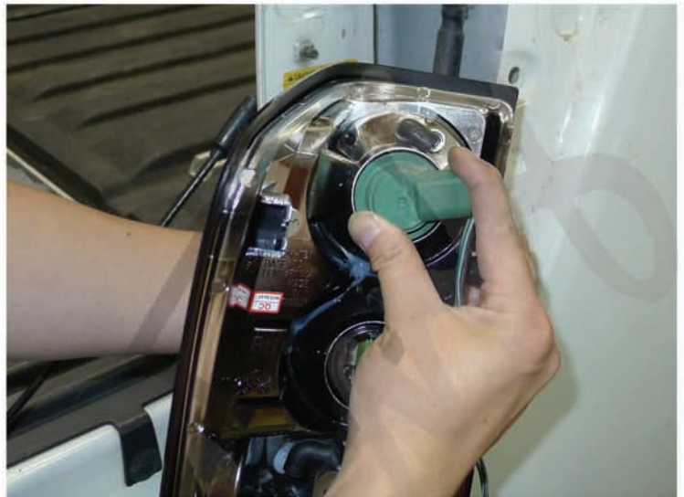
12. Install the taillight socket to the LED taillight housing
