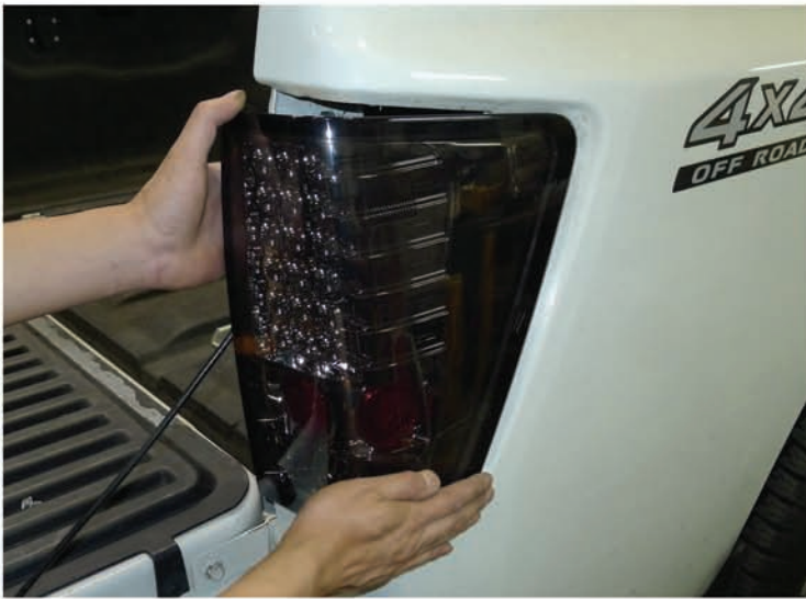
17. Place the LED taillight in the stock location please see the "L.E.D. TAIL LIGHT installation instruction" If your Tail light don't have L.E.D. You can skip the the installation instruction.
