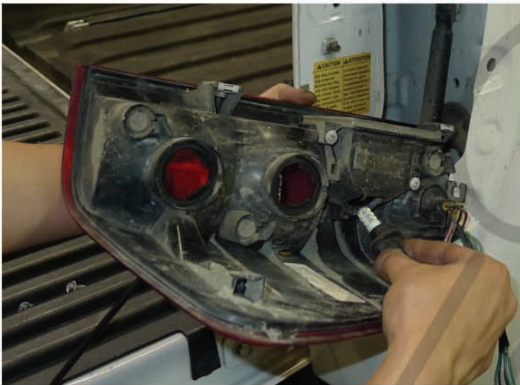
7. Remove the brake light sockets
