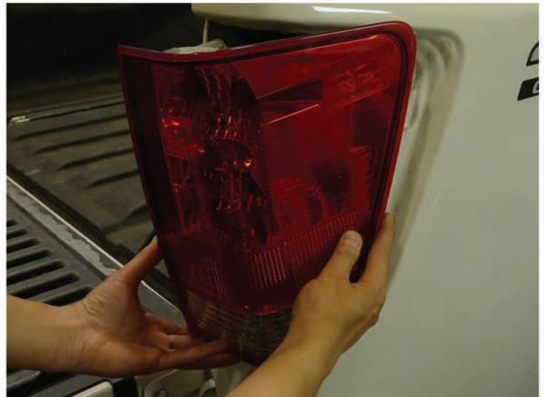
5. Remove the factory taillight
