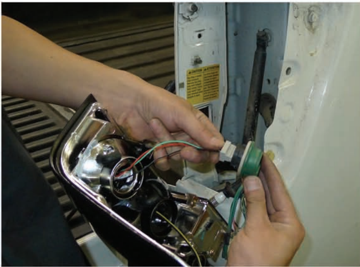
11. Connect the LED taillight harness to the taillight socket please see the "L.E.D. TAIL LIGHT installation instruction" If your Tail light don't have L.E.D. You can skip the the installation instruction.
