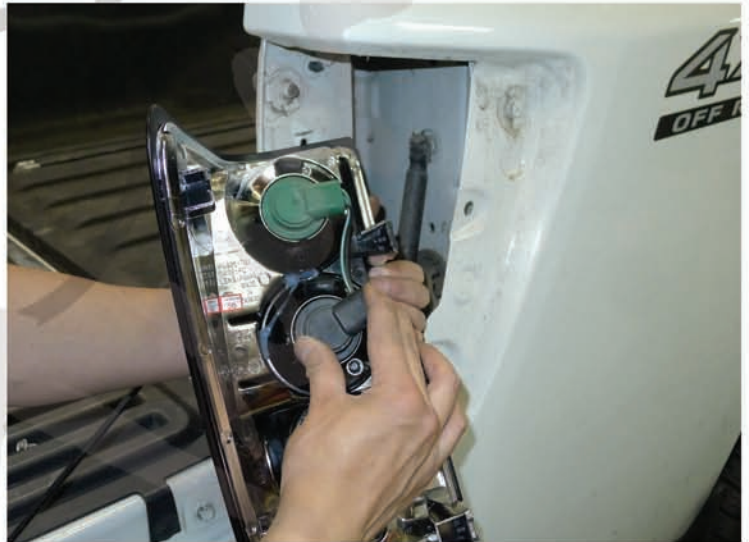
14. Install the taillight socket into the LED taillight
