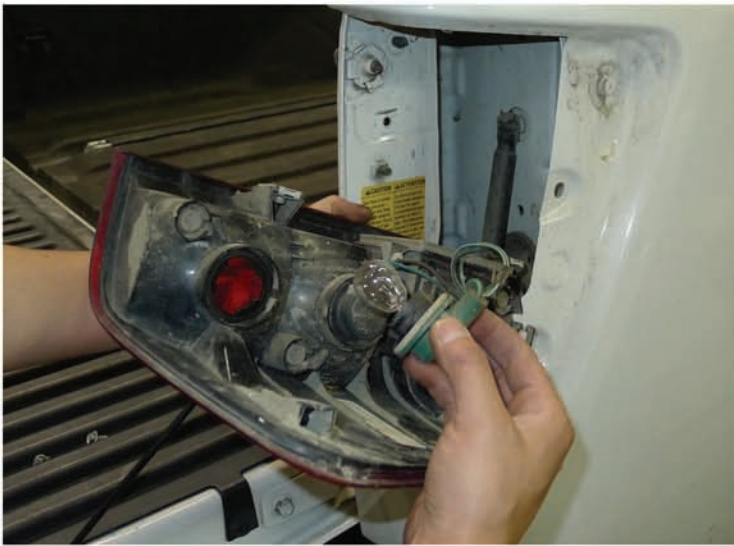
6. Remove the brake light sockets
