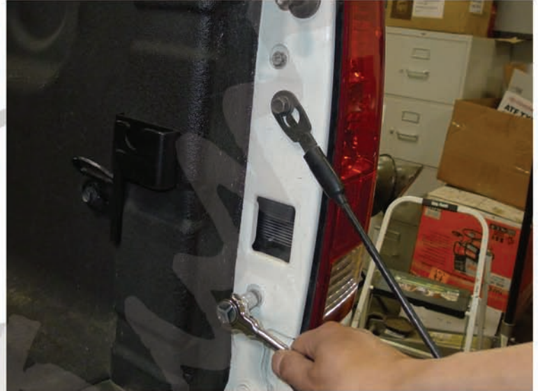
2. Remove the (2) 10mm bolt
