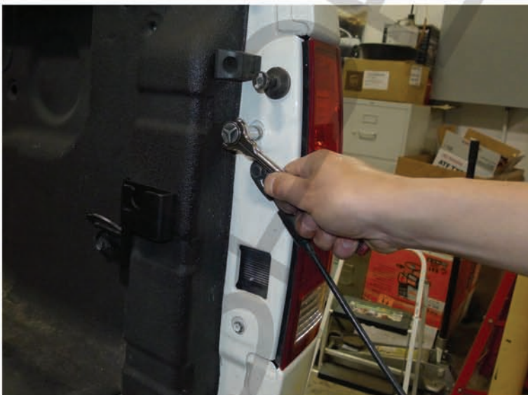
3. Remove the (2) 10mm bolts
