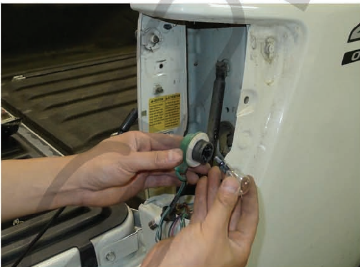
9. Remove the brake light bulbs
