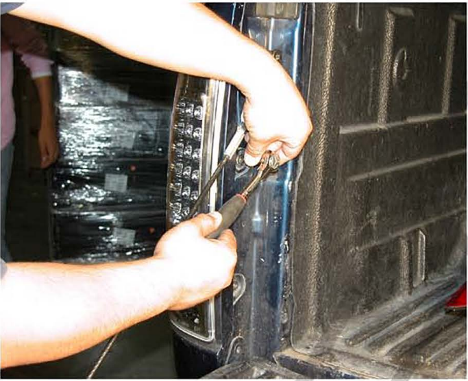
7. Install two T20 bolts
