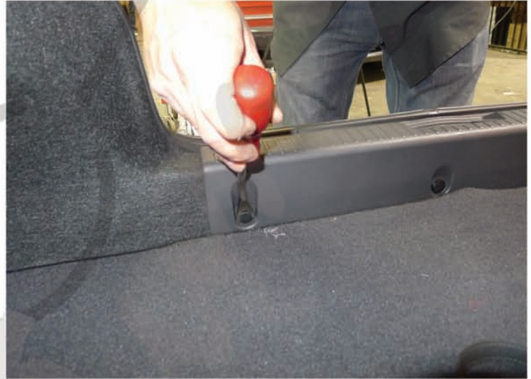
2. Remove the (3) plastic clips
