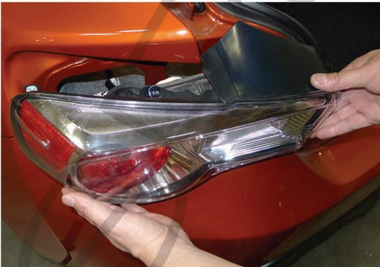
9. Remove the factory tail light
