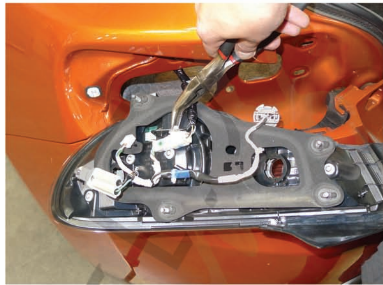
12. Remove the tail light harness from the tail light
