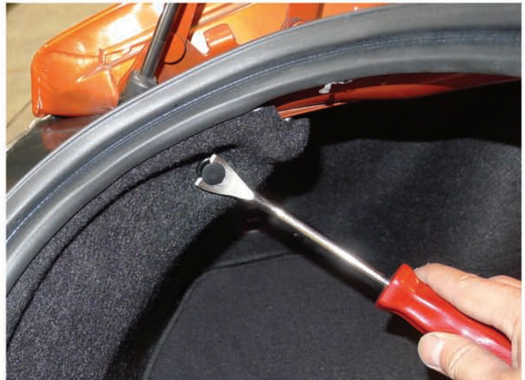
4. Remove the plastic clip
