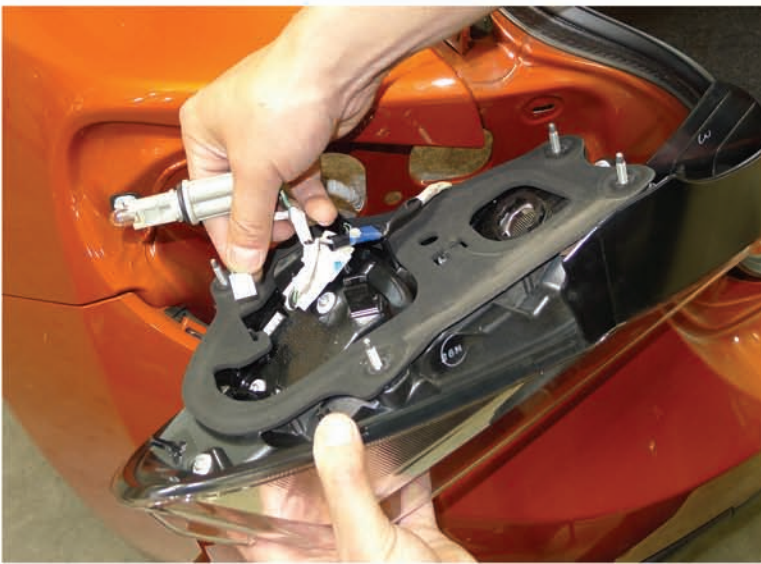
11. Disconnect the tail light harness
