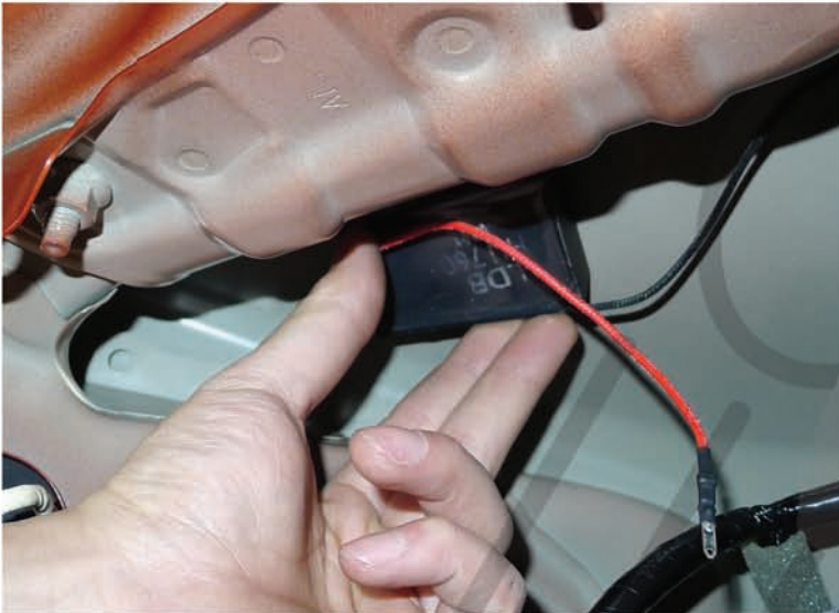
19. Place and attach the resistor on inside roof on the rear panel
