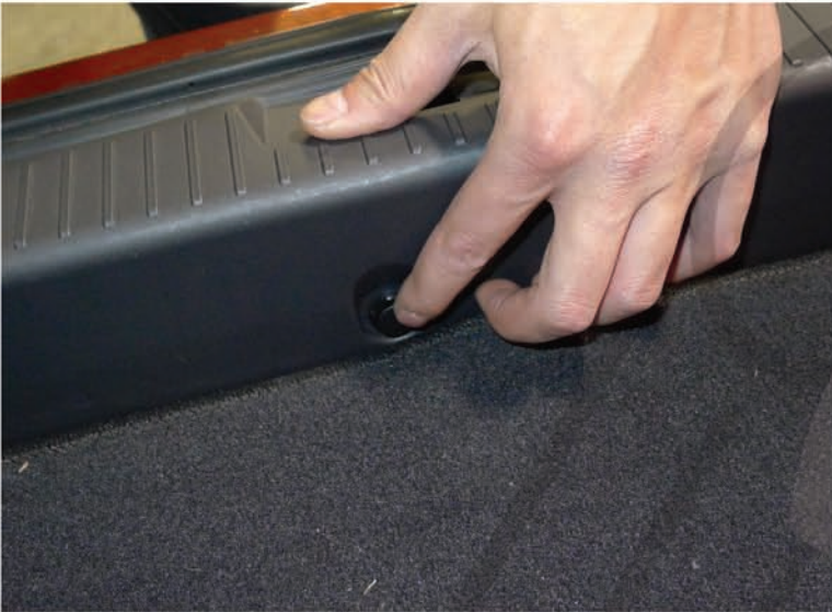
25. Replace the (3) plastic clips
