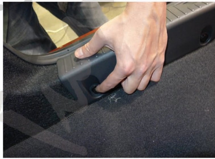
26. Replace the (3) plastic clips
