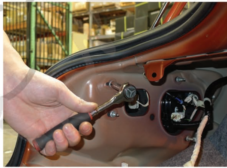
8. Remove the (4) 8mm nuts
