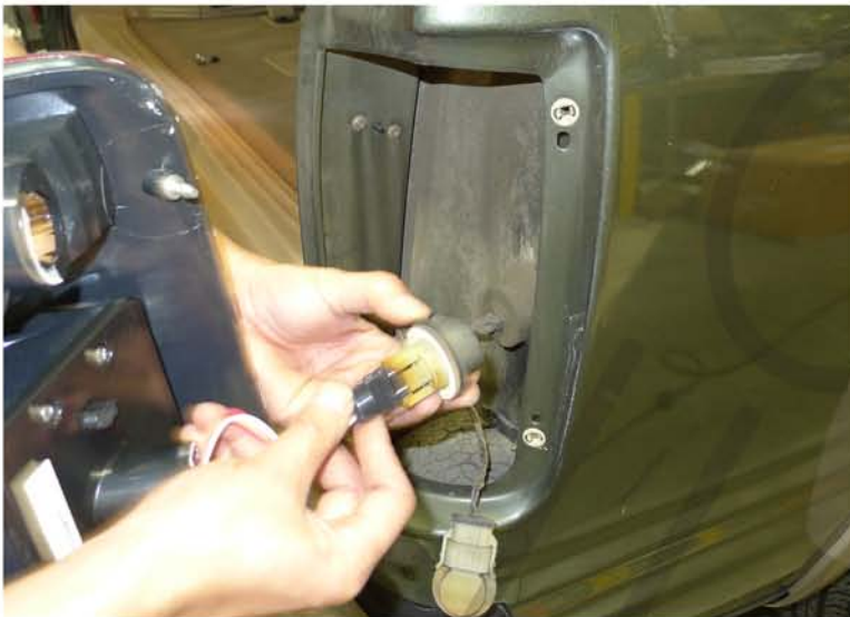
7. Connect the LED taillight harness to the taillight socket Please see the " L.E.D. tail lights installation instructions" If your tail lights don't have L.E.D. you can skip the installation instructions.
