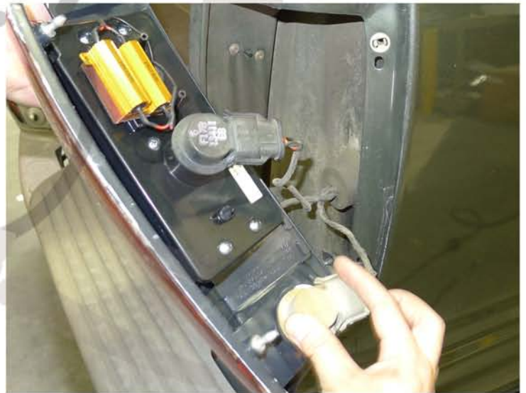
8. Install the taillight socket into the LED taillight Install the reverse light socket into the LED taillight
