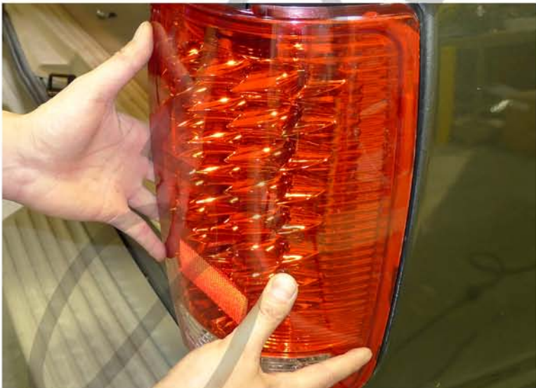
9. Place the LED taillight in the stock location Please repeat the steps in order from 1 to 9 for the opposite side.
