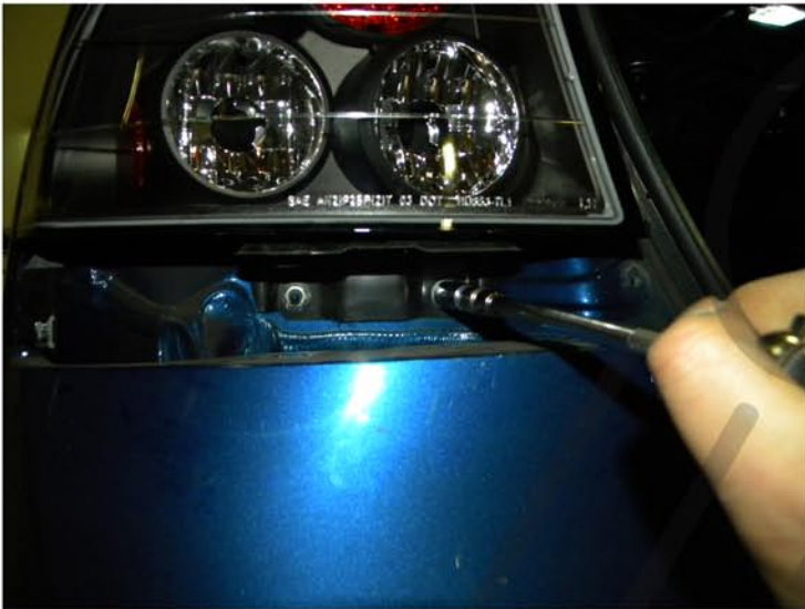
19. Place the new light in the stock location, and tighten the (2) 10mm nuts
