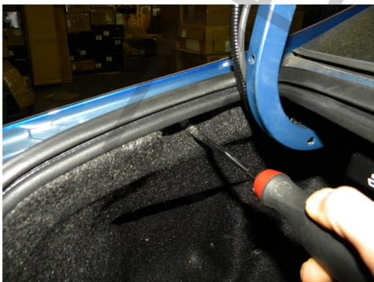
9. Remove the (3) plastic clips
