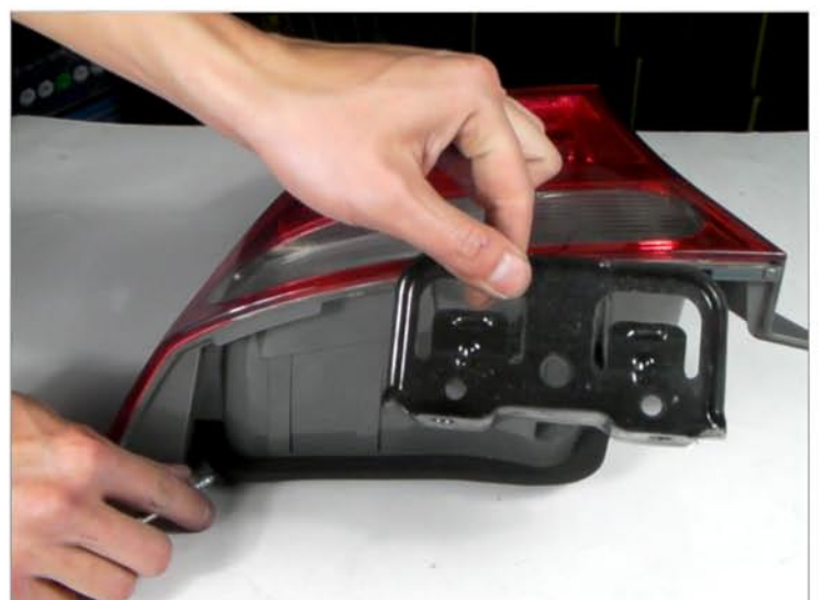
16. Remove the bracket
