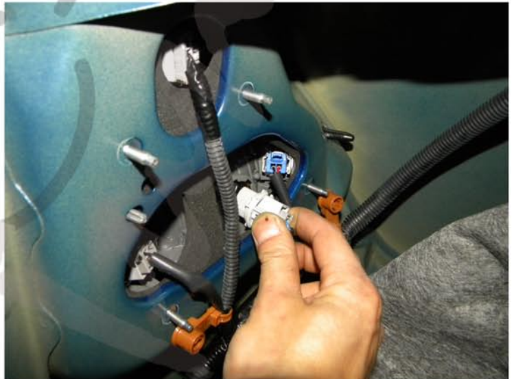
14. Remove the tail light harness
