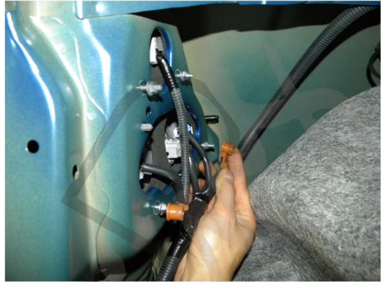
12. Remove the plastic harness holder
