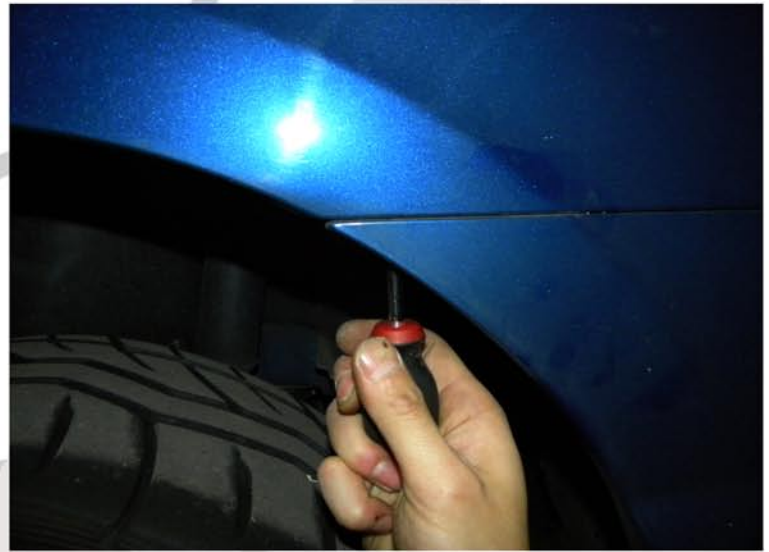
2. Remove the phillips head screw
