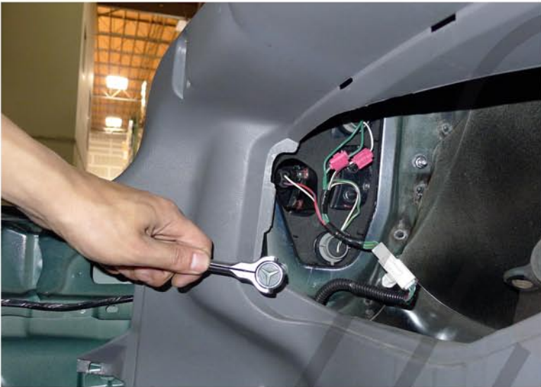
13. Tighten the (3) 10mm nuts
