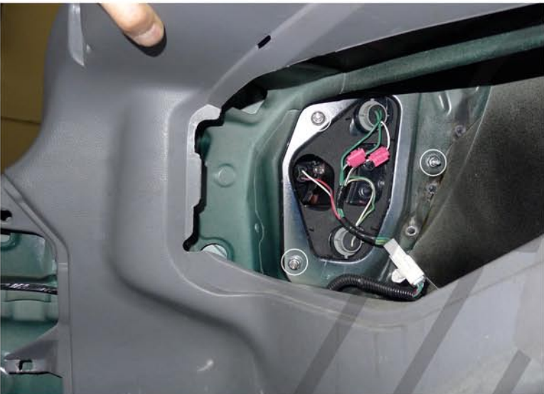
7. Pull the trunk side inner panel to the access the (3) 10mm nuts
