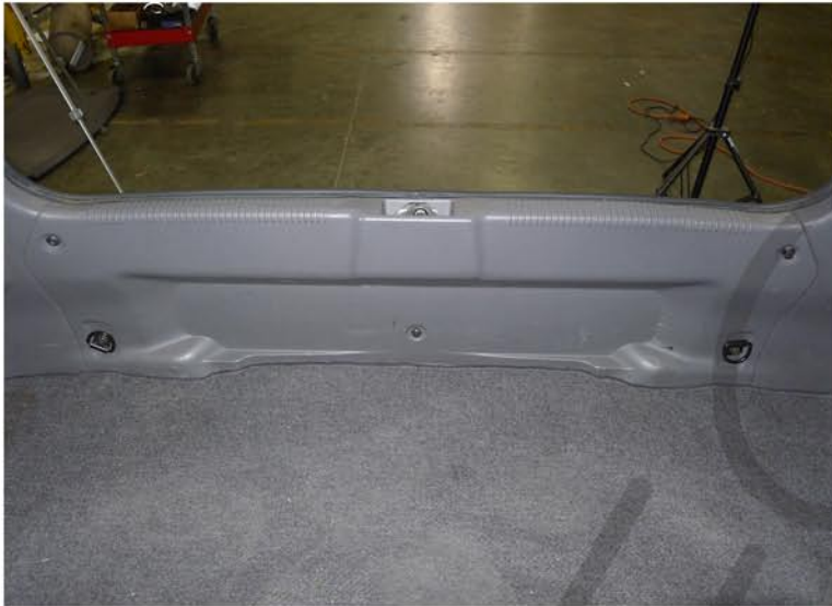
1. (3) Plastic clips and the (2) 10mm bolts location
