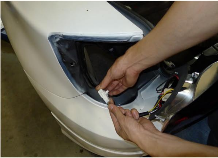
11. Connect the tail light harness to the LED tail light Please see the " L.E.D. tail lights installation instructions" If your tail lights don't have L.E.D. you can skip the installation instructions.
