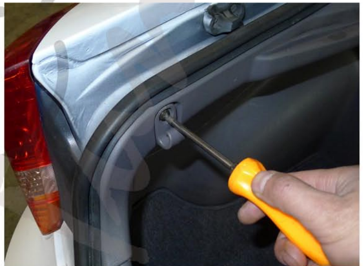
14. Replace the trunk inner panel and tighten the phillips head screw
