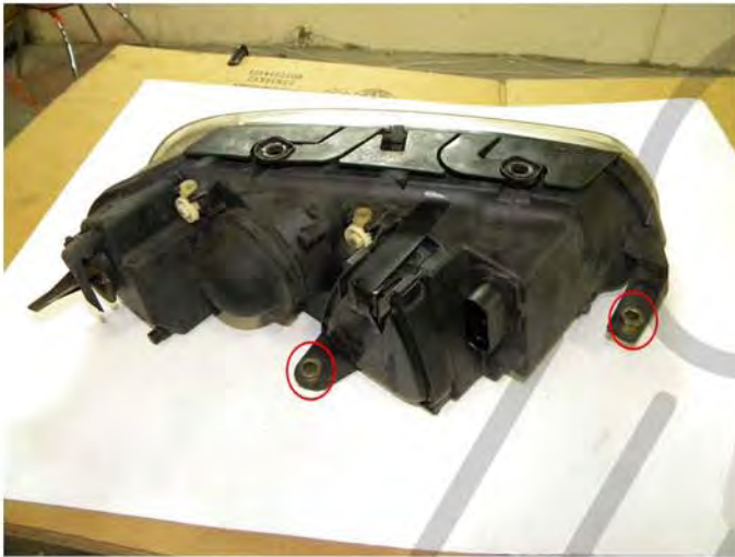
19. Remove two nuts from the OEM headlight
