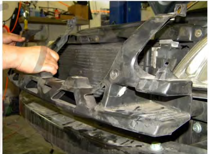
14. Remove the front bumper support
