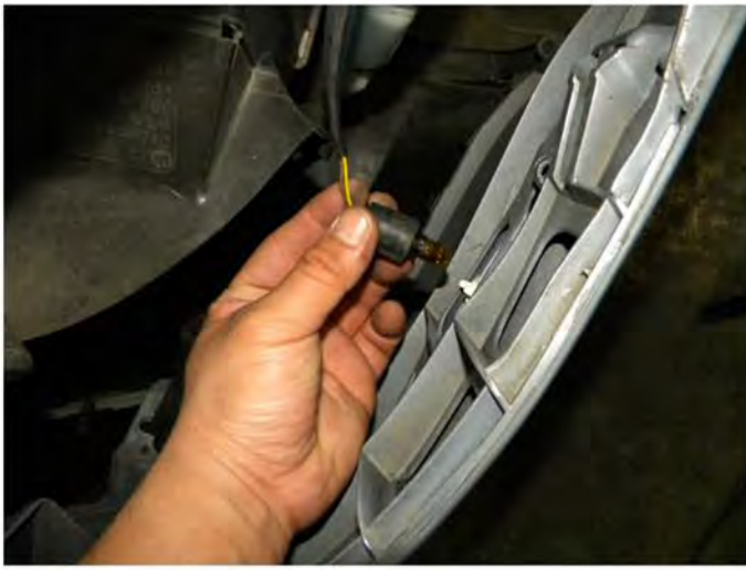
23. Connect driving light socket Please see the "Halo and L.E.D installation instructions" If your headlights don't have HALO or L.E.D. You can skip
