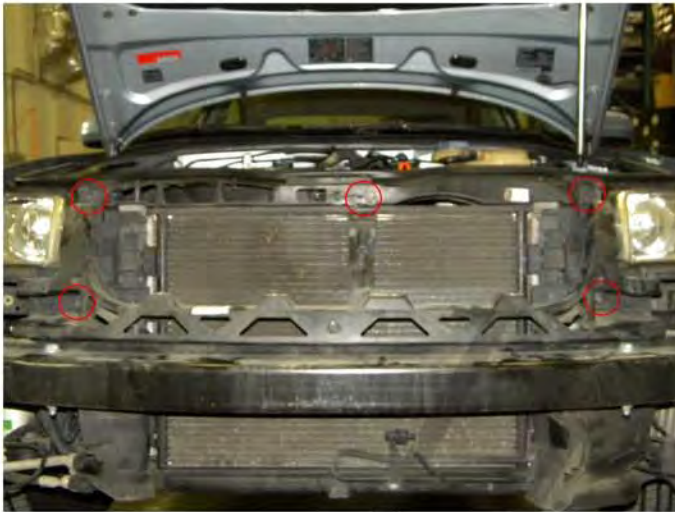
13. Remove five T30 bolts from the front bumper support
