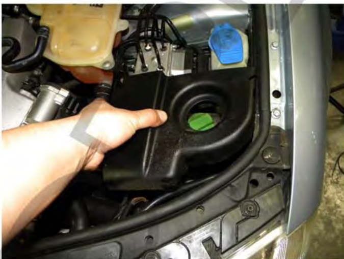
33. Install the cover please repeat the picture order from 1 to 33 for the opposite side
