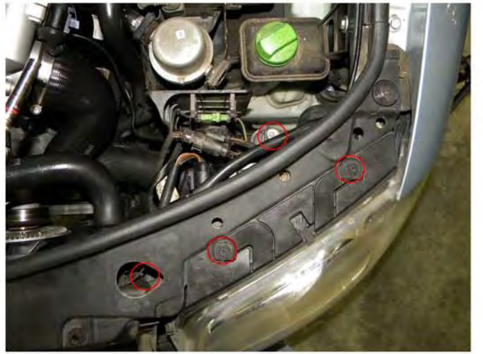
16. Remove four 8mm headlight bolts
