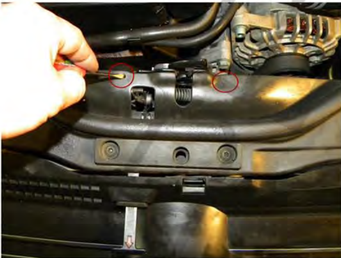
3. Unlock two clips from the hood latch cover then remove the cover
