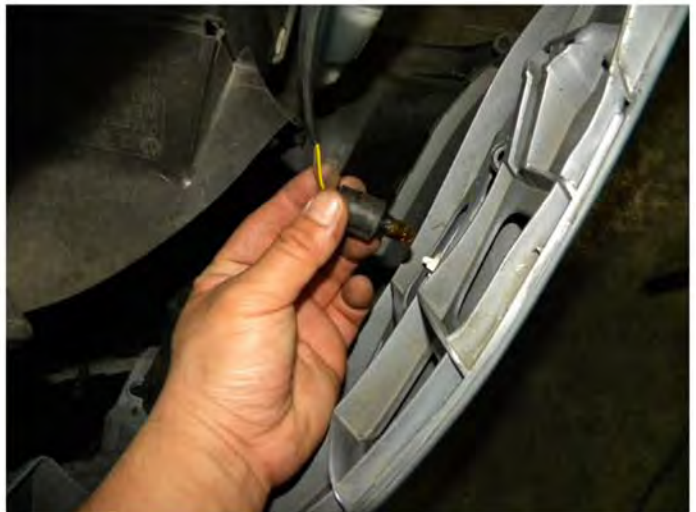
10. Disconnect the driving light socket
