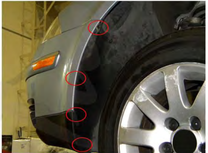
8. Remove four T25 bolts from the side of the bumper
