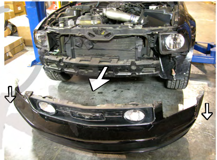
8. Before you remove the bumper, pull the both side down first and then pull out the bumper ( Please disconnect your OEM fog light's connector before you remove the front bumper if equipped)
