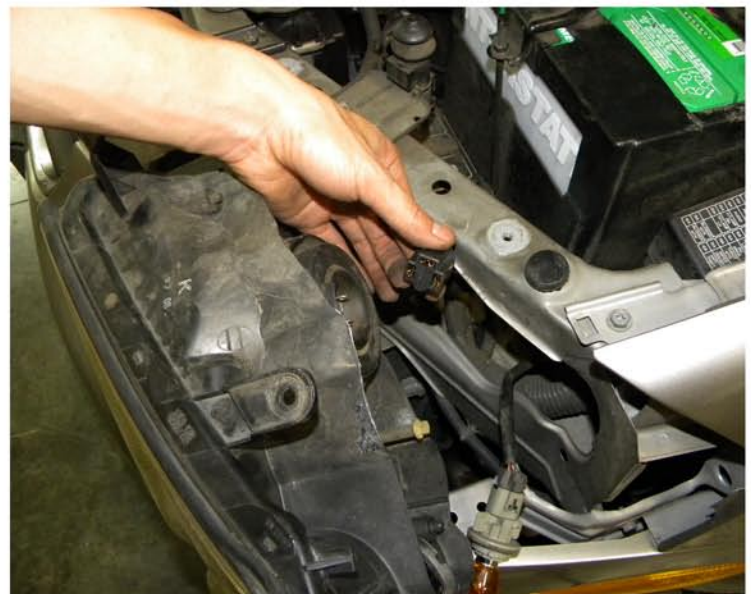
4. Remove the driving light socket and disconnect headlight bulb harness
