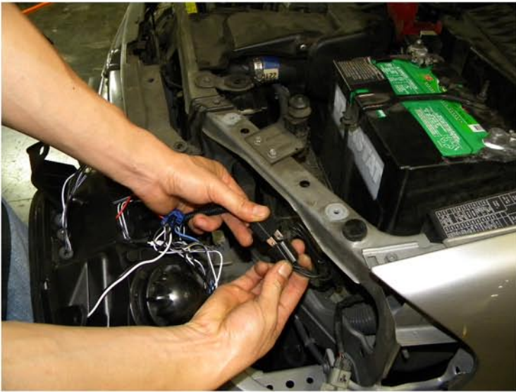
5. Have the new projector ready and put back the driving light socket and connect headlight harness Please see the Halo and L.E.D installation instruction If your headlights don't have HALO or L.E.D. You can skip it
