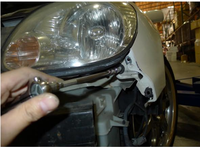
17. Remove the 10mm bolt
