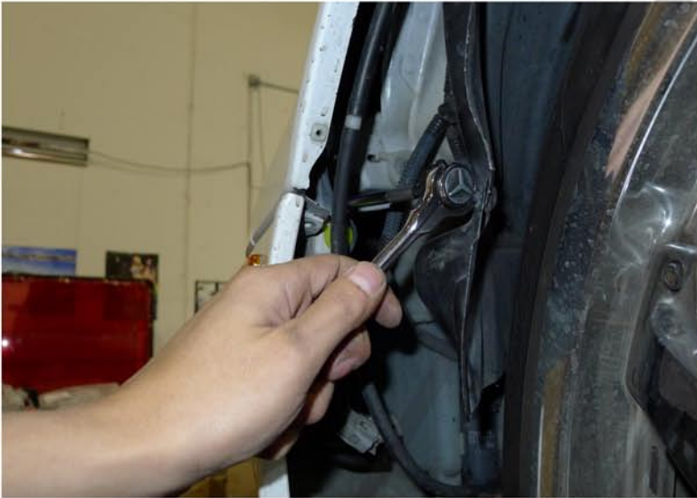
31. Tighten the 10mm nut
