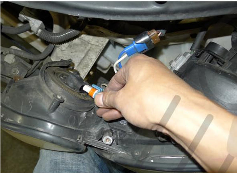
19. Disconnect the headlight harness
