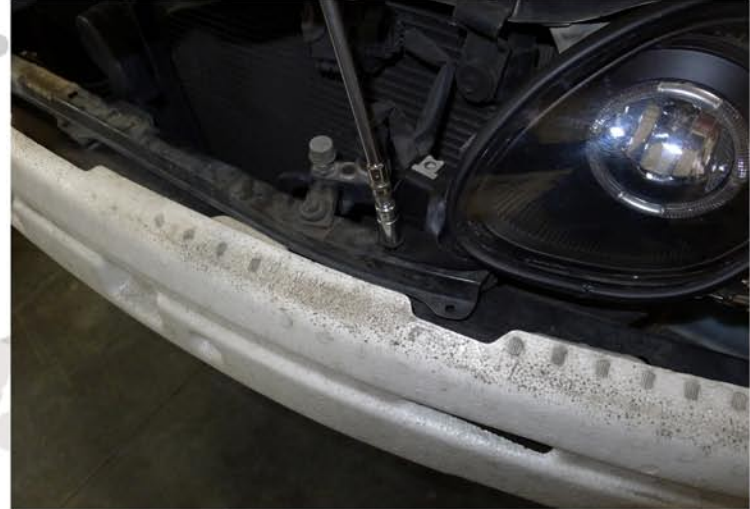
26. Tighten the (3) 10mm bolts
