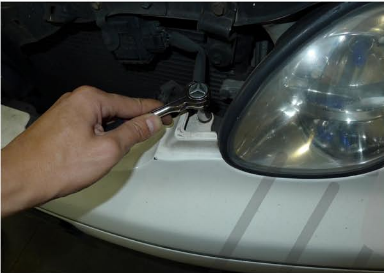
7. Remove the (2) 10mm bolts
