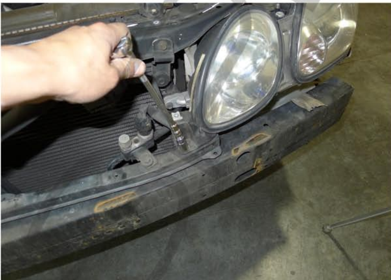
11. Remove the 10mm bolt
