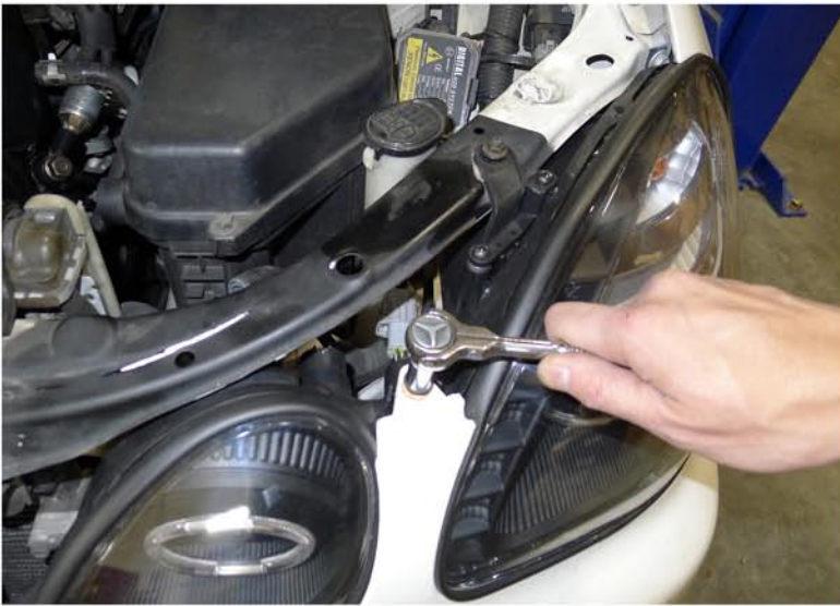
29. Tighten the (2) 10mm bolts
