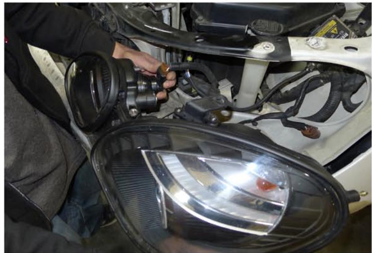
16. Connect the headlight harness to the new headlight
