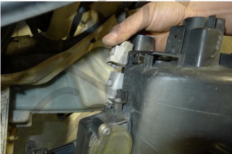
15. Disconnect the headlight harness
