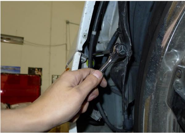
5. Remove the 10mm nut
