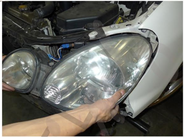
12. Remove the headlight
