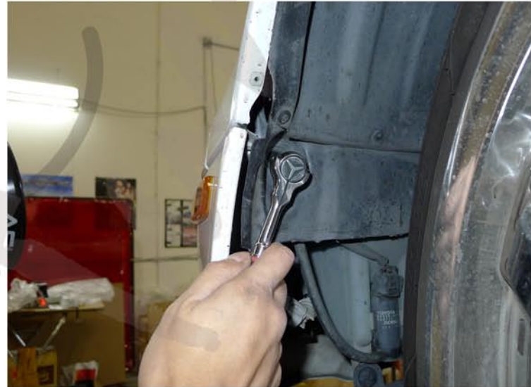
32. Tighten the 10mm screw
