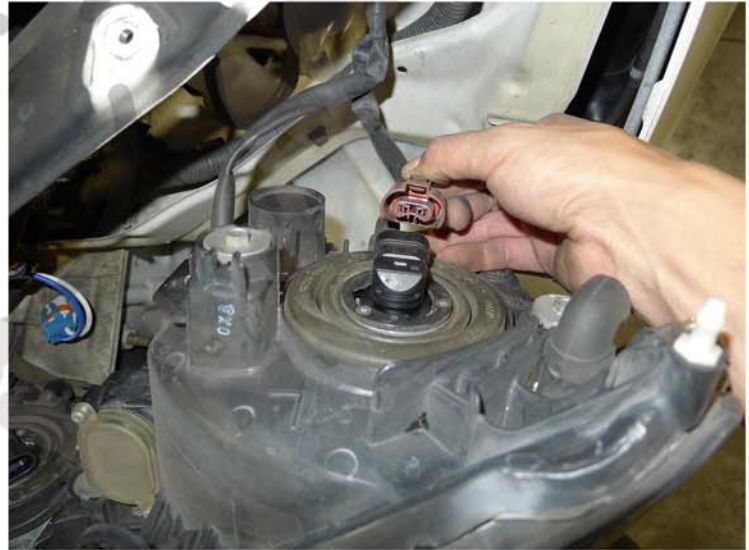
14. Disconnect the headlight harness
