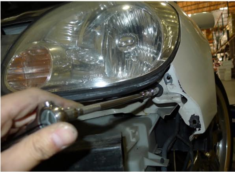
11. Remove the 10mm bolt
