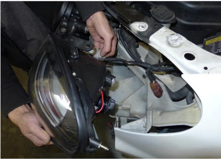
23. Connect the headlight harness to the new headlight
