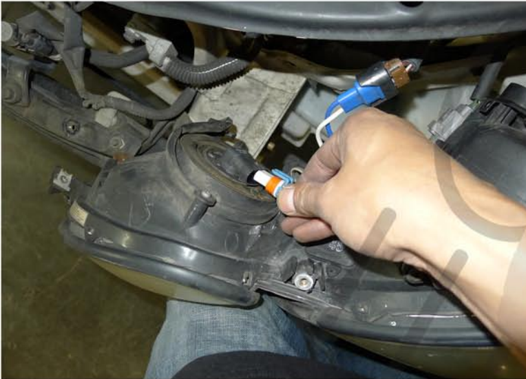
13. Disconnect the headlight harness
