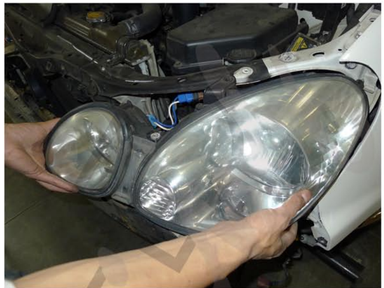
18. Remove the headlight
