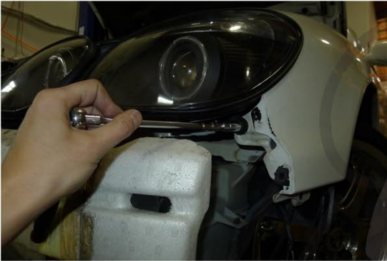
25. Tighten the (3) 10mm bolts
