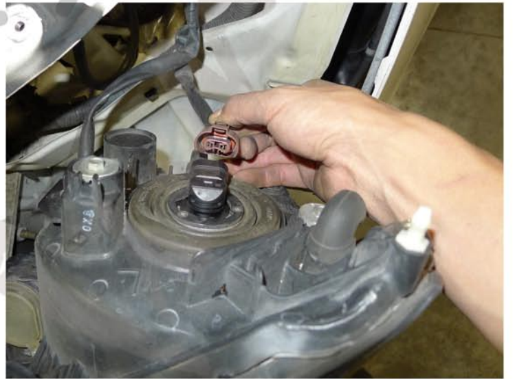
20. Disconnect the headlight harness
