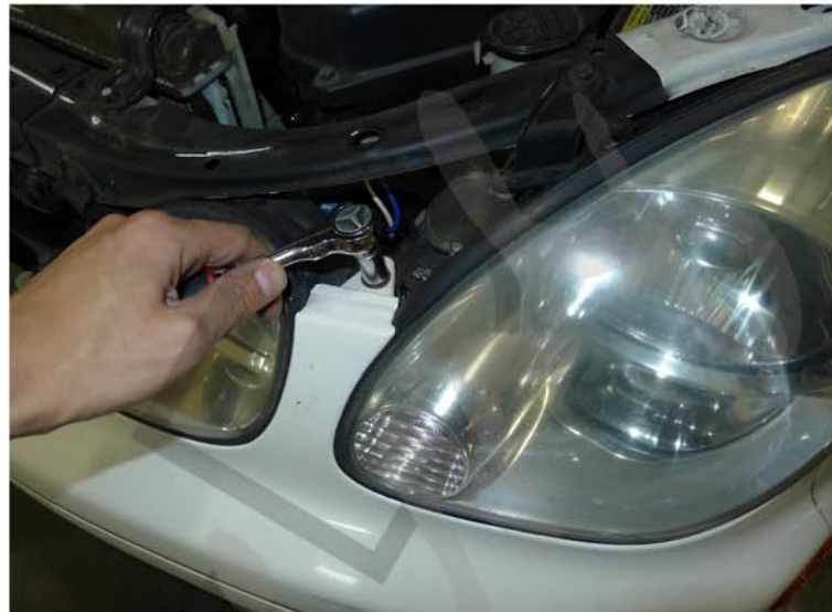
6. Remove the (2) 10mm bolts
