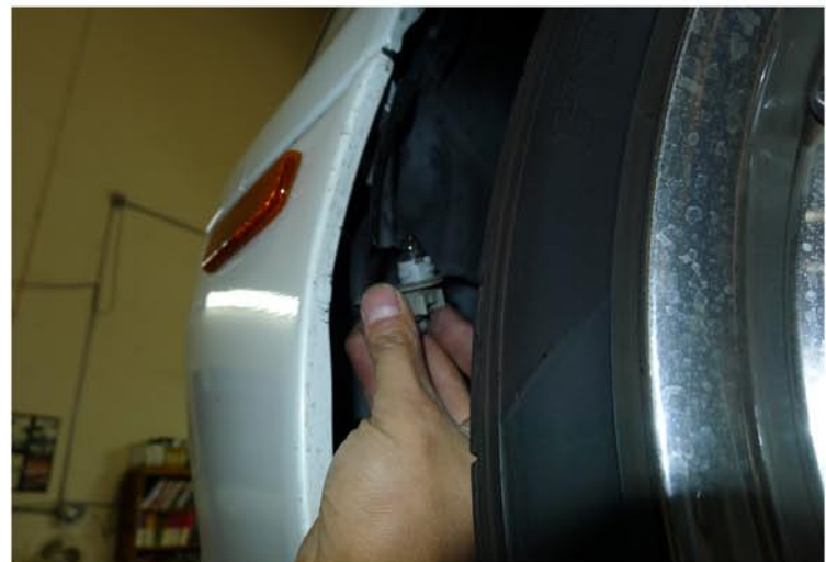
34. Connect the bumper light socket
