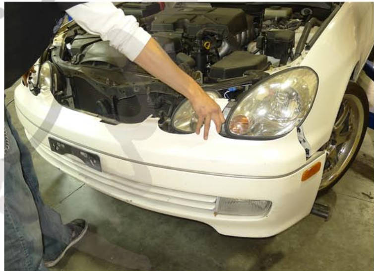
8. Remove the front bumper
