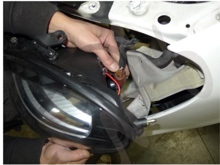
24. Connect the headlight harness to the new headlight
