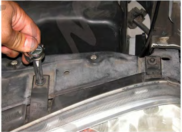
14. Use 8mm socket to remove the two bolts from the top of the headlight
