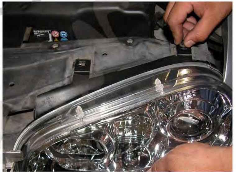
20. Use 8mm socket to install the two bolts to the top of the headlight
