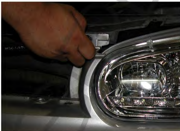
21. Reinstall the two clips removed from earlier
