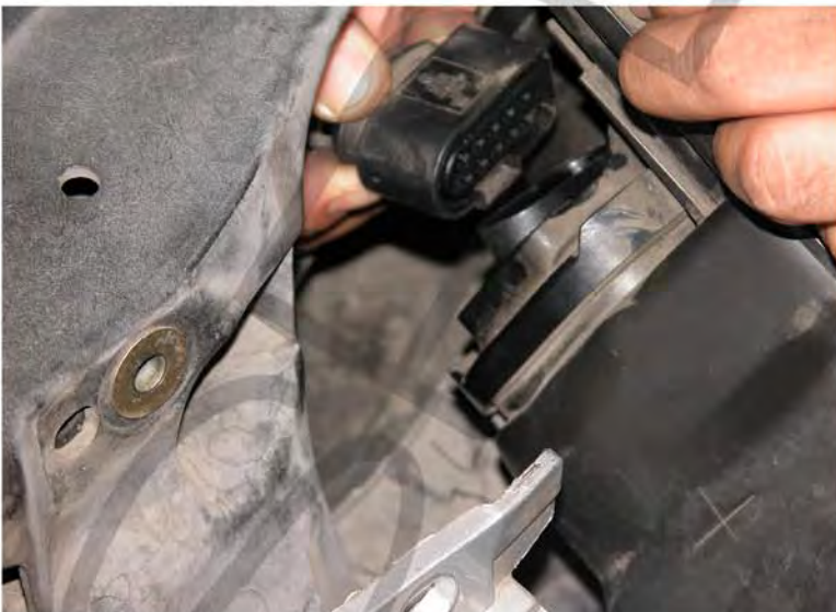
15. Disconnect the harness from the headlight
