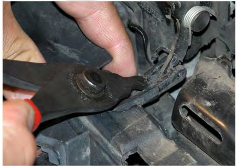
4. Use fixed tip snap ring pliers to prop up the clip and remove the grill
