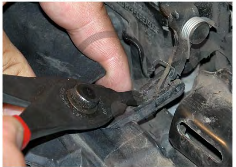
24. Put the grill back and lock the clips to fasten the grill
