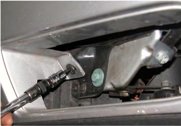
11. Use T30 torx socket to remove the bolt from the fog light spot
