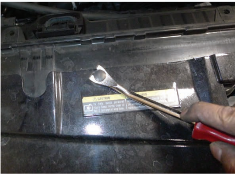
11. Remove the (2) plastic clips
