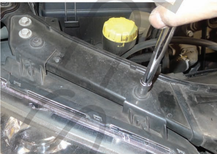
21. Remove the (2) 10mm bolts
