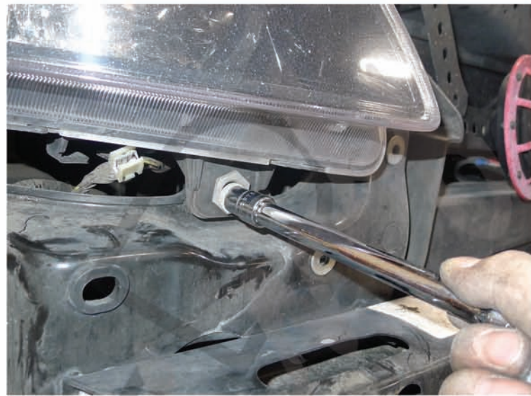
18. Remove the (2) 10mm bolts
