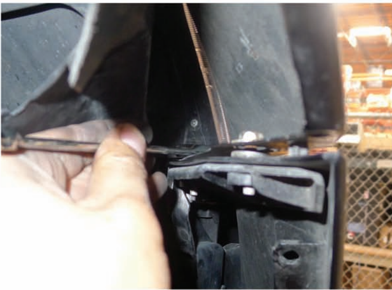
35. Tighten the (2) 10mm bolts
