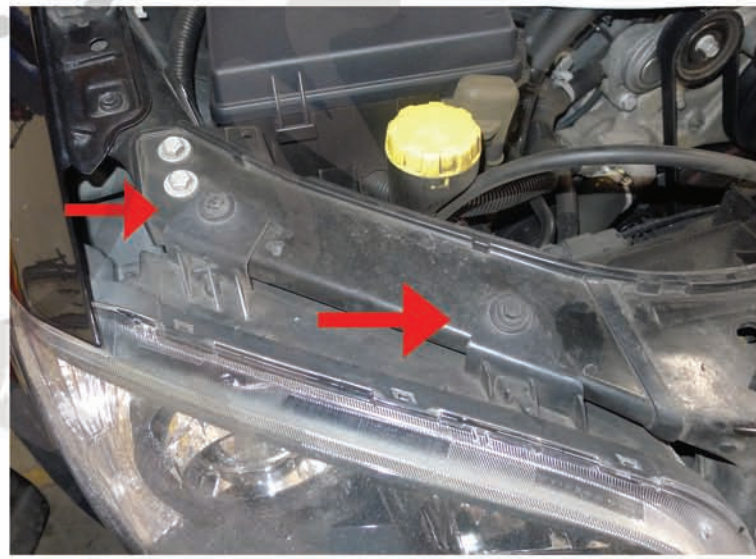
20. Remove the (2) 10mm bolts
