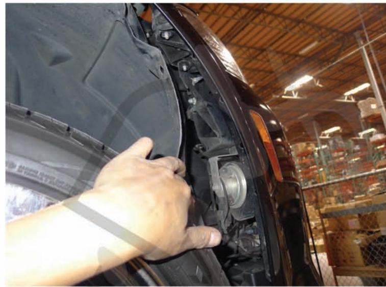
6. Pull the fender liner aside
