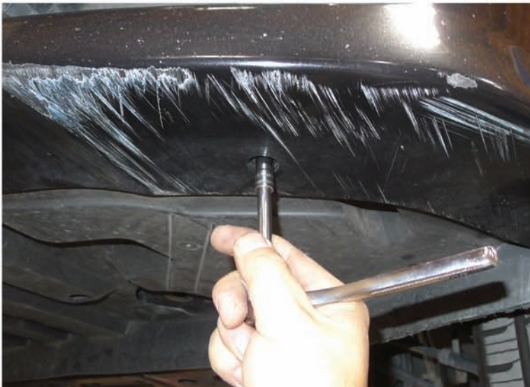
3. Remove the (4) 7mm bolts
