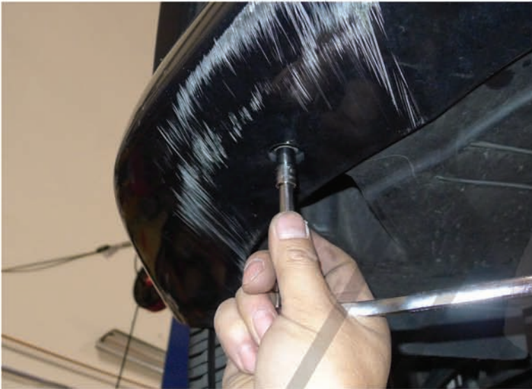
37. Tighten the (4) 7mm bolts Please repeat the steps from 1 to 37 for the opposite side
