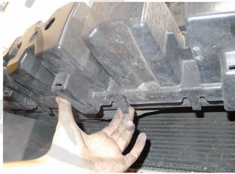
14. Remove the impact absorber
