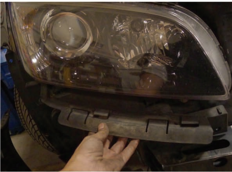
17. Remove the plastic bracket
