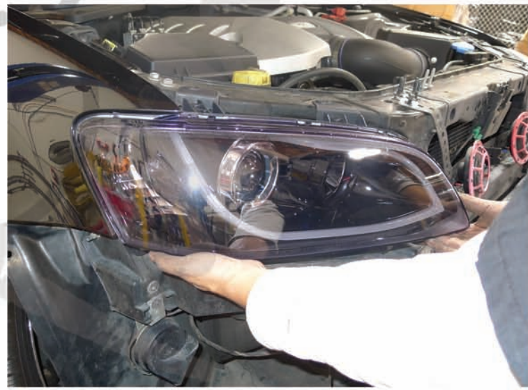
26. Place the new headlight in the position
