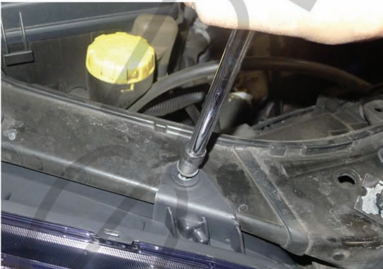
27. Tighten the (2) 10mm bolts
