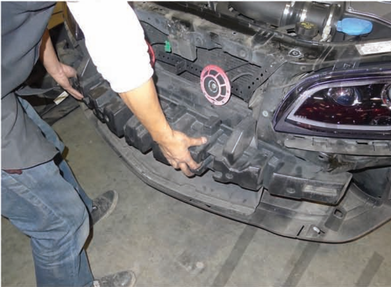
31. Replace the impact absorber
