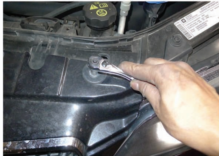
10. Remove the (2) 10mm bolts
