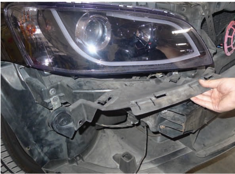
29. Replace the plastic bracket
