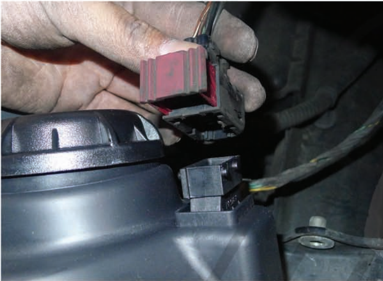
25. Connect the headlight harness to the new headlight
