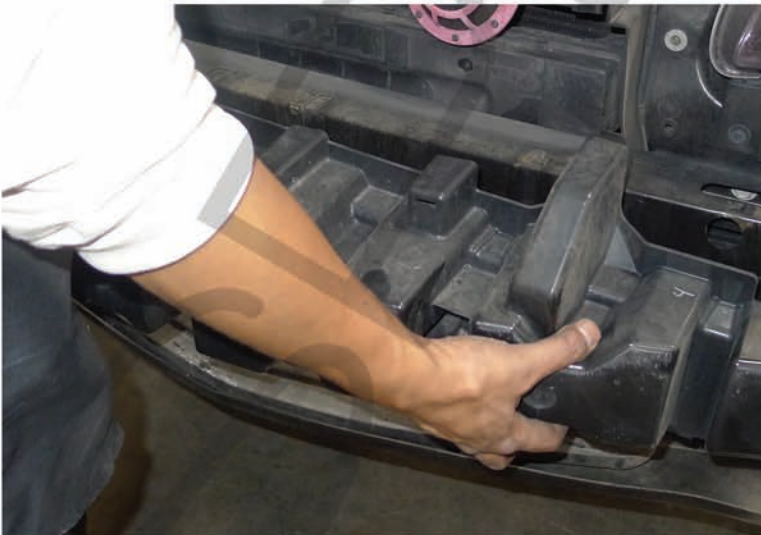
15. Remove the impact absorber
