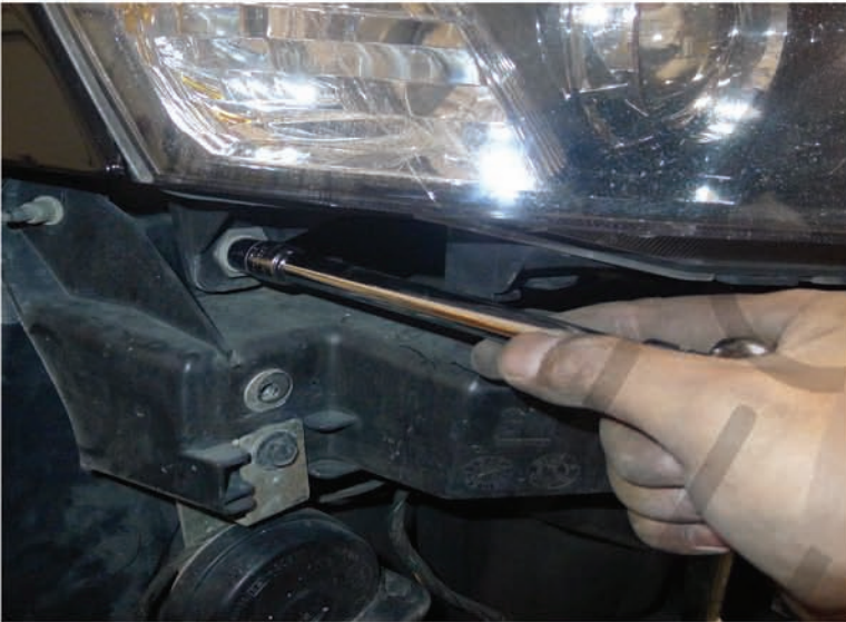
19. Remove the (2) 10mm bolts
