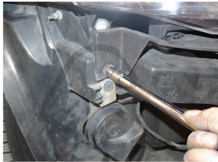
30. Tighten the (2) 10mm bolts
