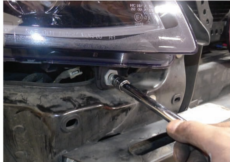
29. Tighten the (2) 10mm bolts
