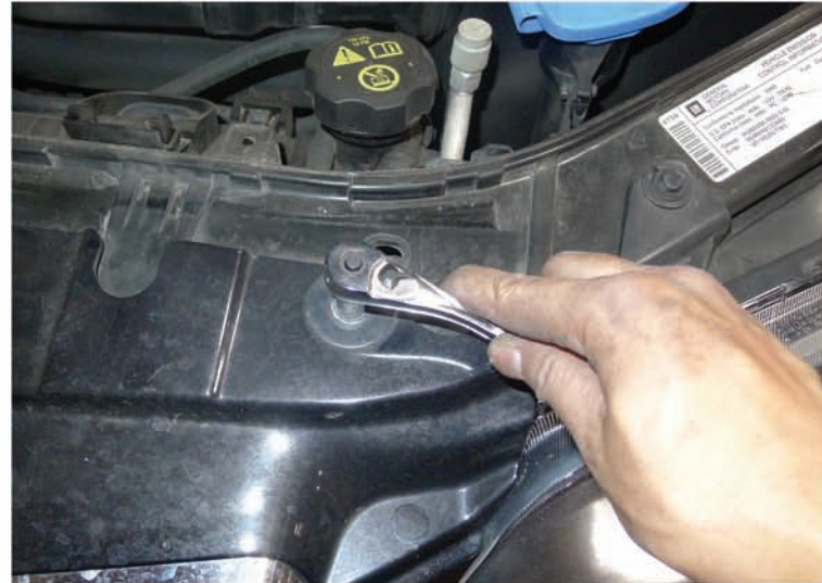
34. Tighten the (2) 10mm bolts
