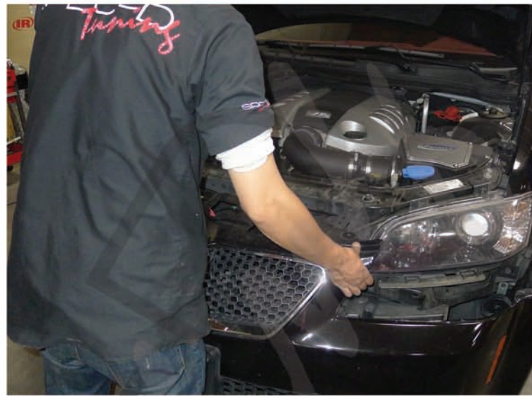
12. Remove the front bumper and set it to the one side
