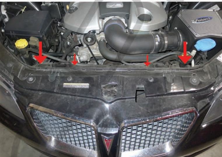
9. (2) plastic clips and (2) 10mm bolts location
