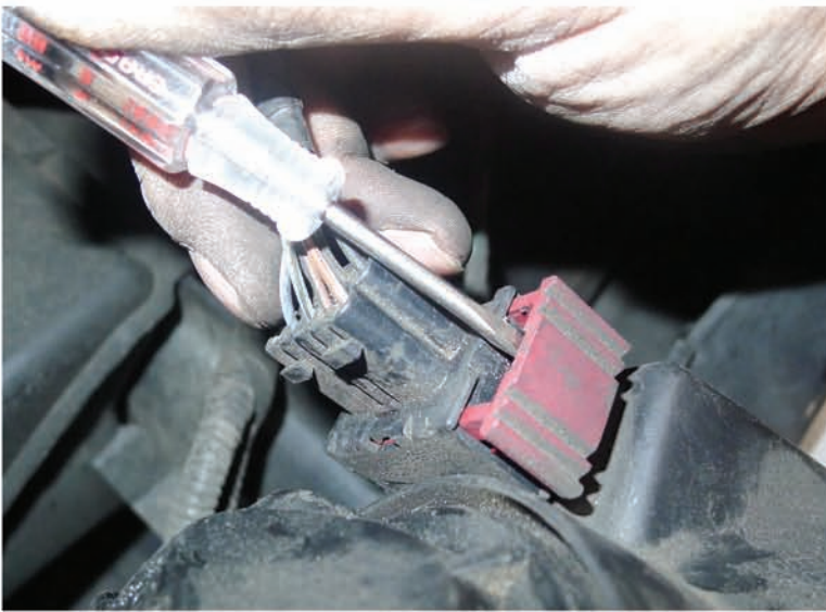
23. Disconnect the headlight harness
