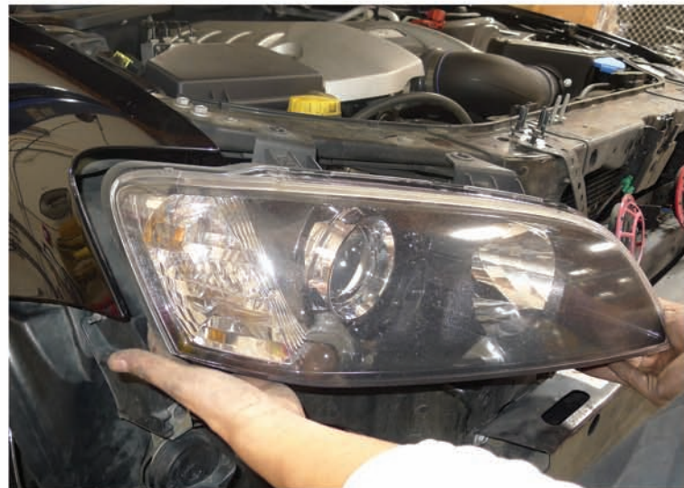
22. Remove the factory headlight
