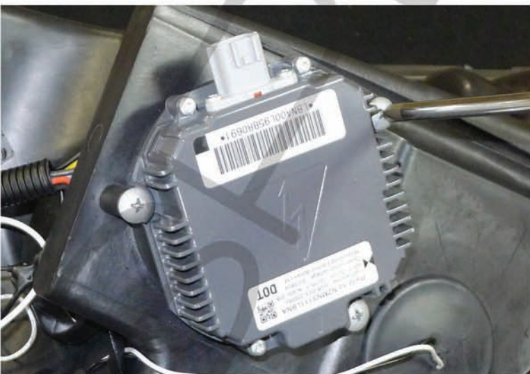
39. Tighten the (3) phillips head screws
