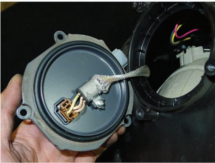
23. Back of the ballast
