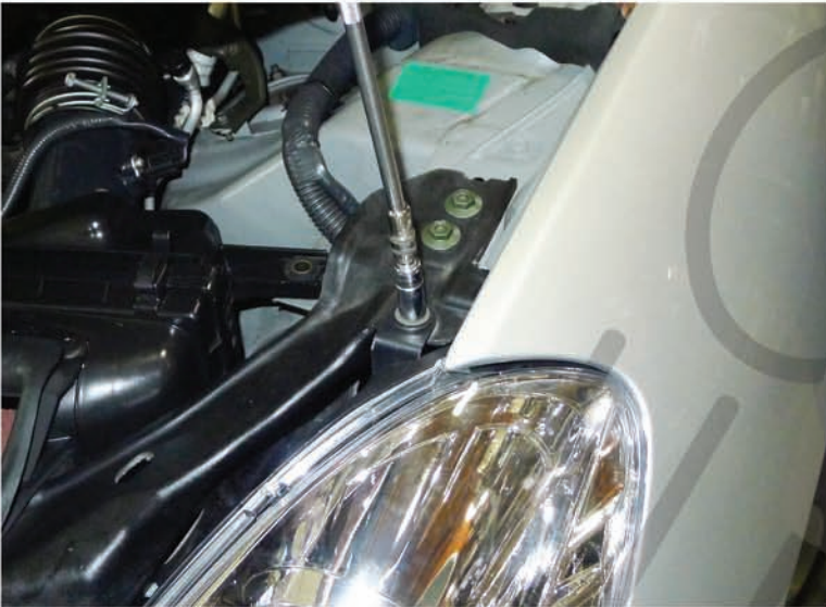
43. Tighten the 10mm bolt
