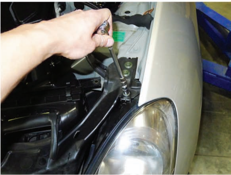
17. Remove the 10mm bolt
