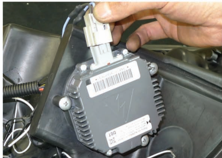
40. Connect the headlight harness to the ballast
