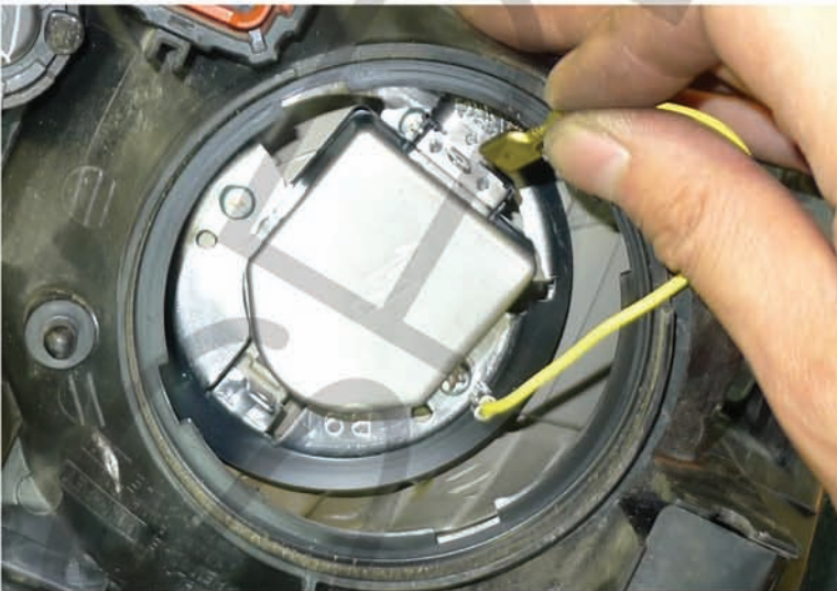
27. Disconnect the ground wire
