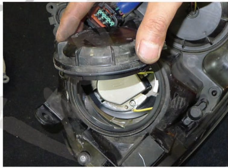
26. Remove the light bulb access hole cover
