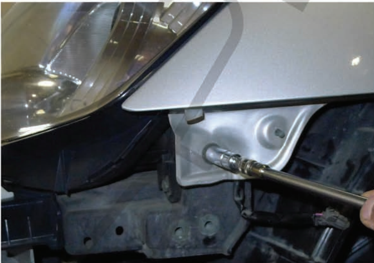
15. Remove the 10mm bolt
