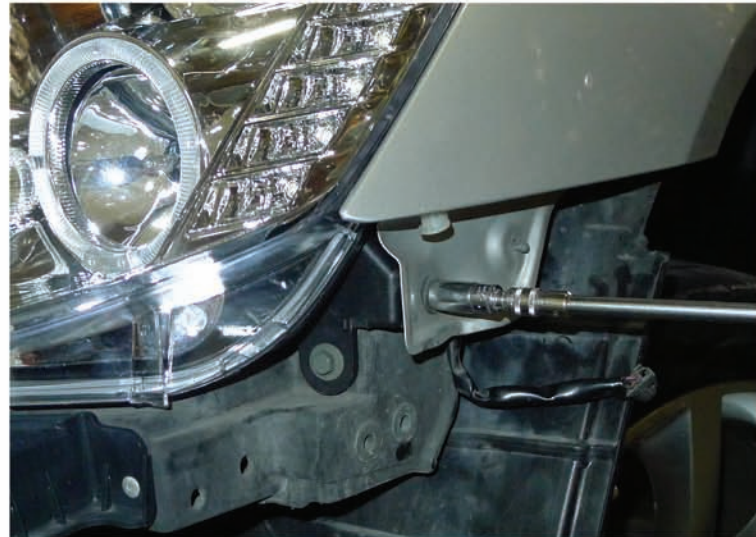
46. Tighten the 10mm bolt
