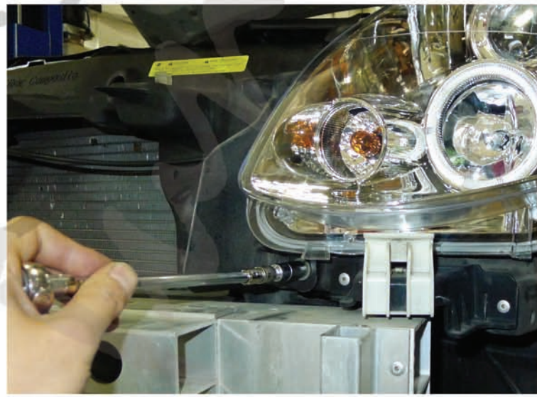
44. Tighten the 10mm bolt
