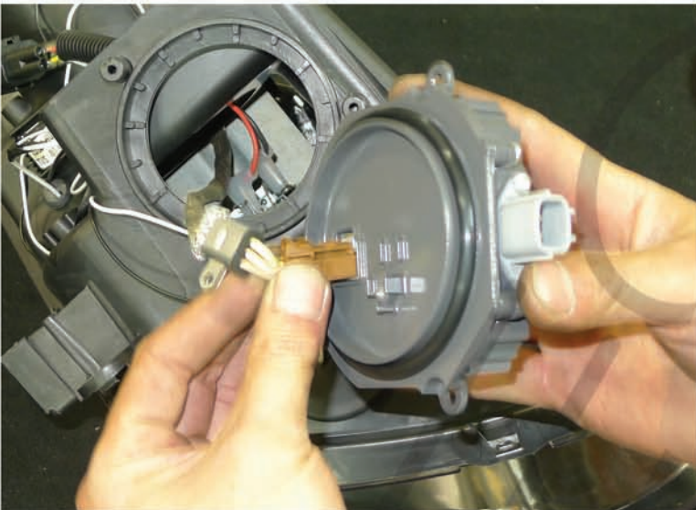
37. Connect the HID socket harness to the ballast
