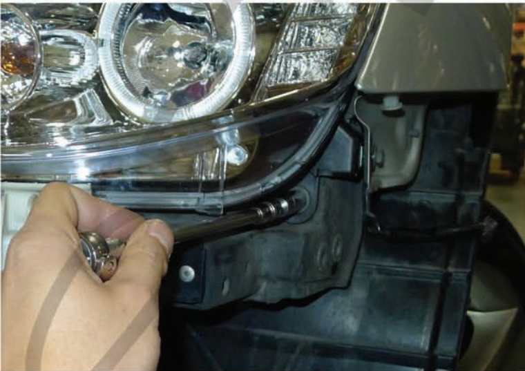
45. Tighten the 10mm bolt
