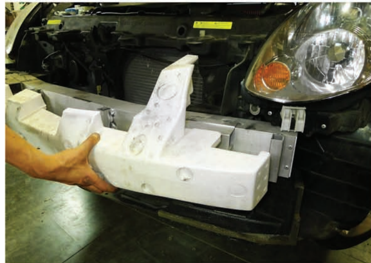
10. Remove the impact absorbing foam
