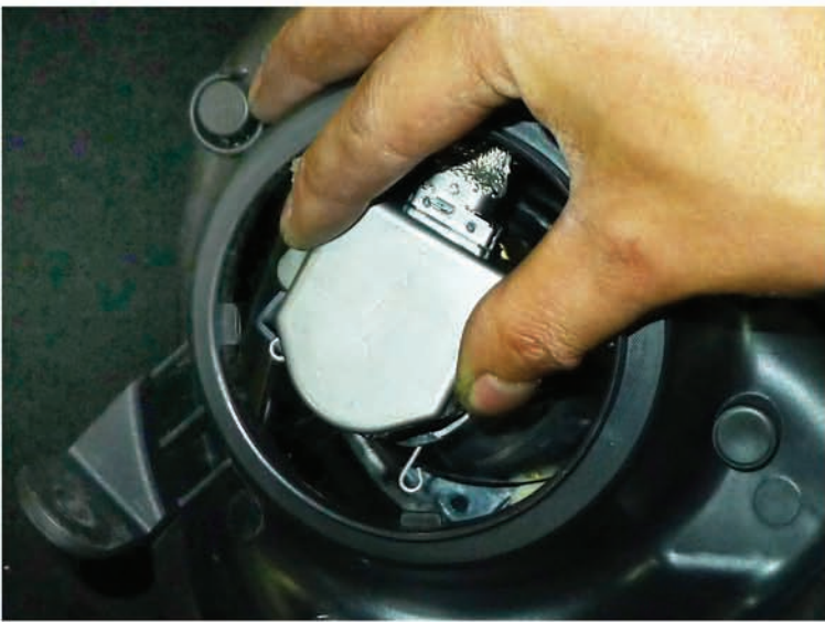
35. Connect the light socket to HID bulb
