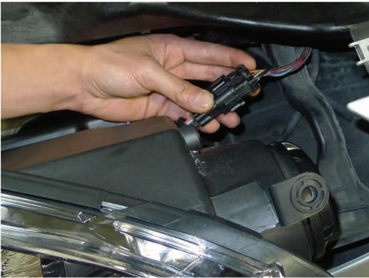
41. Connect the projector headlight to the headlight harness Please see the " L. E. D. headlights installation instructions" If your headlights don't have L.E.D. You can skip the installation instruction.
