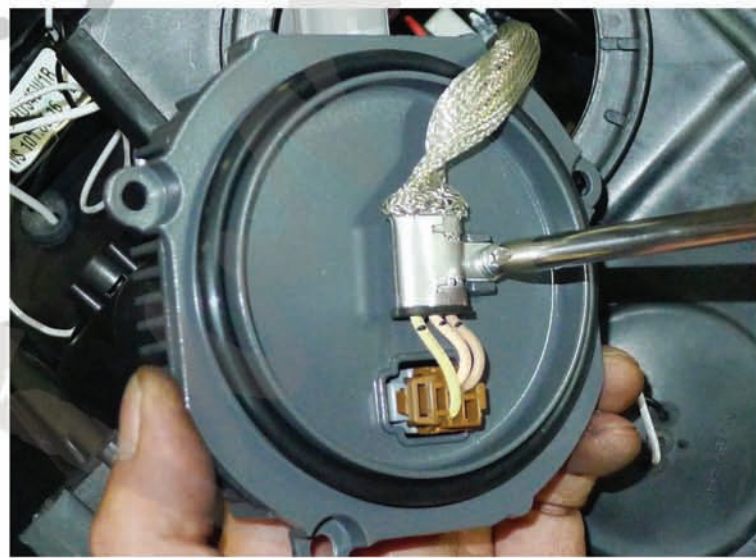
38. Secure with the phillips head screw
