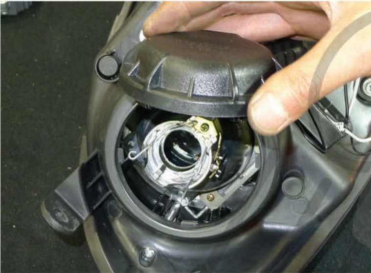
31. Remove the access hole cover from the projector headlight
