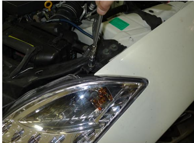
38. Tighten the 10mm bolt
