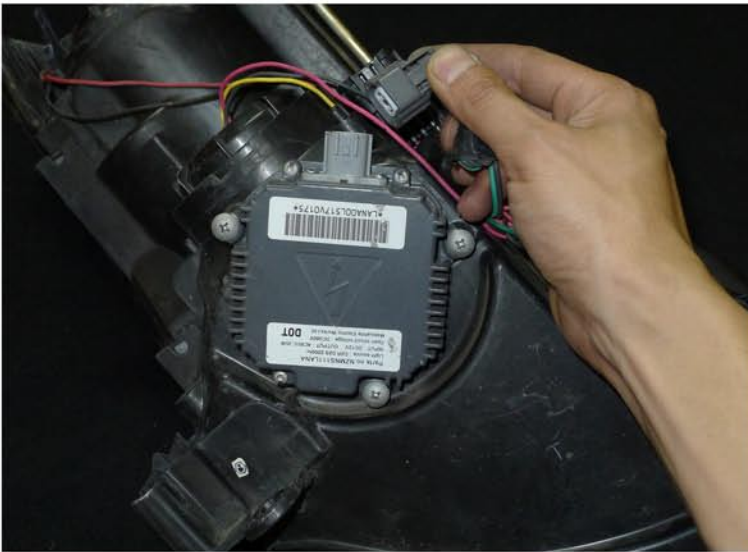
19. Disconnect the headlight harness from the ballast
