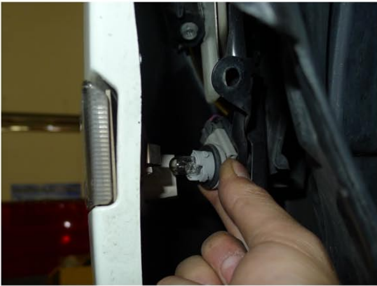
5. Disconnect the bumper light socket
