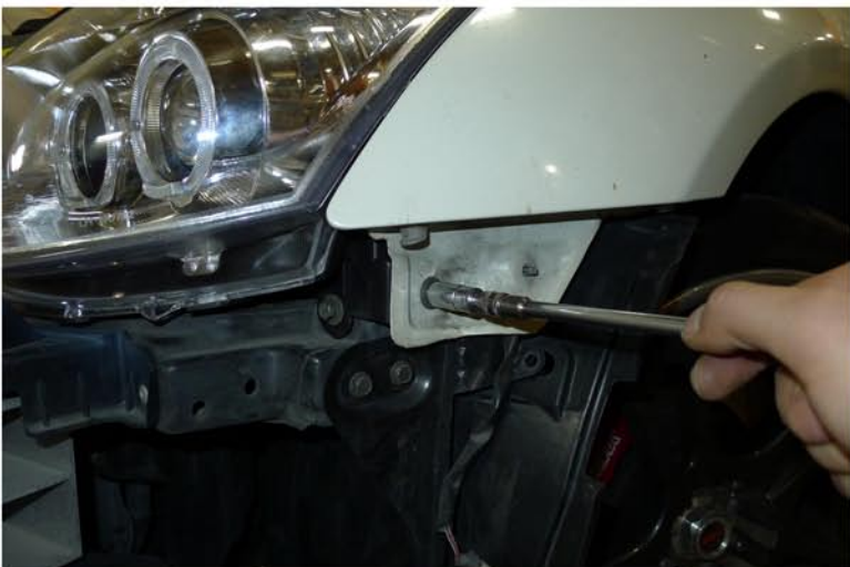
39. Tighten the 10mm bolt
