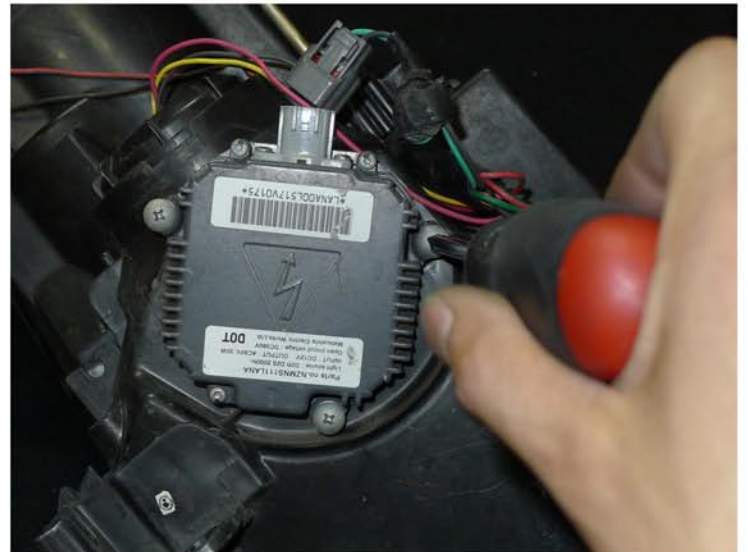
20. Remove the (3) phillips head screws
