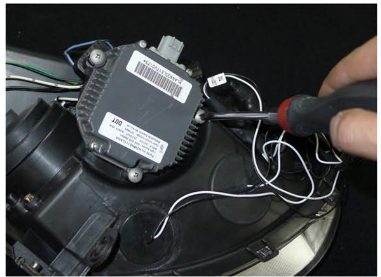
34. Tighten the (3) phillps head screws
