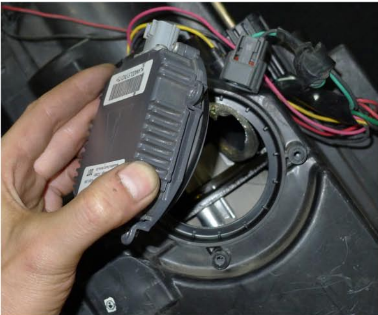
21. Remove the ballast from the stock headlight
