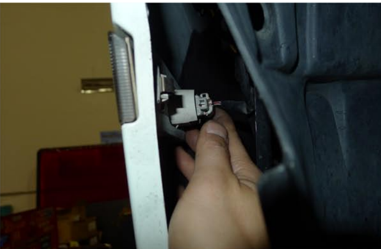
45. Replace the bumper light socket
