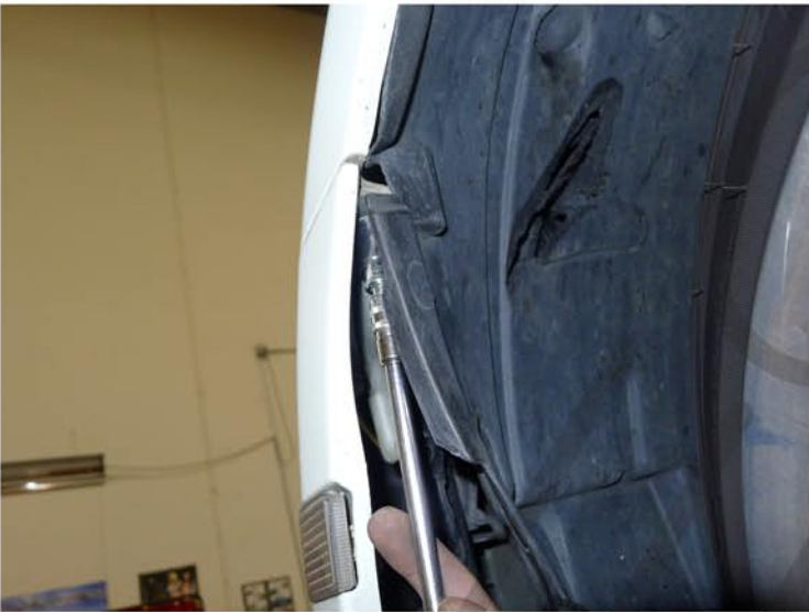
7. Remove the (2) 10mm screws
