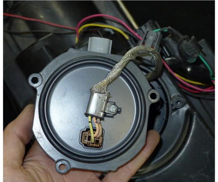
22. Back of the ballast
