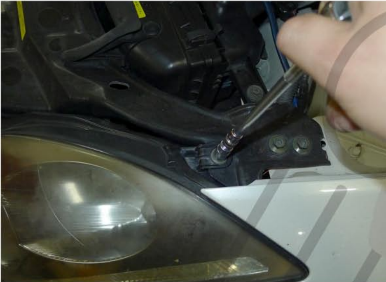
13. Remove the 10mm bolt
