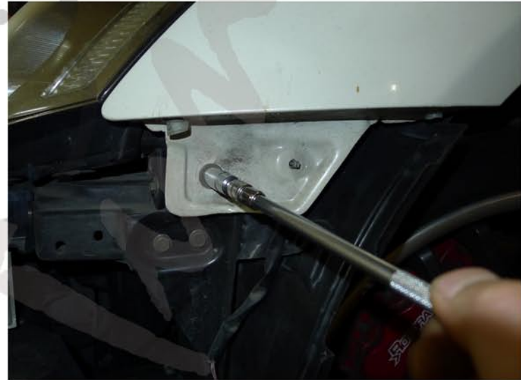
14. Remove the 10mm bolt
