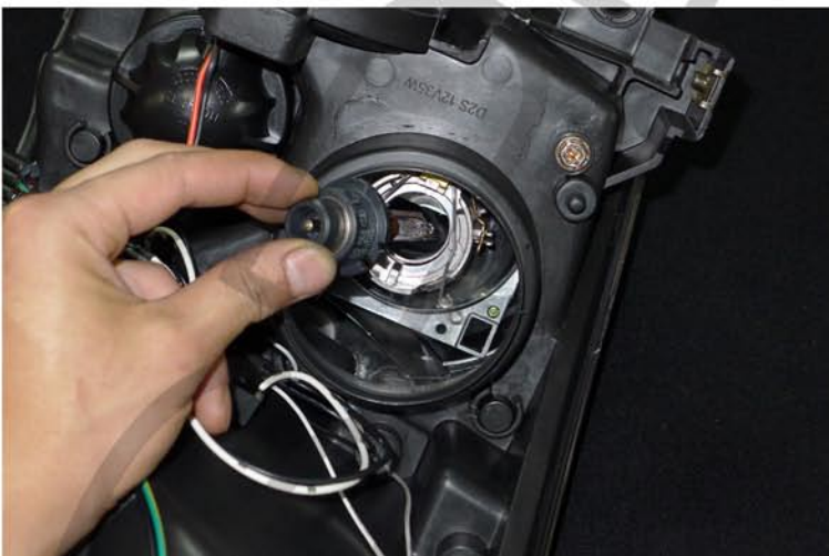
27. Remove the HID bulb from the stock headlight and place in the new headlight
