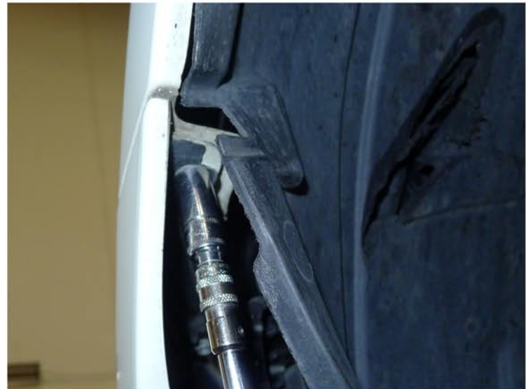
44. Tighten the (2) 10mm screws
