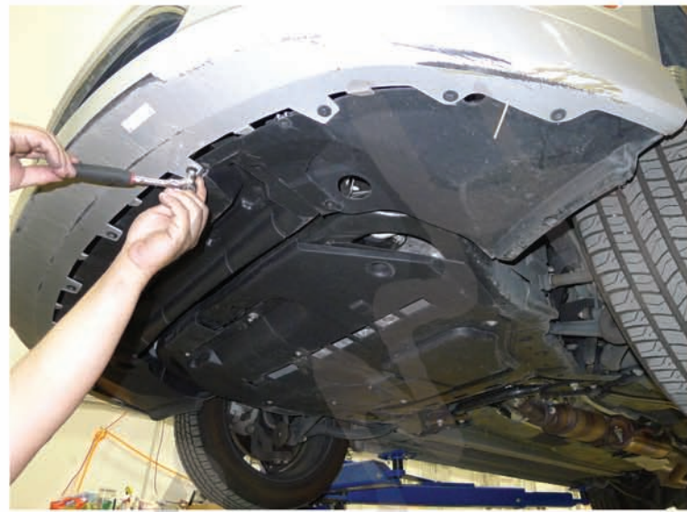
36. Replace the (14) 7mm bolts Please repeat the steps from 1 to 36 for the opposite side
