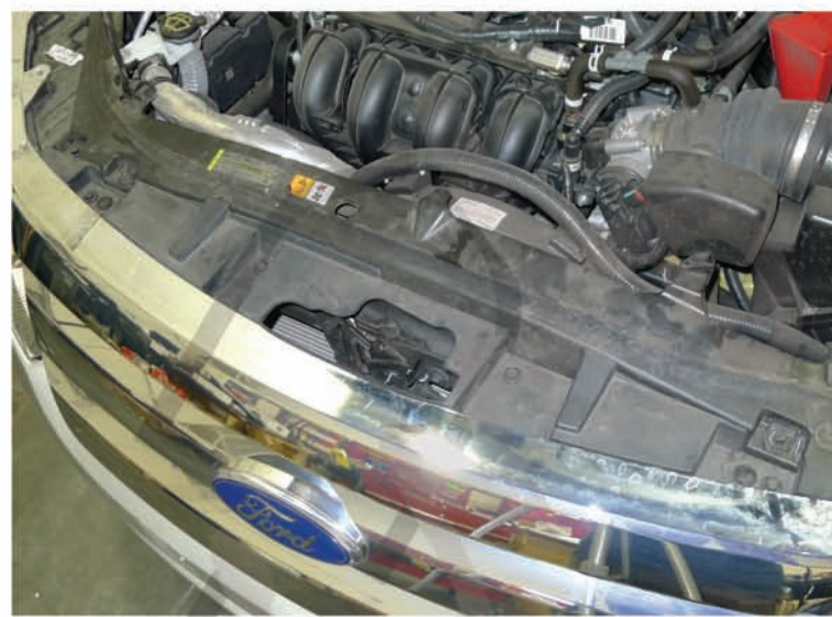
6. (2) plastic clips and (4) 10mm bolts location
