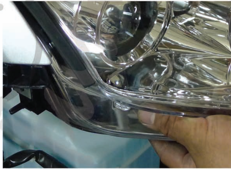
26. Place the new headlight in the stock location Please see the " L. E. D. headlights installation instructions" If your headlights don't have L.E.D. You can skip the installation instruction.
