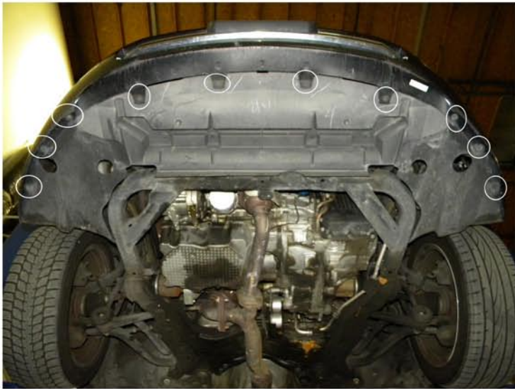
1. (10) 11mm bolts location
