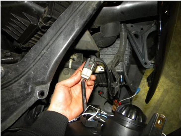
19. Plug in the headlight harness into the new headlight Please see the Halo and L.E.D installation instructions If your headlights don't have HALO or L.E.D. You can skip it
