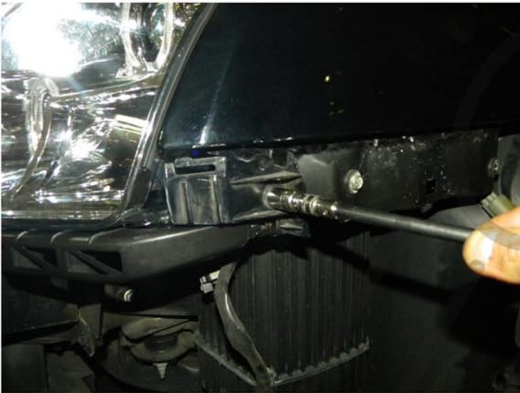
25. Tighten the 11mm bolt
