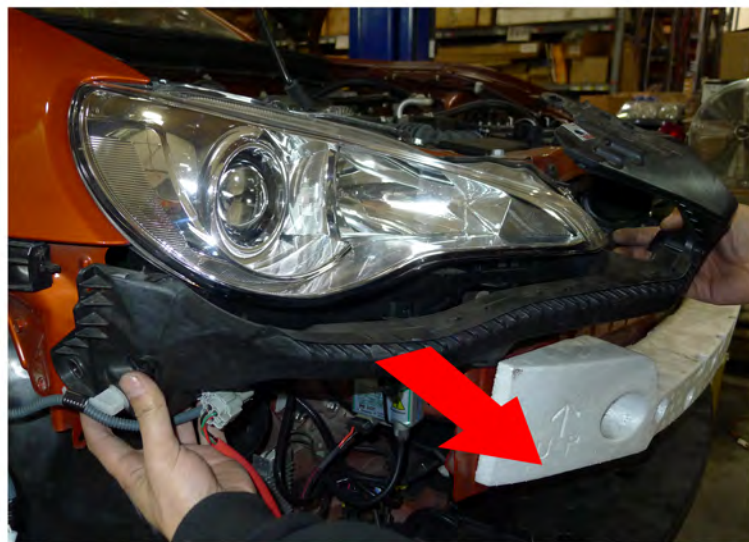
22. Remove the headlight bracket
