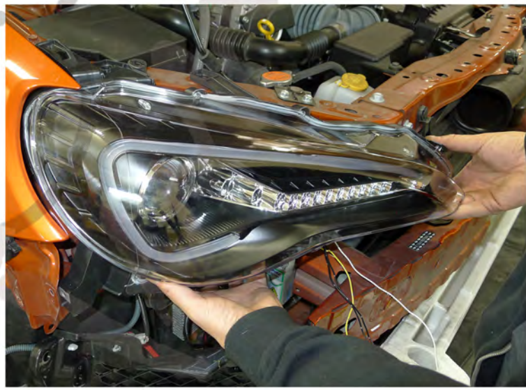
26. Place the new headlight in the stock location
