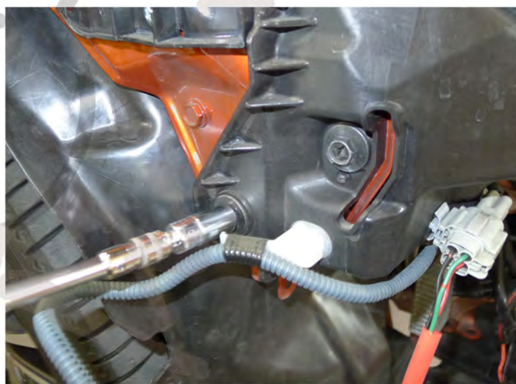
20. Remove the (2) 10mm bolts
