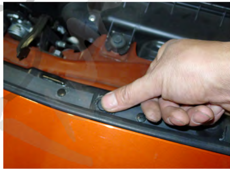
38. Replace the (2) plastic clips
