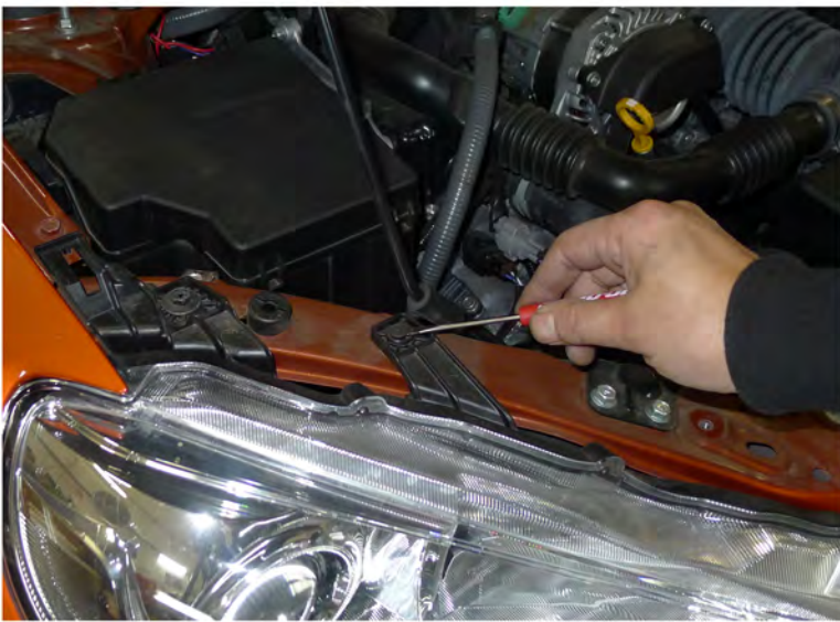
23. Remove the plastic clip
