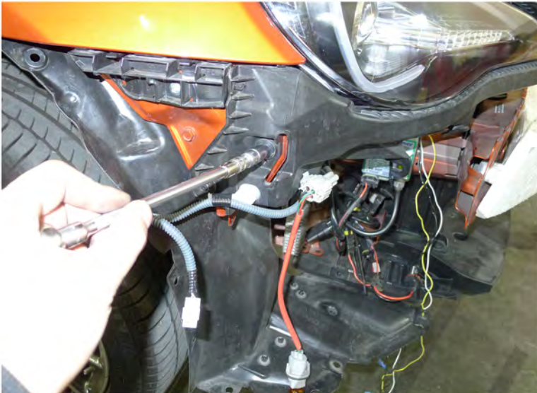
31. Tighten the (2) 10mm bolt
