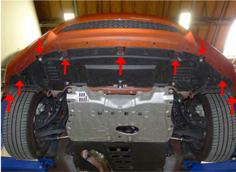
1. (6) plastic clips and (2) 10mm bolts location
