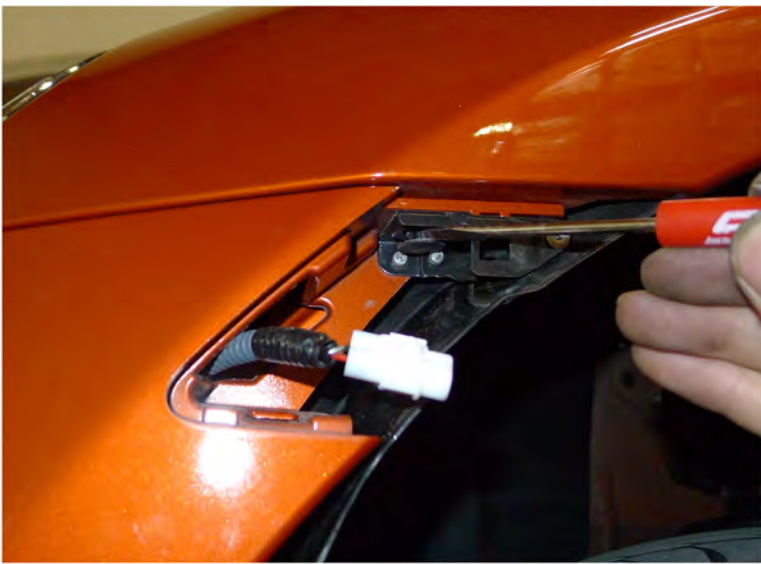
11. Remove the plastic clip
