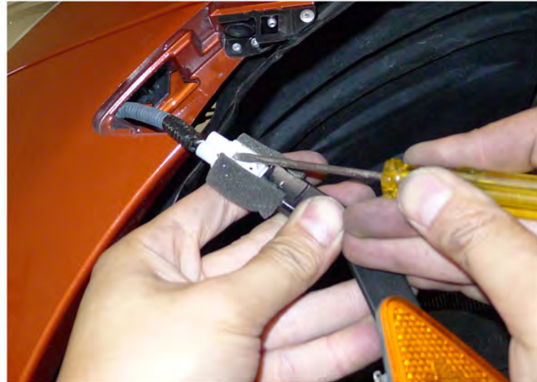
10. Disconnect the bumper light harness
