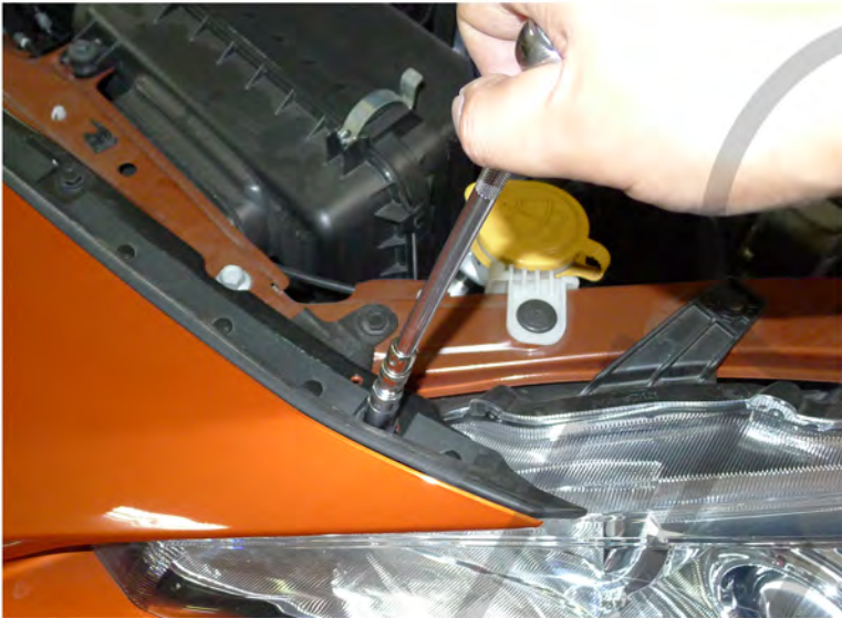
13. Remove the (5) 10mm bolts
