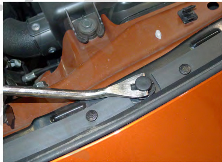
14. Remove the (2) plastic clips
