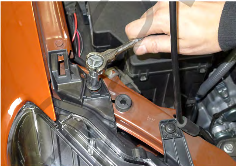
27. Tighten the 10mm bolt
