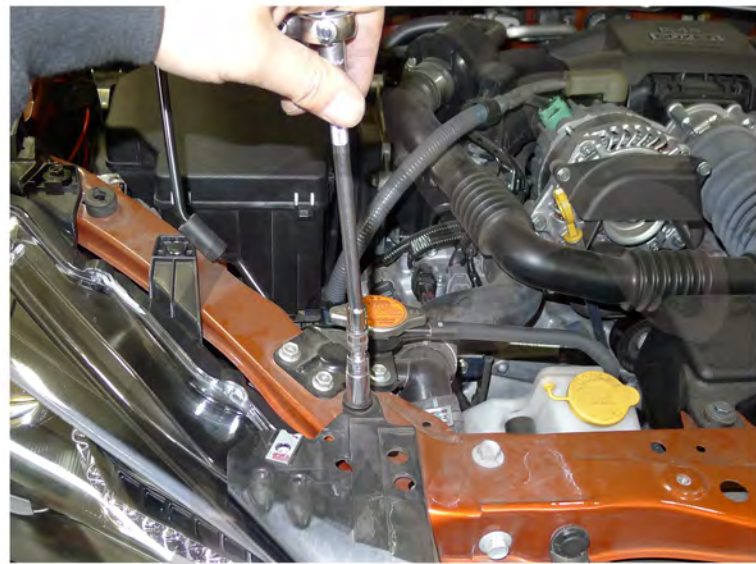
30. Tighten the 10mm bolt
