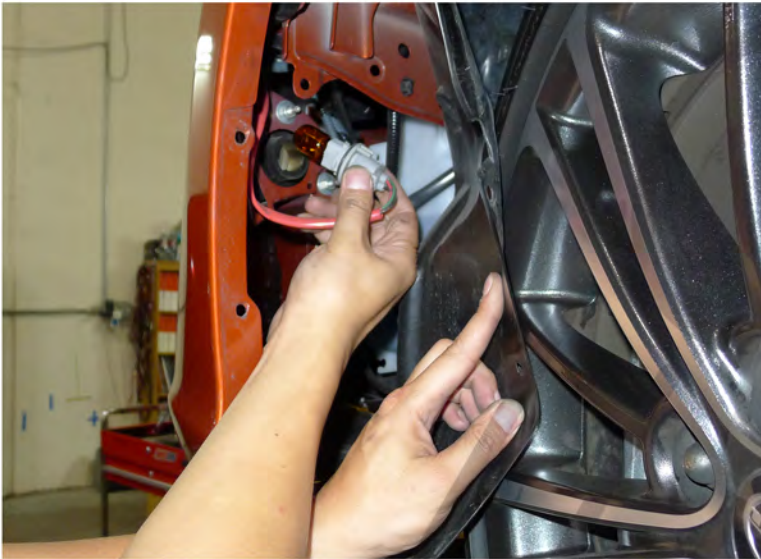
43. Replace turn signal light socket
