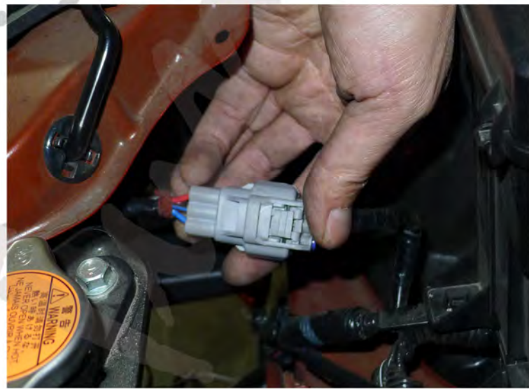
32. Connect the headlight harness
