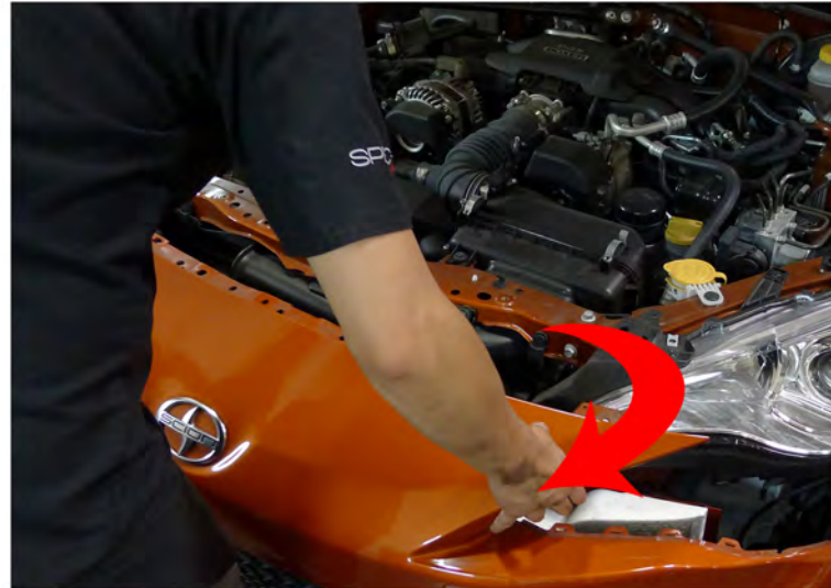
16. Remove the front bumper
