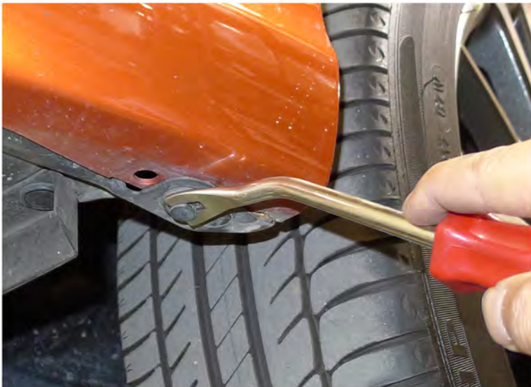
3. Remove the (6) plastic clips
