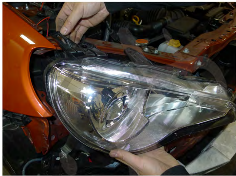
24. Remove the headlight
