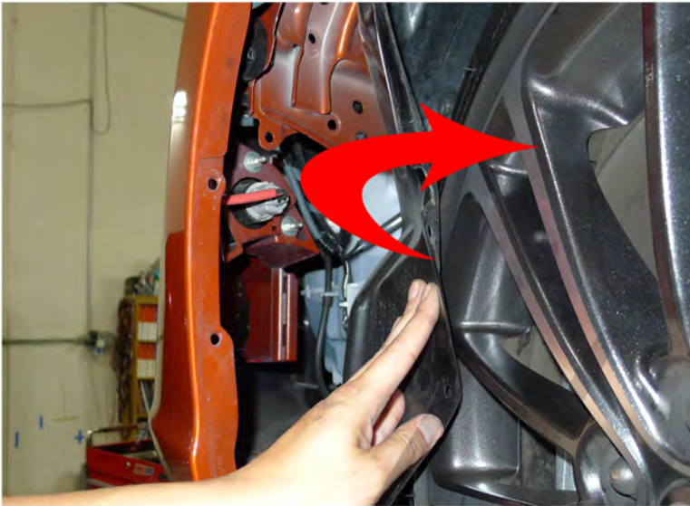
7. Pull the fender liner aside
