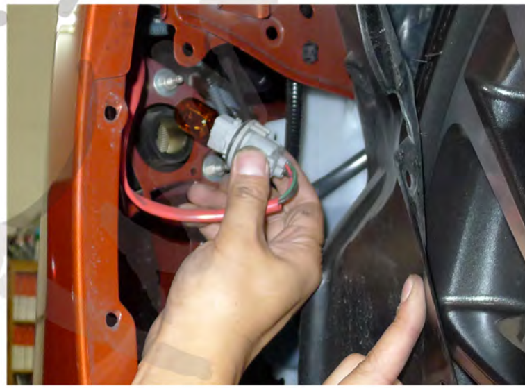
8. Remove the turn signal light socket
