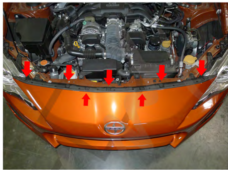
12. (5) 10mm bolts and (2) plastic clips location
