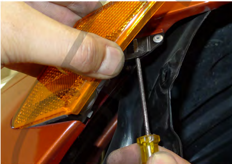
9. Remove the bumper light
