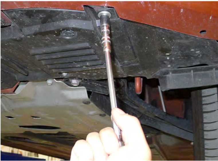
47. Tighten the (2) 10mm bolts
