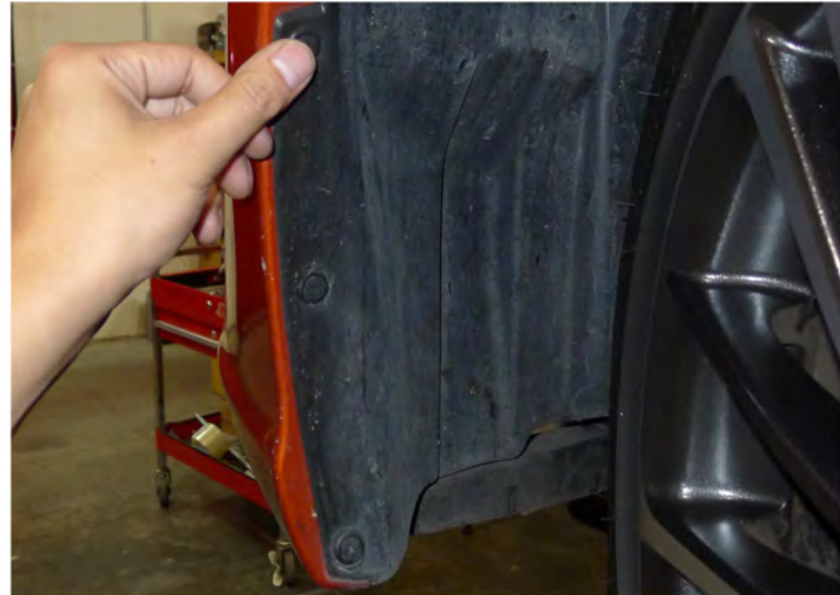
46. Replace the (3) plastic clips
