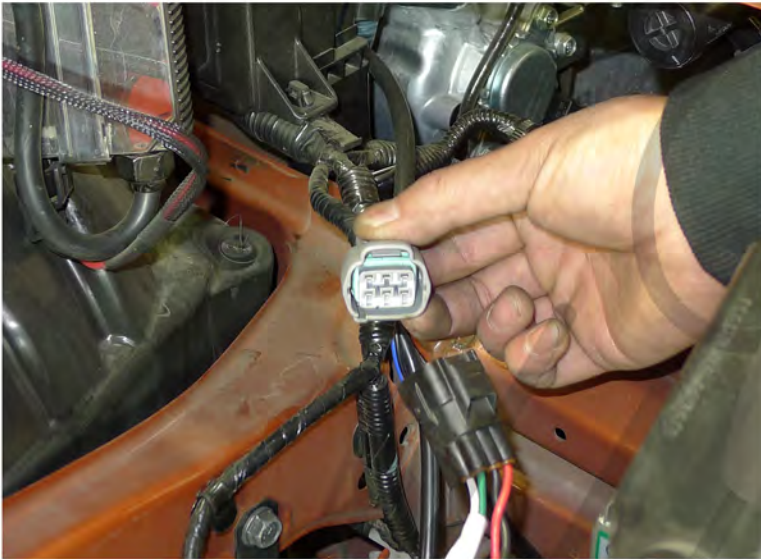
25. Disconnect the headlight harness
