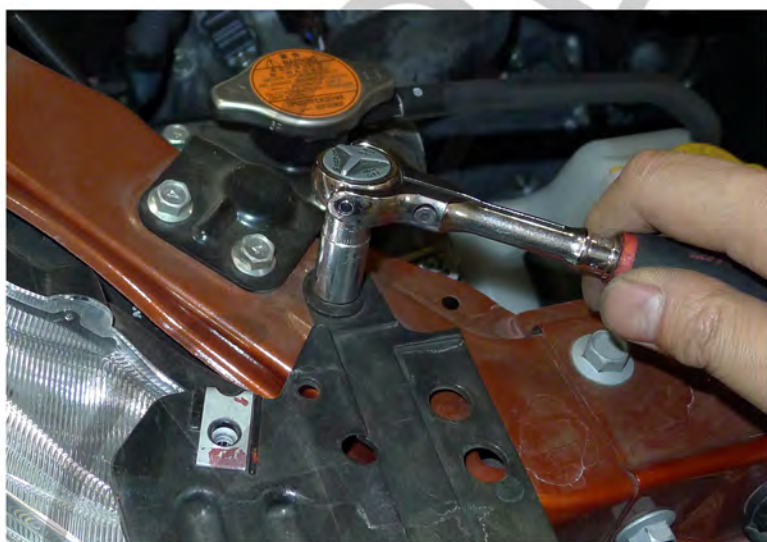
21. Remove the 10mm bolt
