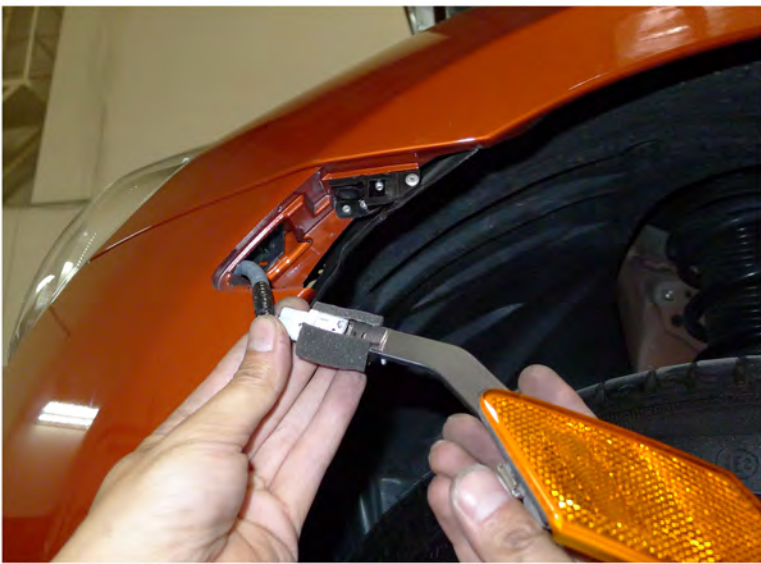
41. Connect the bumper light harness
