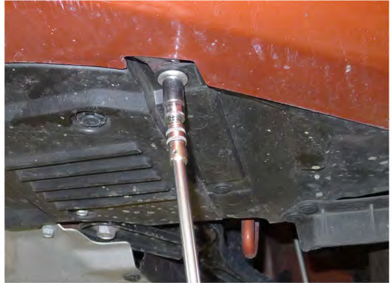
2. Remove the (2) 10mm bolts
