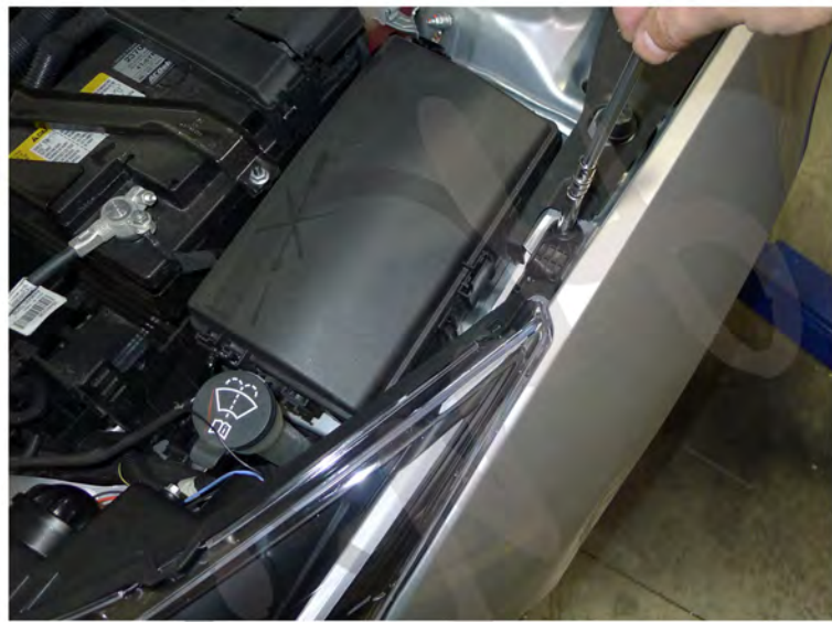
30. Tighten the 7mm bolt
