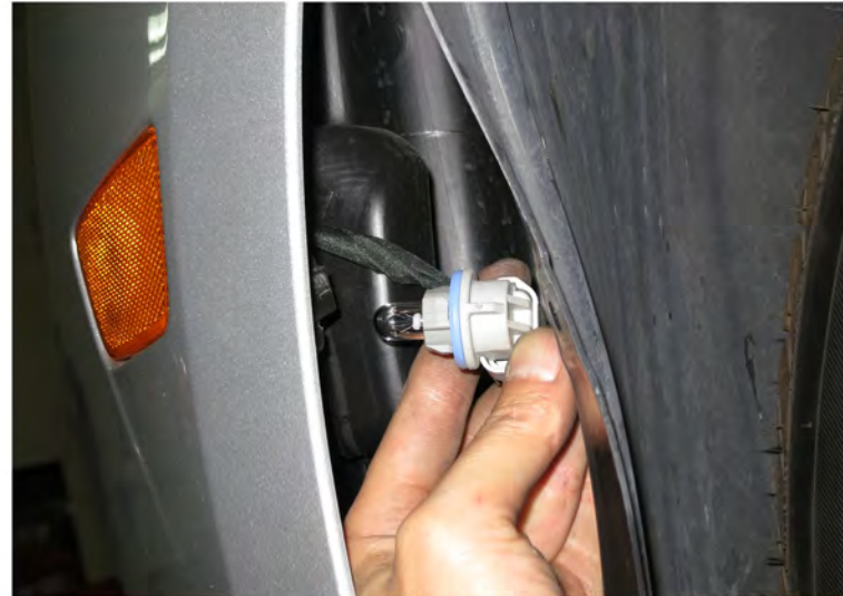
40. Replace the bumper light socket
