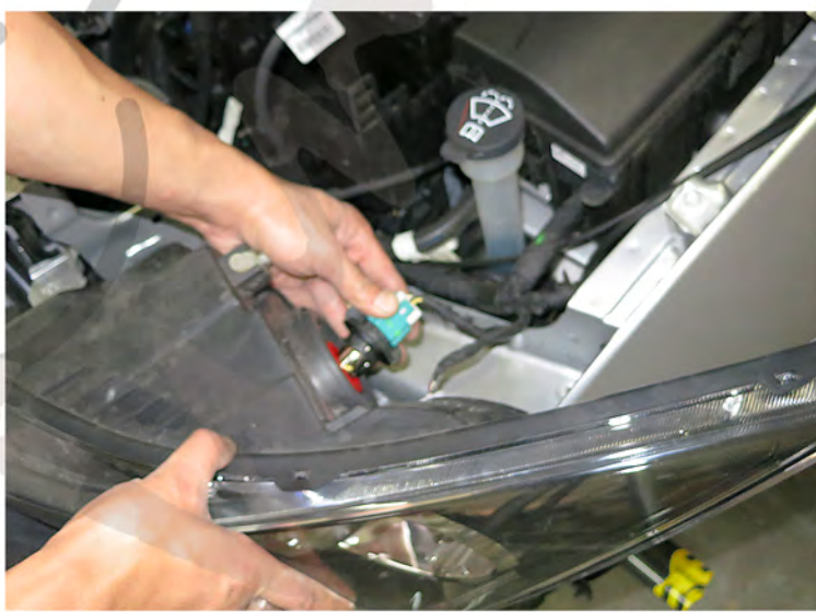
20. Remove the headlight bulb
