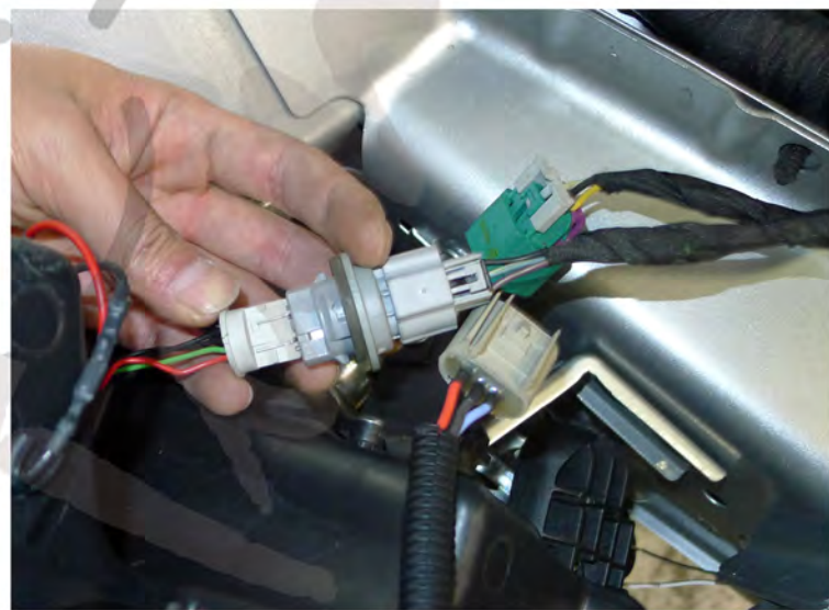
26. Connect the turn signal socket to the connector
