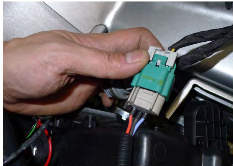
28. Connect the headlight harness to the projector headlight
