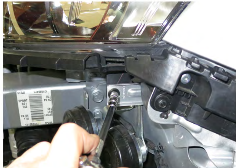
16. Remove the 7mm bolt
