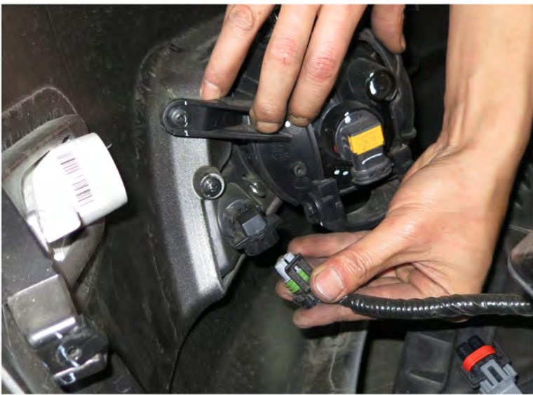
35. Connect the air temp sensor harness
