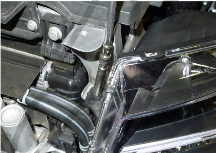
33. Tighten the 7mm bolt
