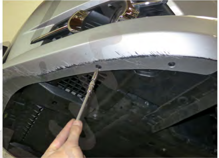
2. Remove the (8) T20 screws
