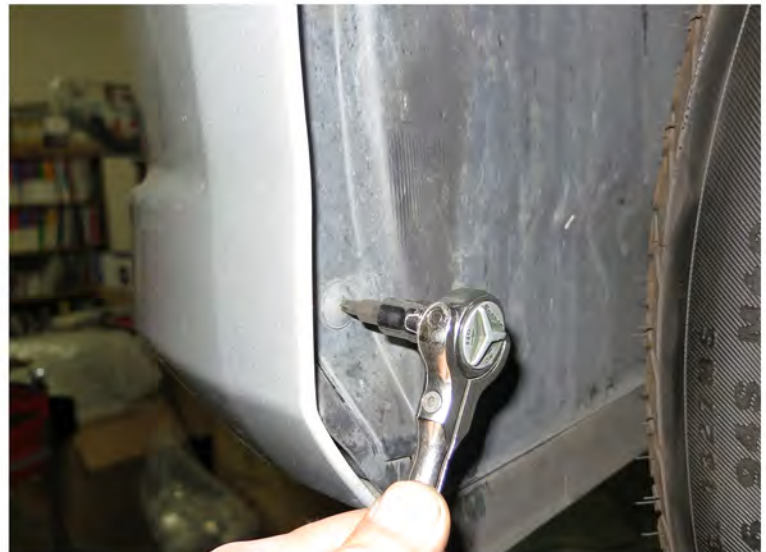
4. Remove the (3) T20 screws
