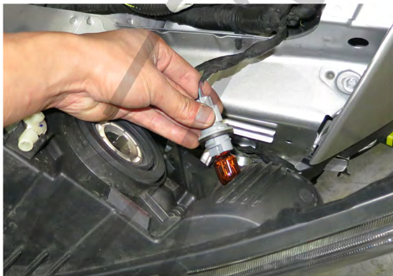
21. Remove the signal light bulb
