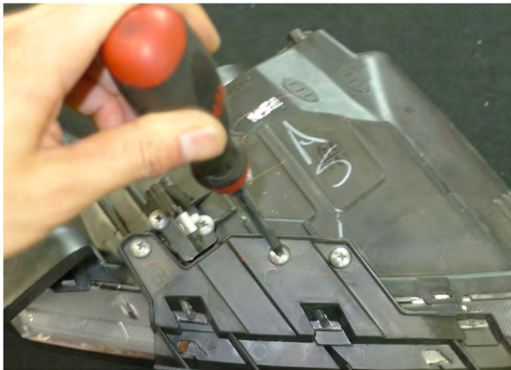
22. Remove the (5) phillips head screws
