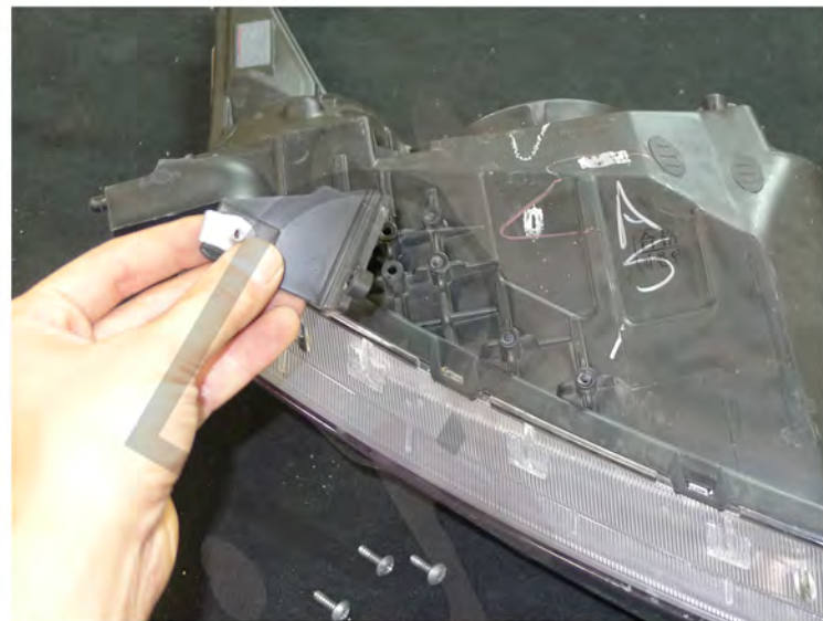
24. Remove the headlight bracket
