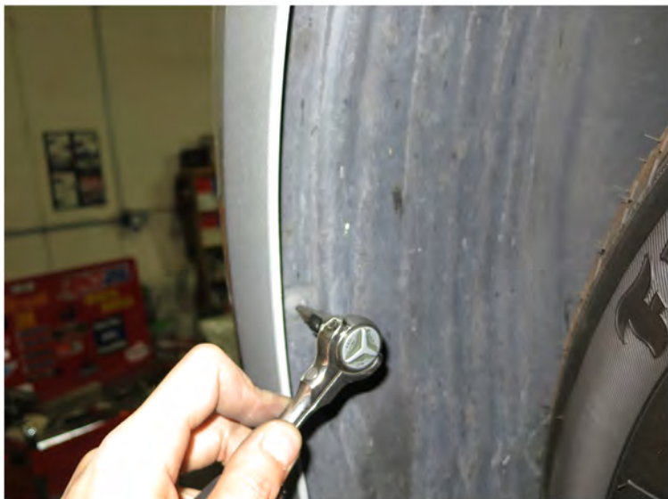
41. Tighten the (3) T30 screws
