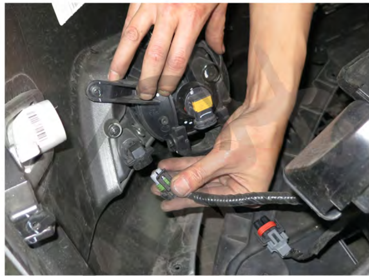
12. Disconnect the air temp sensor harness
