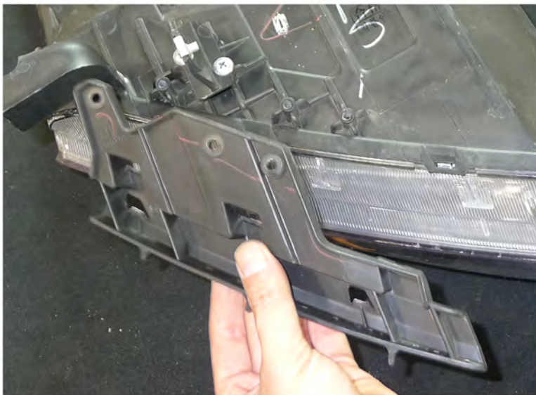
23. Remove the headlight bracket
