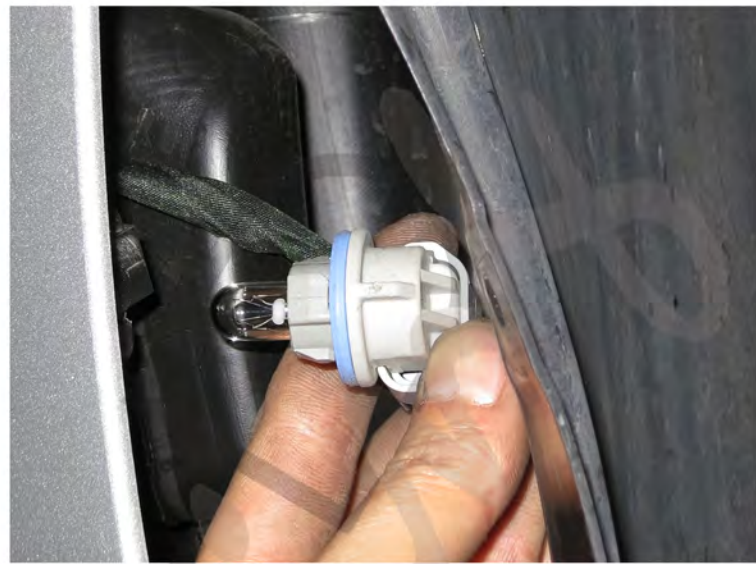
6. Remove the bumper light socket
