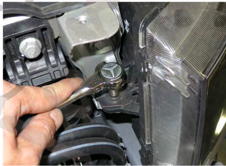
14. Remove the 7mm bolt
