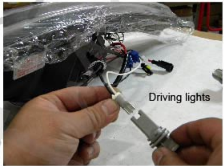
20. Install driving light socket to new headlight
