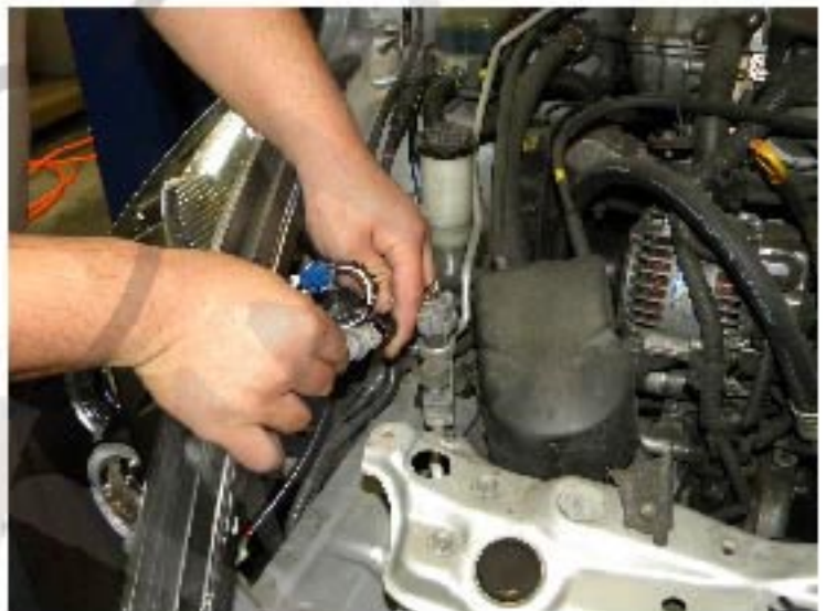
25. Connect all headlight connectors
