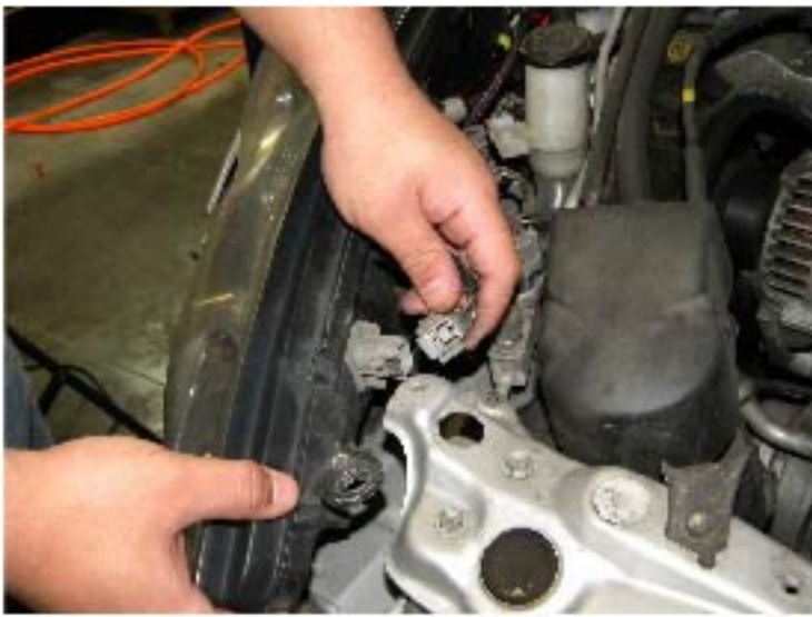
17. Disconnect all connectors from the headlight
