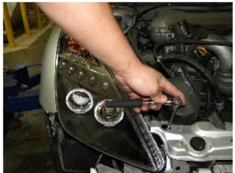
27. Install the bolt to fasten the headlight
