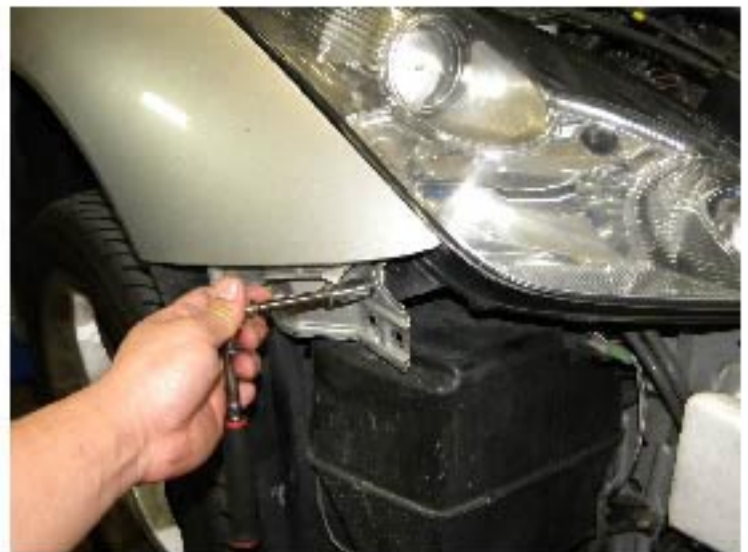
16. Remove the third bolt
