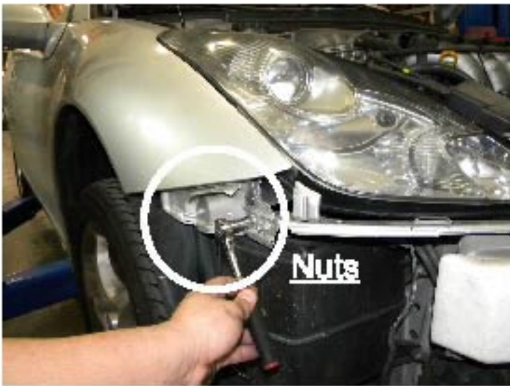
11. Remove two 10mm nuts
