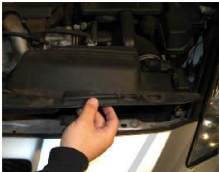
36. Install the cover and clips
