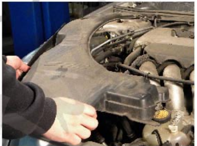
37. Install the cover and clips
