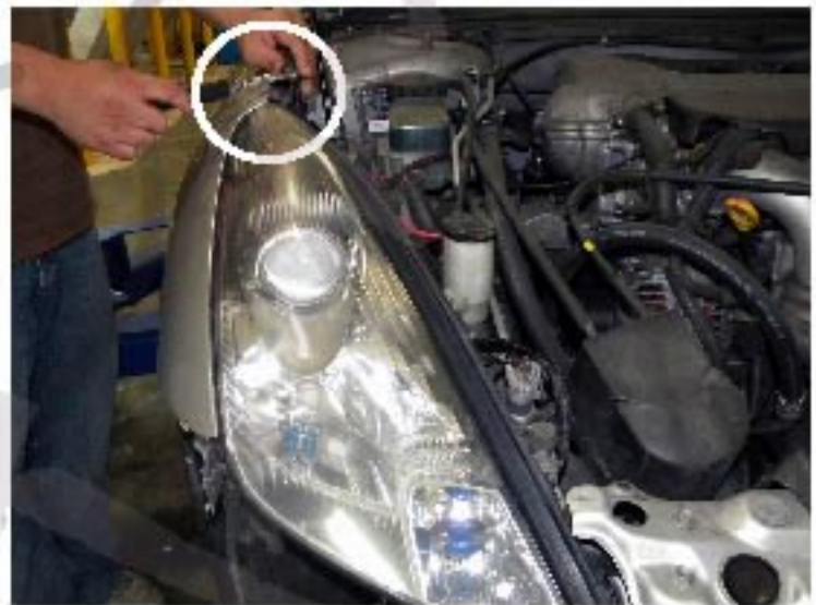
14. Remove three headlight bolts
