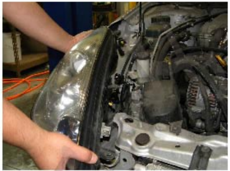
18. Remove the headlight
