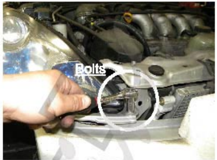
12. Remove one 10mm bolt
