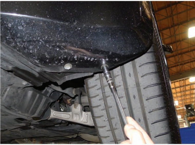
41. Tighten (10) 10mm bolts Please repeat the steps from 1 to 41 for the opposite side
