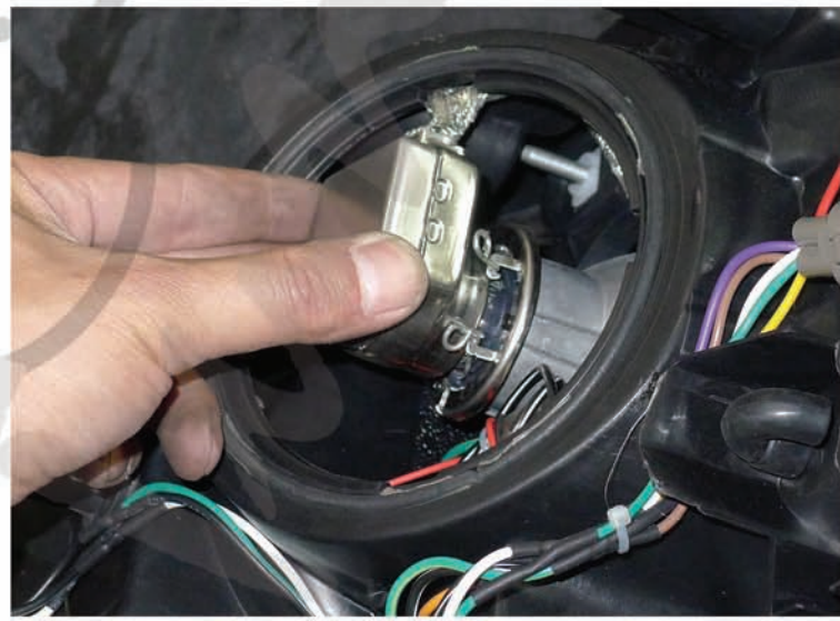
32. Install the HID socket onto HID bulb
