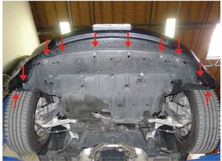
2. (10) 10mm bolts location
