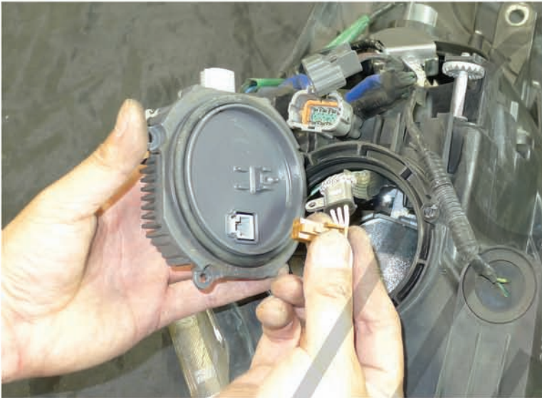
25. Disconnect the HID light socket harness from the ballast
