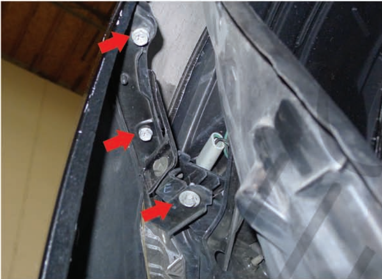
7. (3) 10mm bolts location
