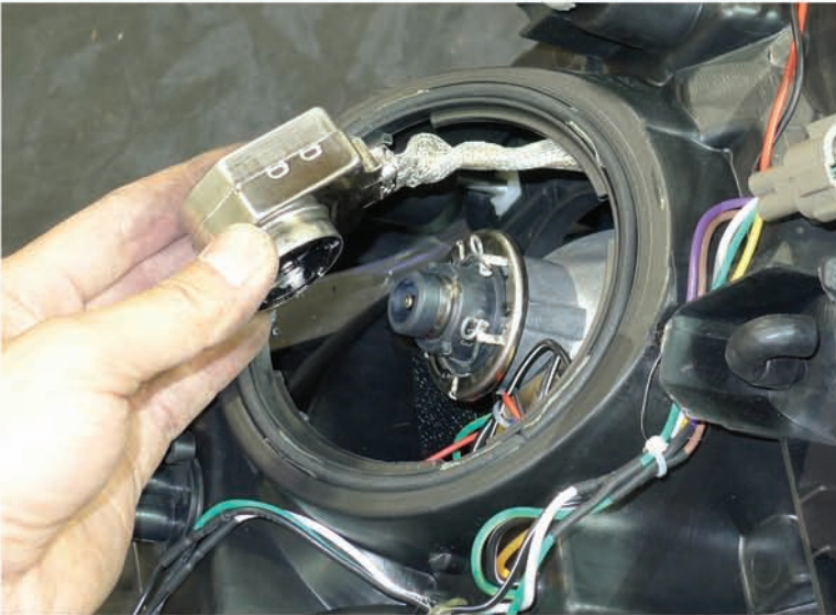
31. Run the HID bulb socket harness through the new headlight housing
