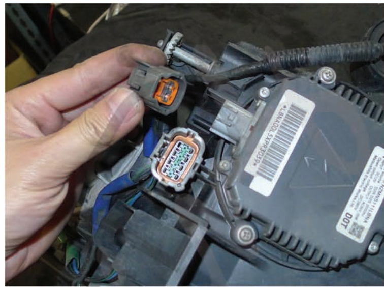
18. Disconnect the harness from the ballast
