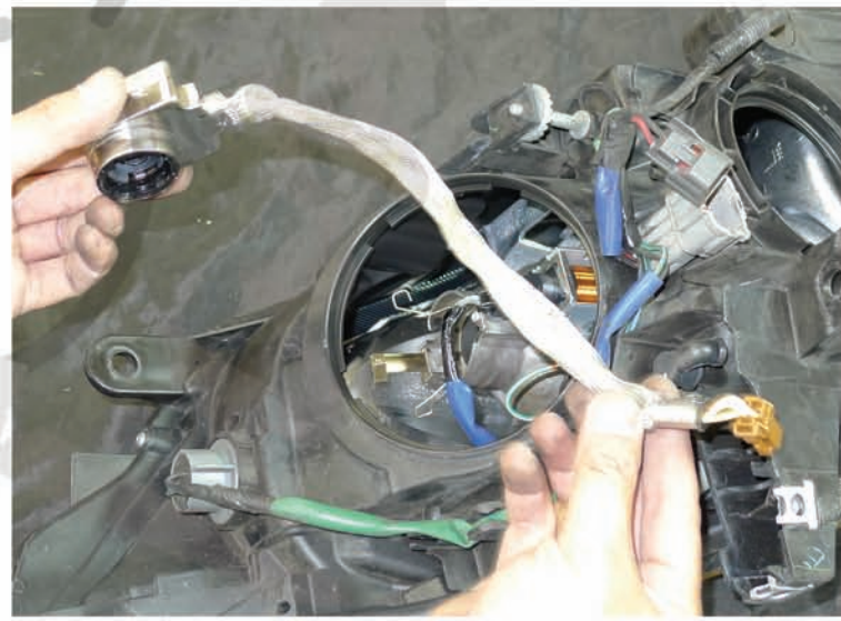
26. Remove the HID light socket harness from the factory housing
