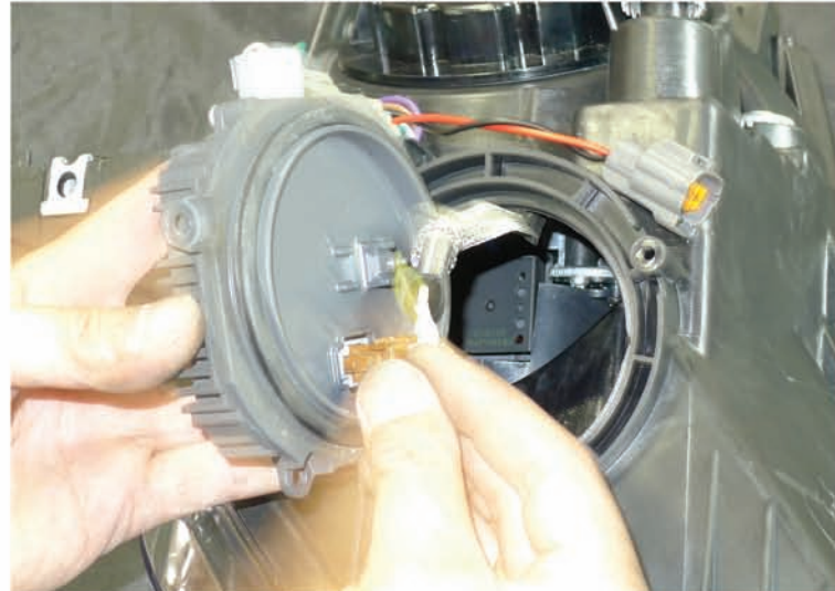
34. Connect the HID socket harness to the ballast
