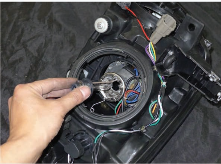
29. Install the HID bulb into the new projector headlight
