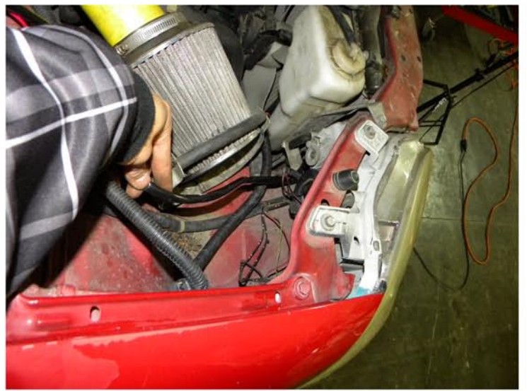
22. Run the fog light harness through the bulkhead along the stock harness
