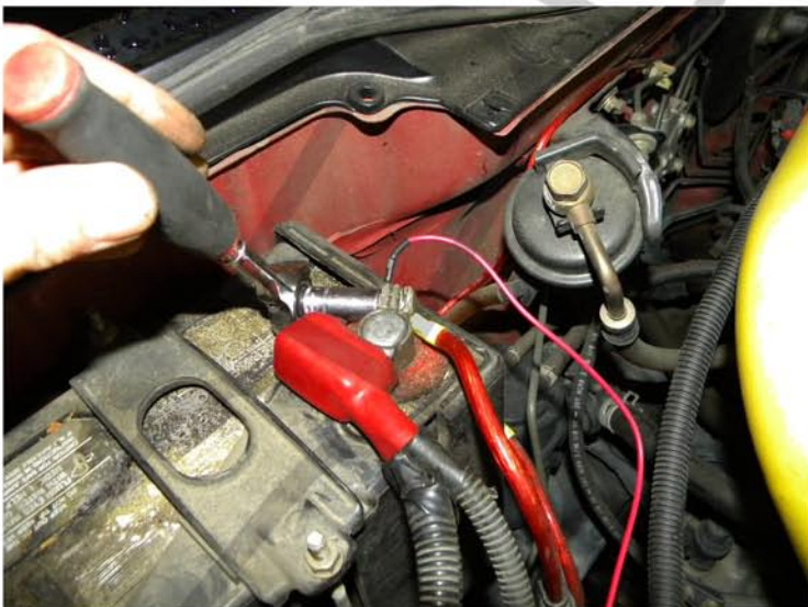
21. Connect the red wire from the fog light harness and tighten the 10mm bolt
