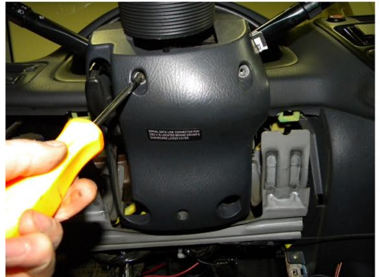
44. Remove the (3) phillips head screws from the steering column cover
