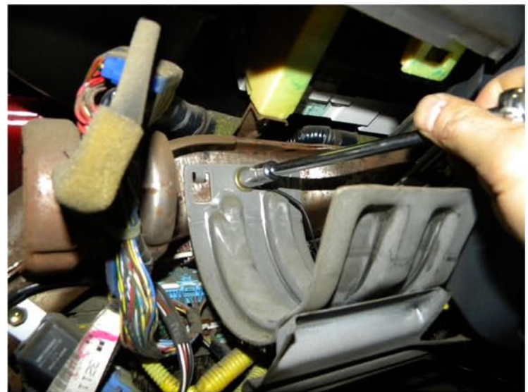
42. Connect the switch harness ground wire to the 10mm bolt and tighten the 10mm bolt
