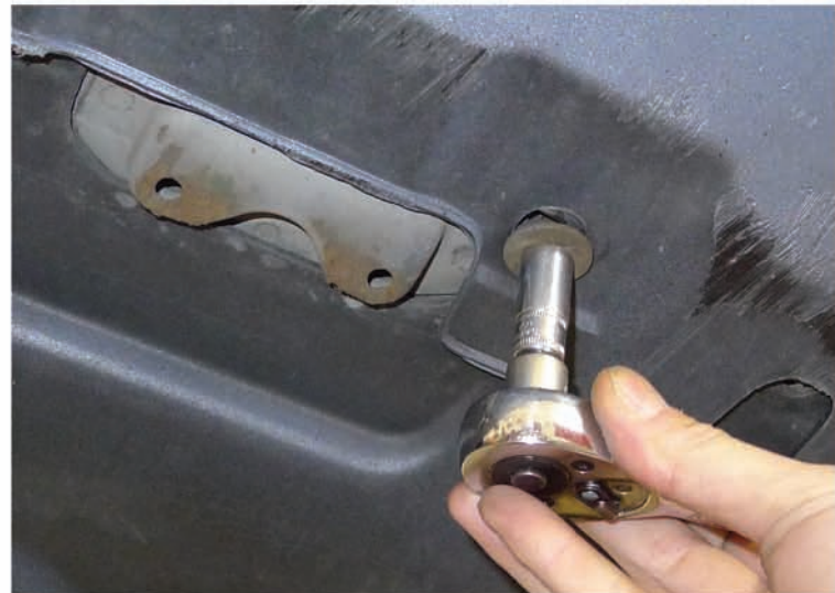
28. Tighten the (2) 10mm bolts
