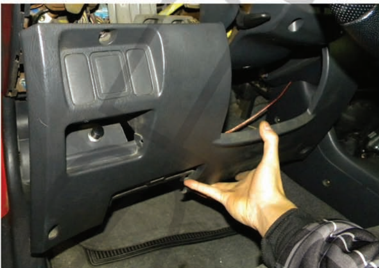
33. Remove the lower dash panel
