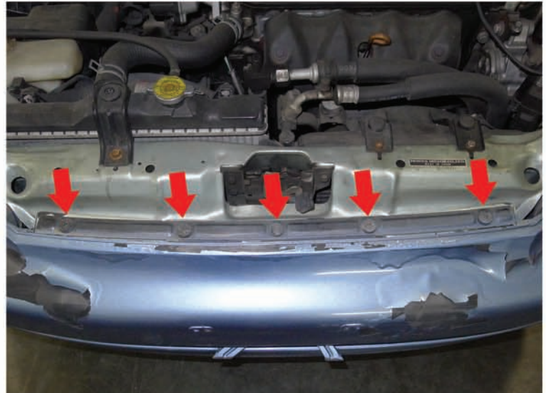
4. (5) phillips head screws location
