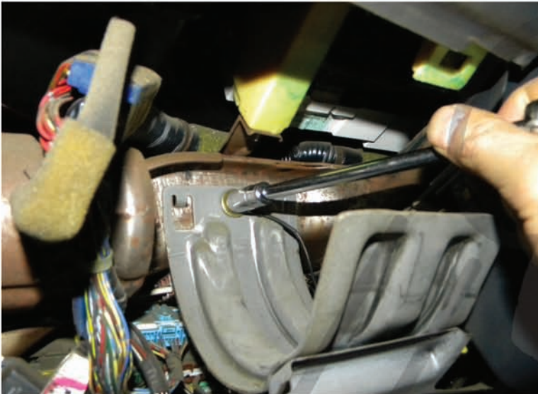
37. Connect the switch harness ground wire to the 10mm bolt and tighten the 10mm bolt
