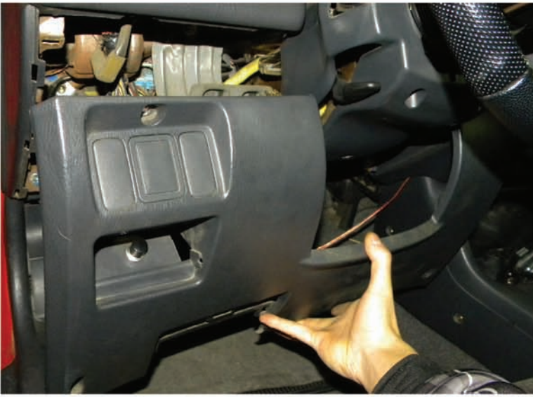
47. Replace the lower dash panel
