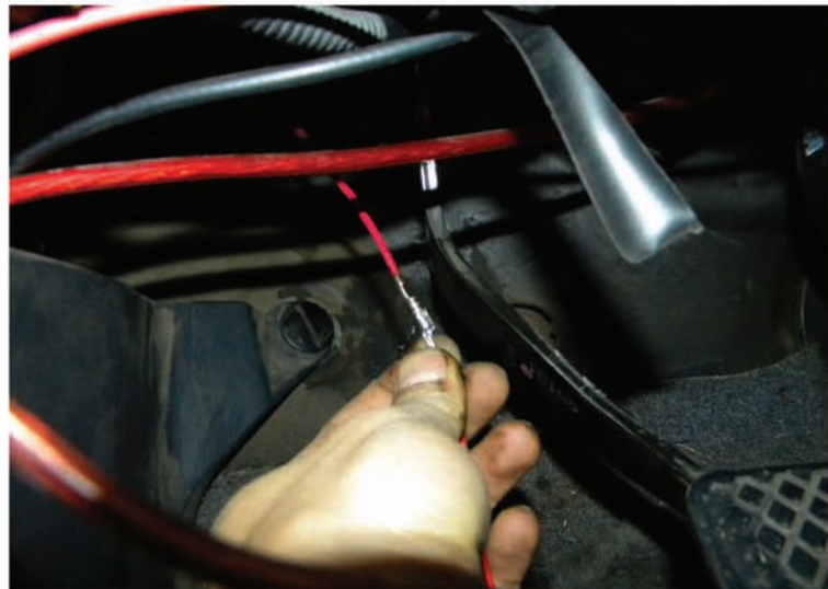
34. Connect the switch harness
