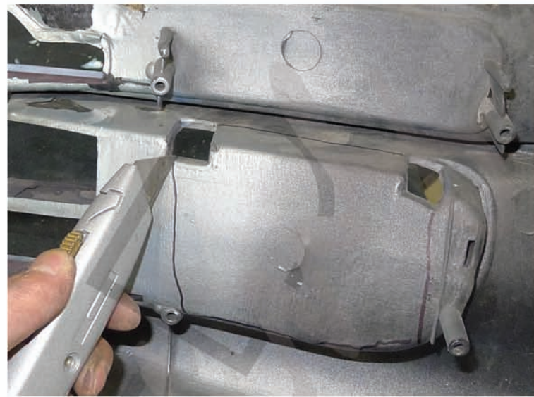
18. Cut the area previously marked
