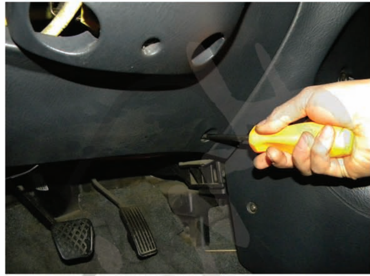
48. Tighten the (3) philips head screws Please repeat the steps from 1 to 48 for the opposite side
