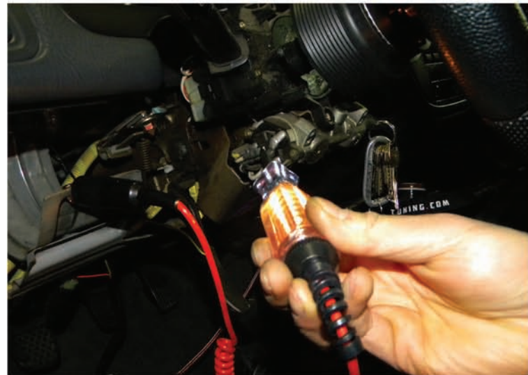
40. Find the ACC power wire with the test light
