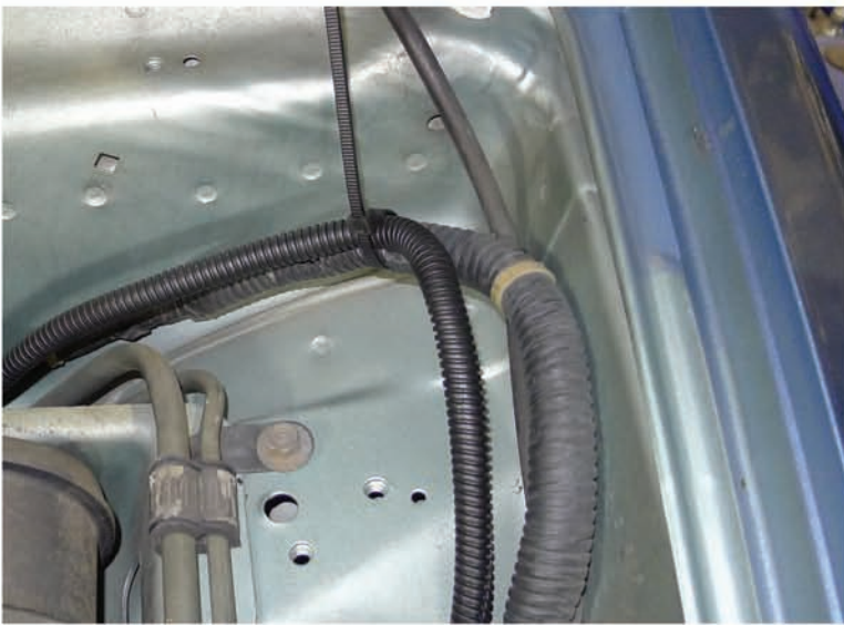
29. Secure the fog light harness to the factory harness with the zip ties
