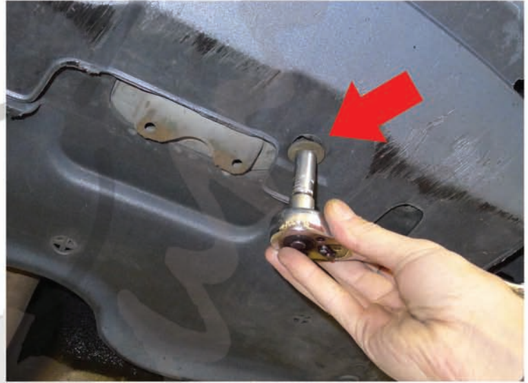
2. Remove the (2) 10mm bolts
