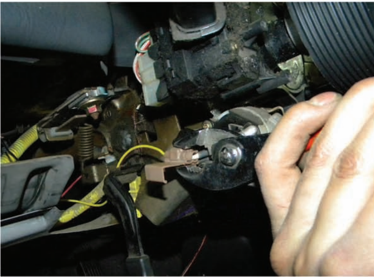
41. Connect the wire on switch harness to the ACC power wire using the quick connector
