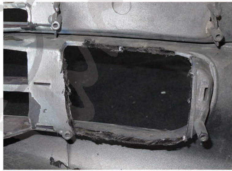
20. Cut the portion removed
