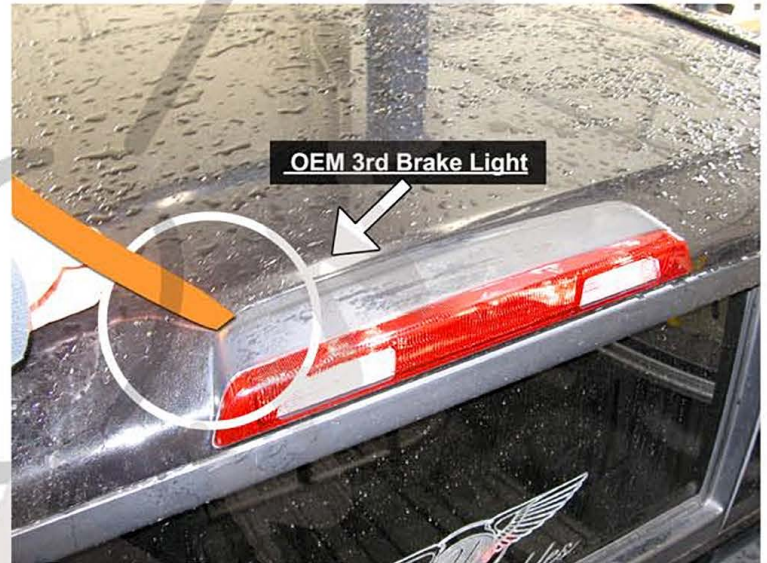
2. Carefully loosen the OEM 3rd brake light from the roof of the vehicle
