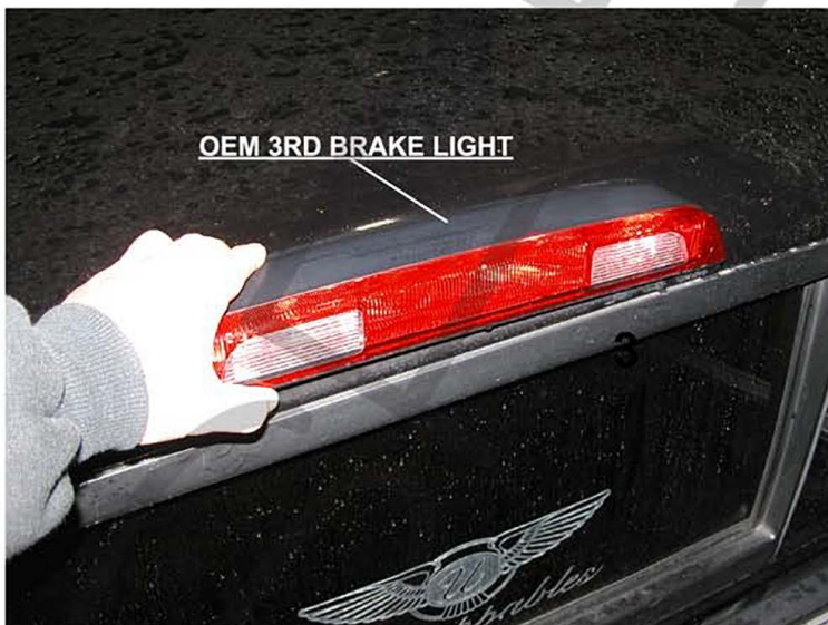
3. Pull out the OEM 3rd brake light
