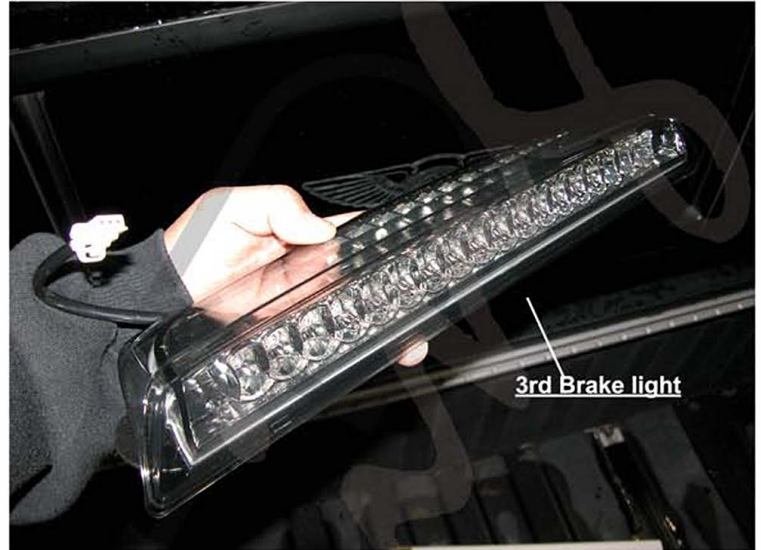
6. Bring out the new 3rd brake light
