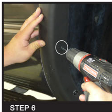
Drill (4) 3mm pilot hole on the fender
