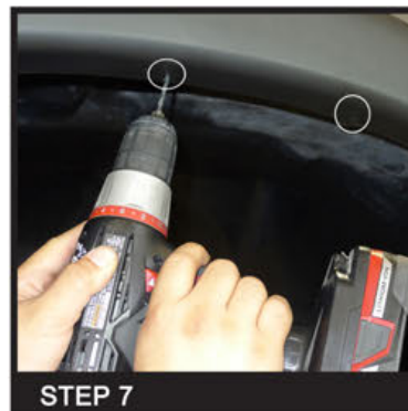
Drill (4) 3mm pilot hole on the fender
