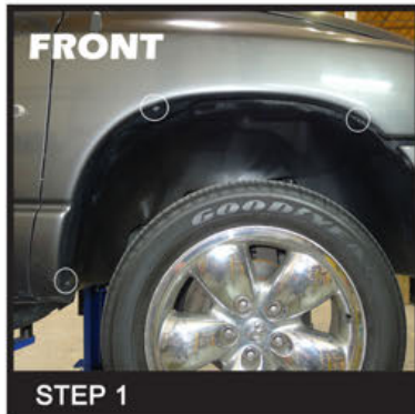
Remove (3) 8mm front wheel well liner bolts
