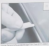
seat edge trim against face by inserting straight end between edge frim and flare at one end, Next, slide around entire edge to the other end
