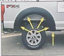
Hold flare to vehicle and mark five flare hole locations. with a grease pencil
