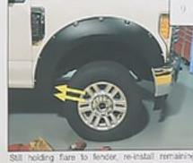
Still holding flare to fender, re-install remaining factory screws removed in Step 4 using 7mm socket and wrench. Tighten all screws.
