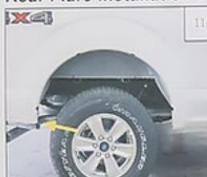
Remove factory fastener from read of wheel well. Thoroughly clean the vehicle sheet metal and inner flange prior to installation.
