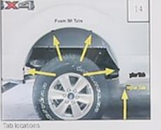
tab installed at the lower front of the rear wheel well.
