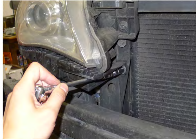
16. Remove the (2) 10mm bolts
