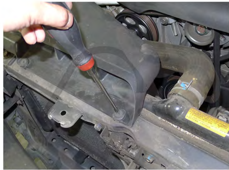
12. Remove the (2) plastic clips
