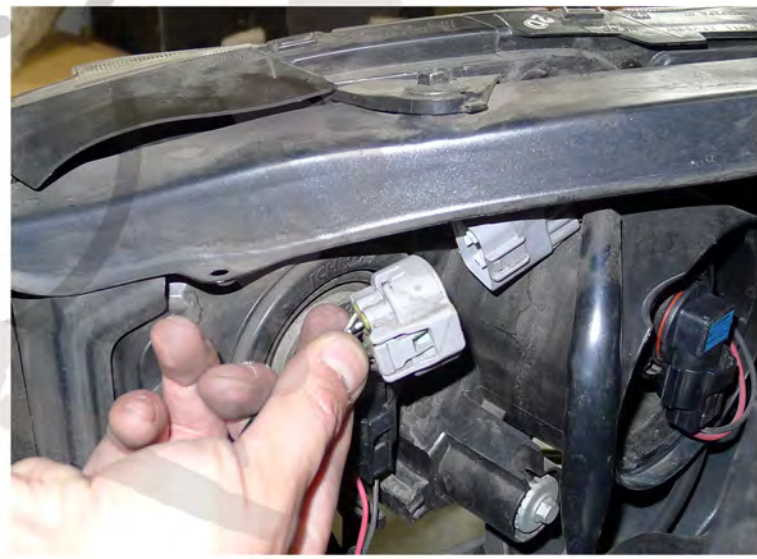
14. Disconnect the headlight harness
