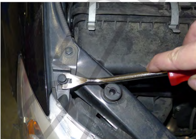
21. Remove the plastic clip
