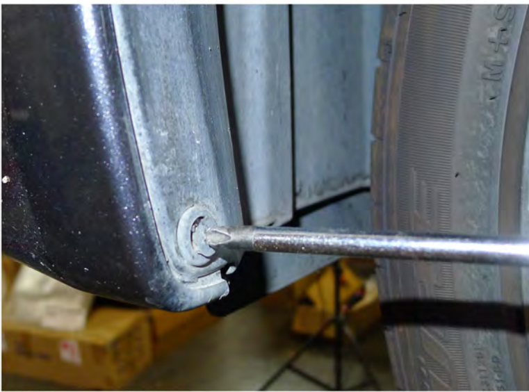
5. Remove the (3) plastic clips
