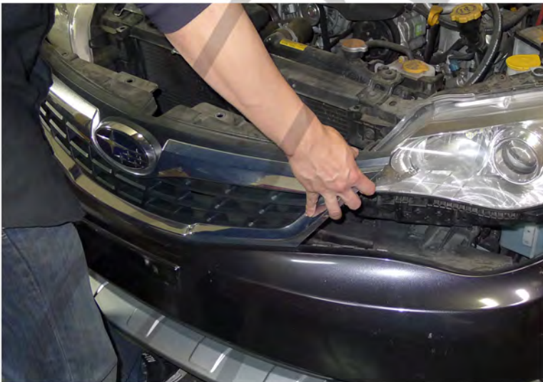
9. Remove the front bumper
