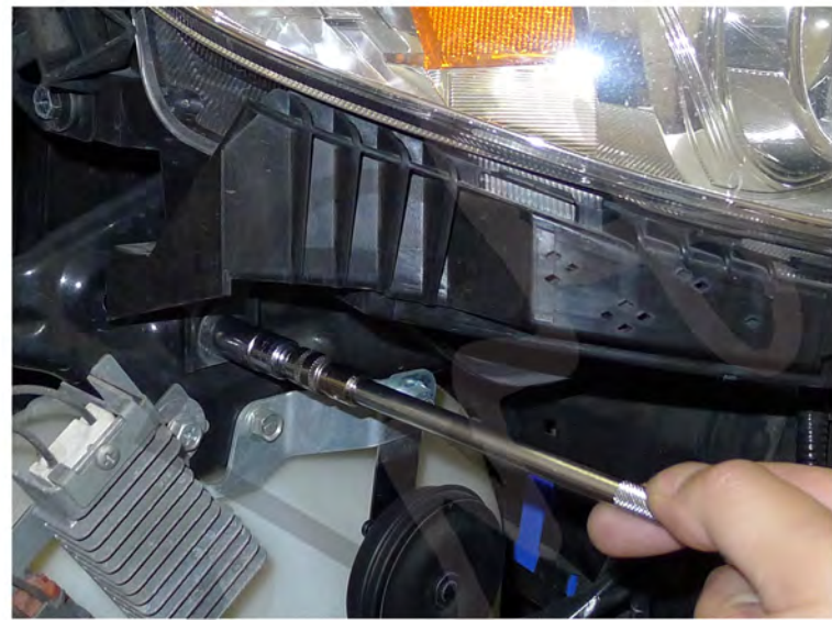
18. Remove the (2) 10mm bolts
