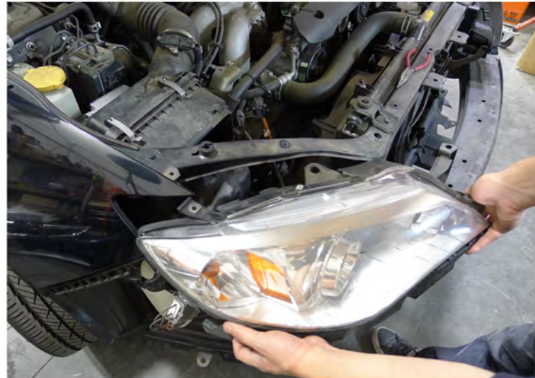
28. Remove the factor headlight
