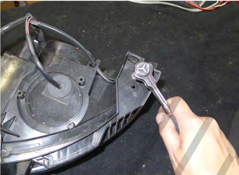
25. Remove the (3) 10mm bolts
