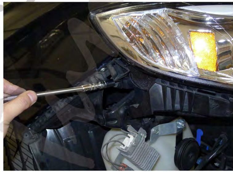
32. Tighten the (2) 10mm bolts
