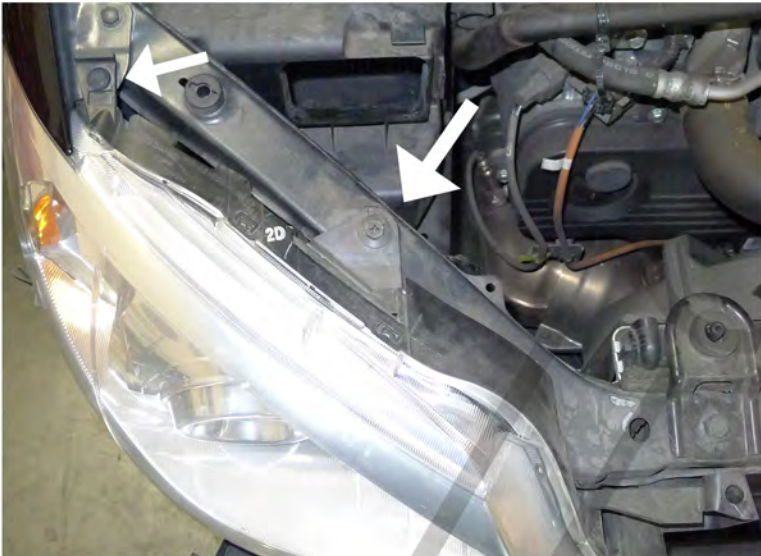
19. Remove the plastic clip
