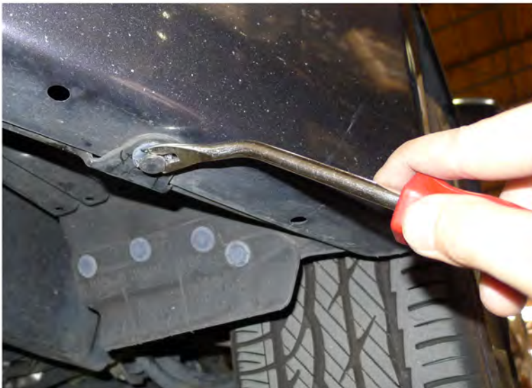
3. Remove the (6) plastic clips
