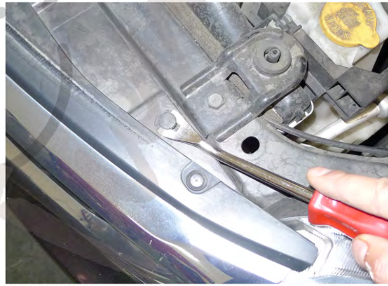
8. Remove the (4) plastic clips
