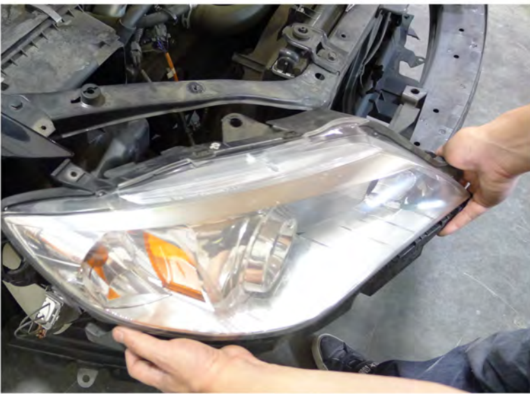
23. Remove the factor headlight
