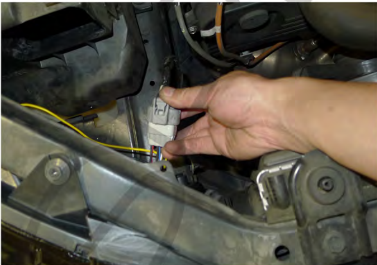
33. Connect the headlight harness to the new projector headlight Please see the " L. E. D. head lights installation instructions" If your head lights don't have L.E.D. You can skip the installation instruction.
