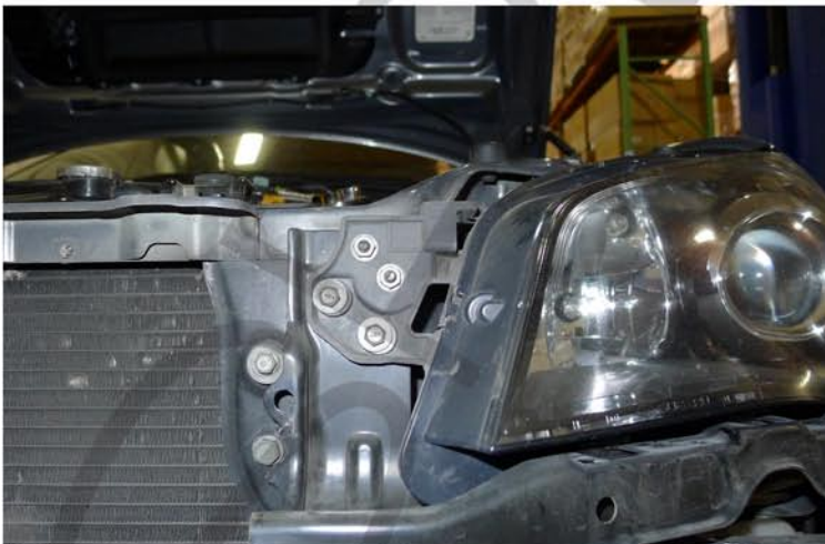
15. (2) 10mm nut and the (2) 10mm bolts location
