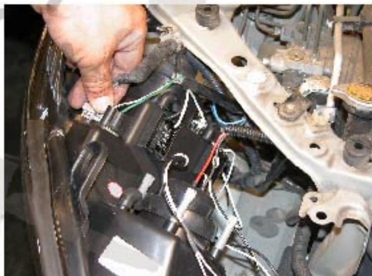
14. Connect all headlight connectors please see the "Halo and L.E.D. installation instructions" If your headlights don't have HALO or L.E.D. You can skip the installation instructions.
