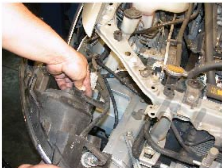
13. Disconnect all connectors from the headlight, then remove the headlight
