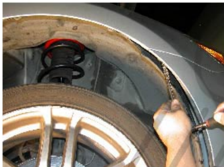
19. Install one 10mm bolt at side of the bumper ( Both sides)
