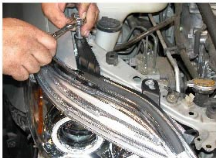
16. Install two 10mm headlight bolts at top of the headlight
