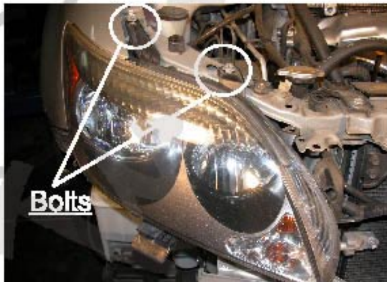
8. Two 10mm headlight bolts at top of the headlight
