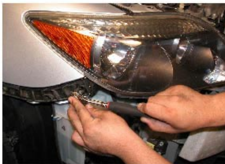
10. Remove one 10mm headlight bolt at side of the headlight
