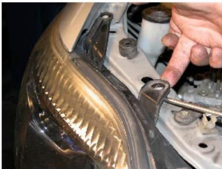
11. Pull the bracket up to unlock the headlight
