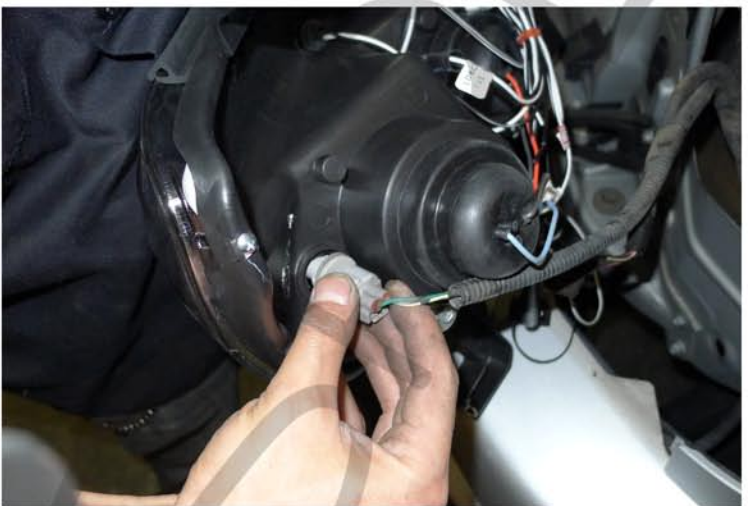
21. Connect the light sockets to the new headlight Please see the Halo and L.E.D installation instruction If your headlights don't have HALO or L.E.D. You can skip it
