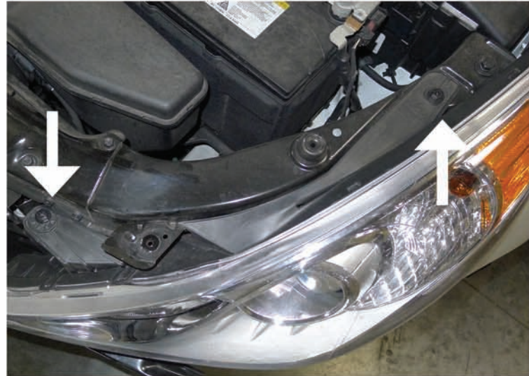
10.. 2 10mm bolts location
