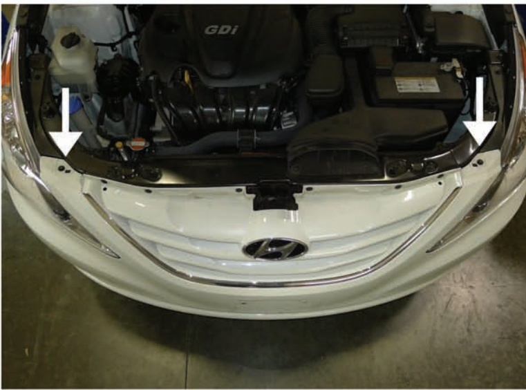
5. (2) 10mm bolts and (6) plastic clips location
