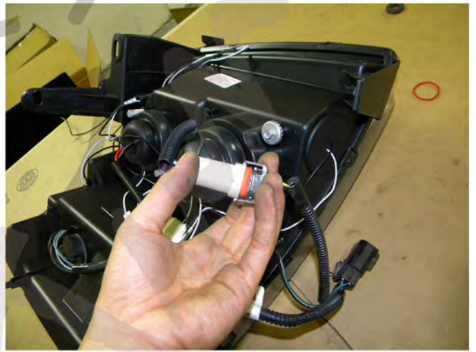
20. Connect the headlight connectors onto the harness
