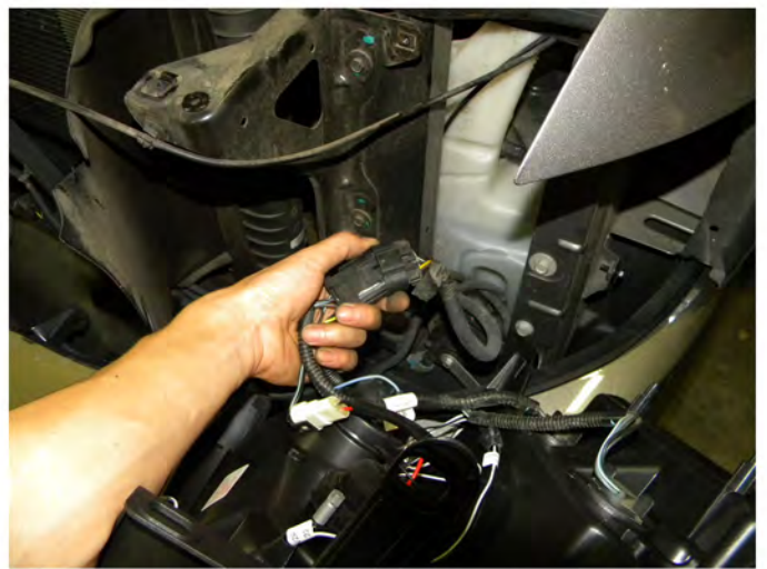
22. Connect the headlight harness connector
