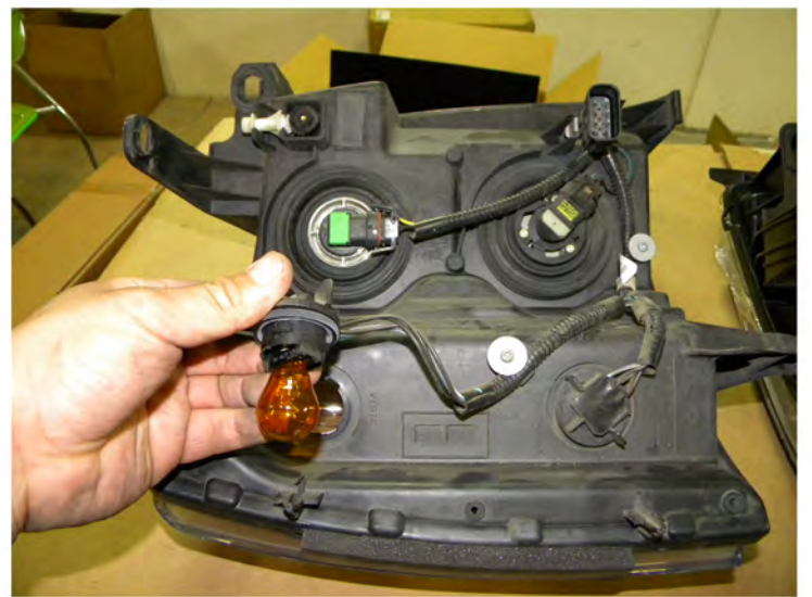
16. Remove headlight harness Please see the Halo and L.E.D installation instruction If your headlights don't have HALO or L.E.D. You can skip it
