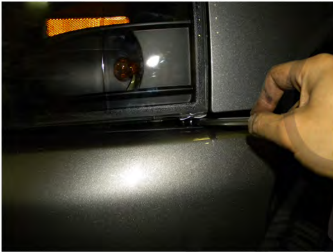
25. Tighten the 10mm bolt
