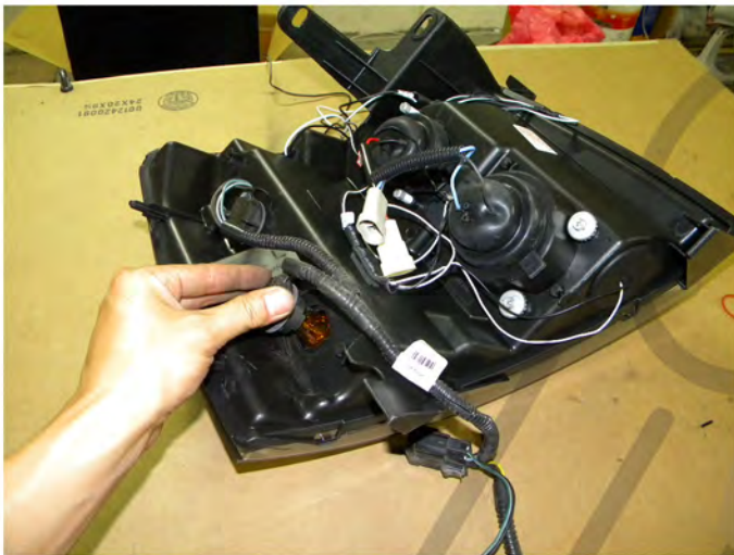
19. Place headlight sockets in the projector headlight
