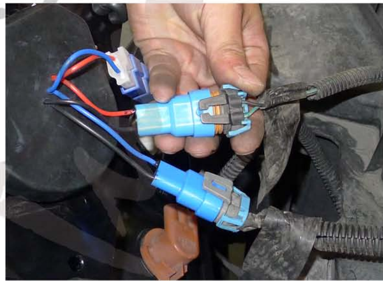
20. Connect the headlight harness to the new headlight Please see the " Halo and L. E. D. headlights installation instructions" If your headlights don't have Halo and L. E. D. You can skip the installation instruction.
