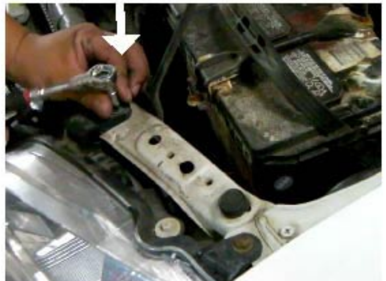
16. Install the other bolt to fasten the headlight
