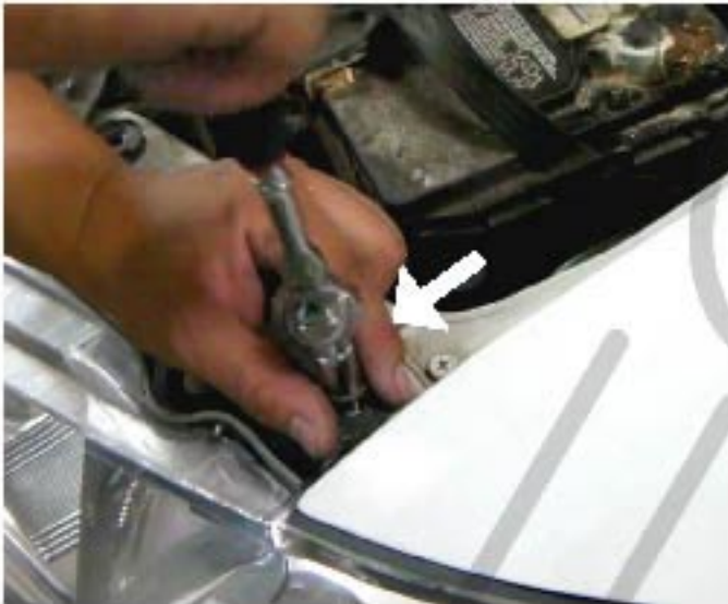
7. Remove one more bolt on the top of the headlight
