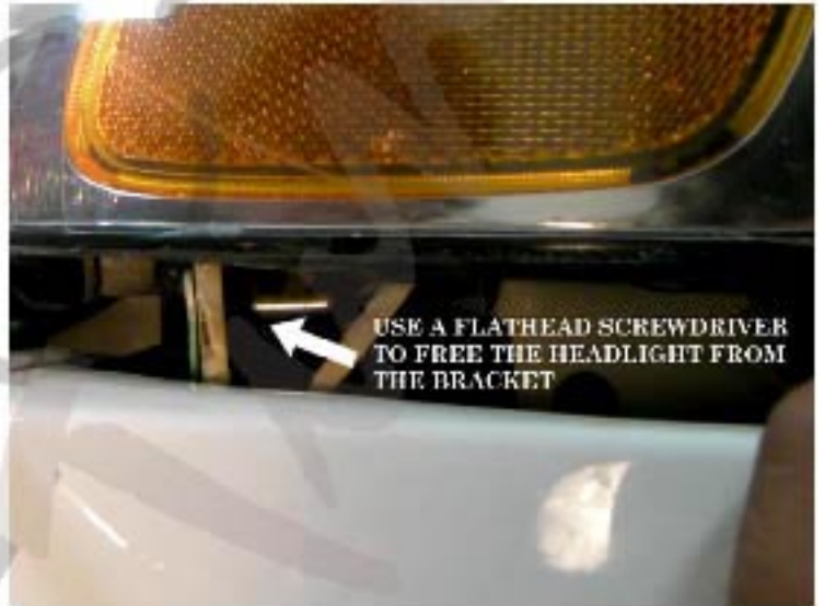
8. Use a flathead screwdriver to loosen the headlight
