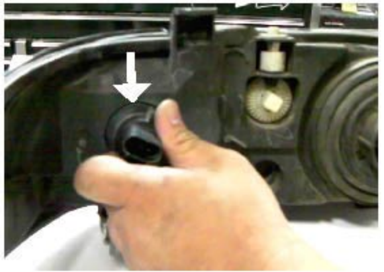
10. Remove the signal socket from the OEM headlight
