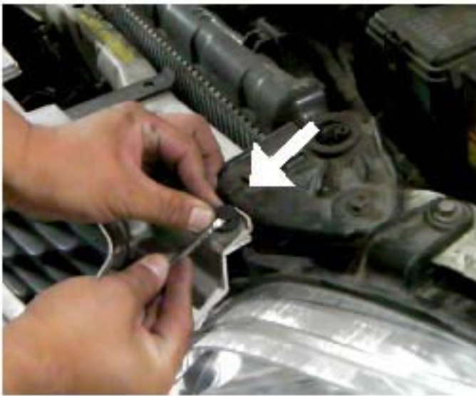
17. Install one clip for the front bumper
