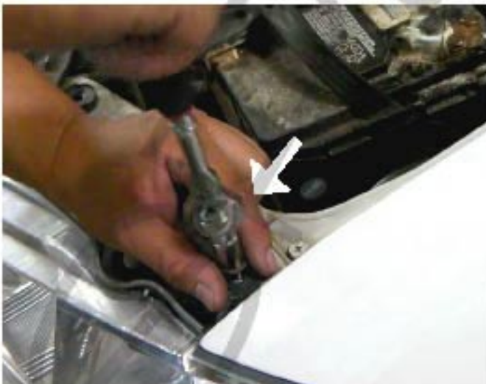
15. install one bolt at the top of the headlight
