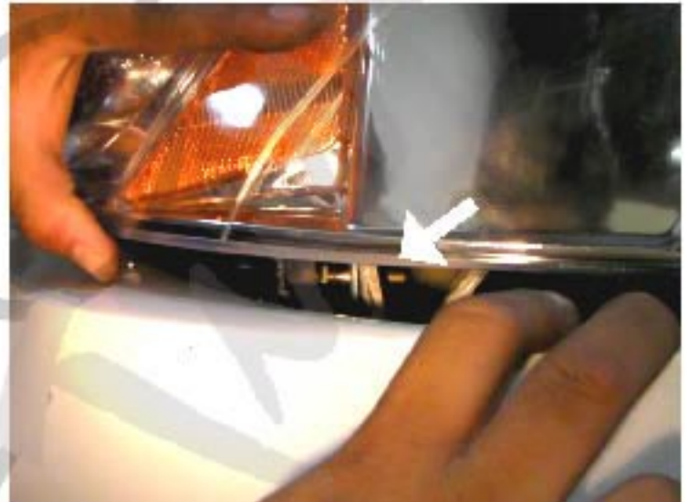
14. Hook the pin to fasten the headlight
