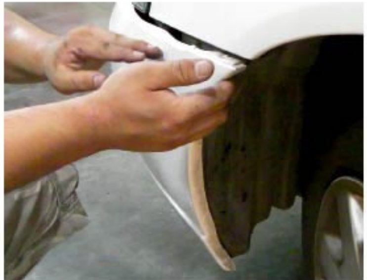
4. Pull out the side of the bumper slightly
