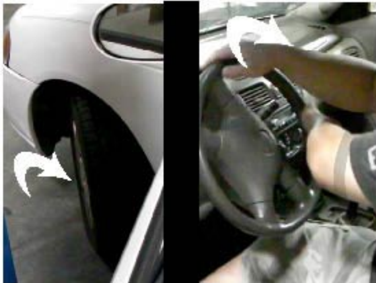
1. Space steer front wheels to the right
