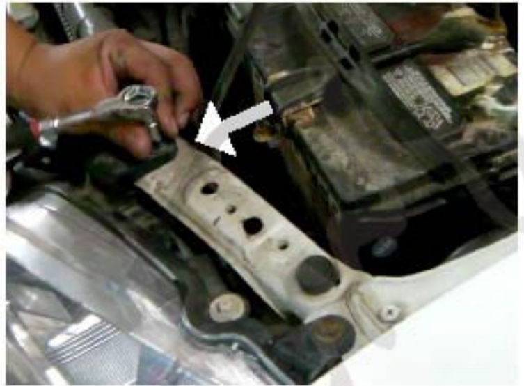
6. Remove one bolt from the top of the headlight
